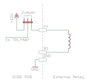
Figure 14. Normal Relay Connection
