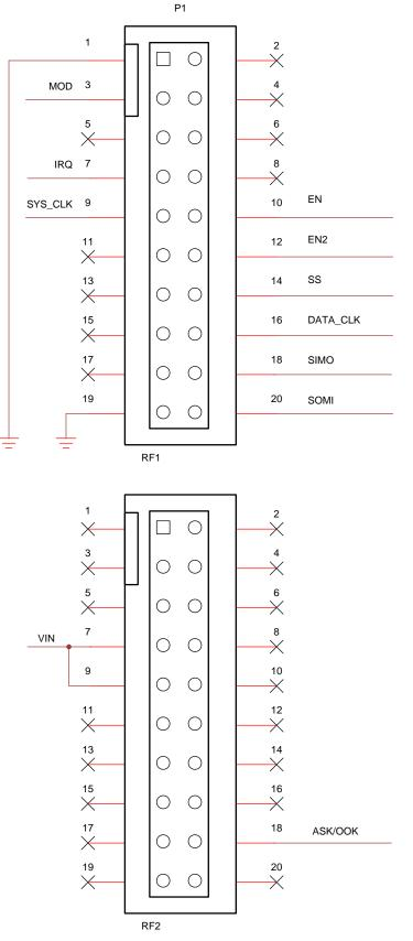
Figure 17. Connections on TRF7970ATB RF1 and RF2 Connectors
