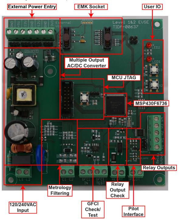
Figure 12. Top View of EVSE PCB
