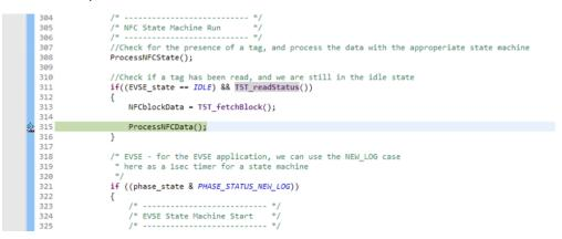
Figure 22. Break Point When Tag Data is Available
