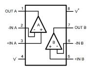
Figure 7. LM7322 Package Layout
