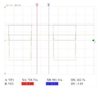
Figure 10. Pilot Signal TINA Simulation
