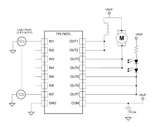
Figure 8. TPL7407 Sample Application Schematic
