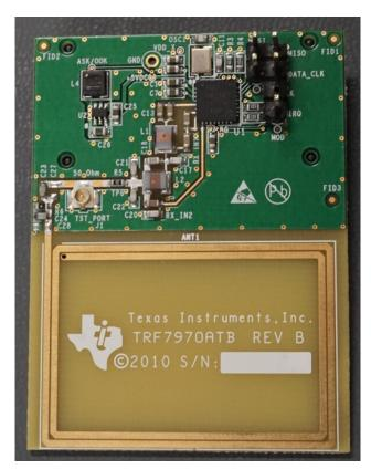
Figure 13. Front View of the TRF7970ATB
