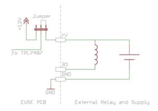
Figure 15. Relay with External Supply
