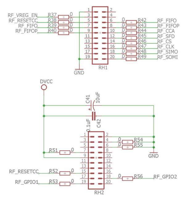
Figure 16. Connections on TIDC-EVSE-NFC RH1 and RH2 Connectors
