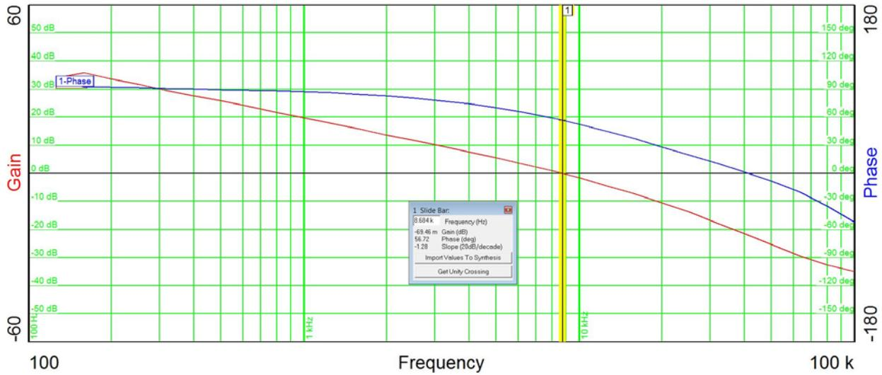
The frequency response below shows the 28V output with a full load of 2.5A.
