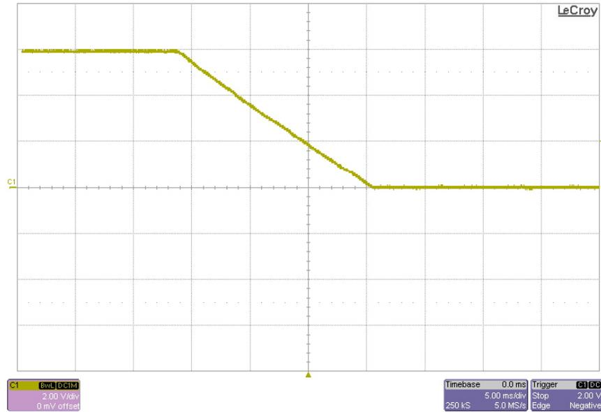
The photo below shows the turn off waveform of the 28V output, with a 100mA load, and an input voltage of 48V.
