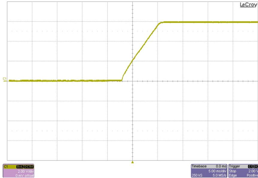
The photo below shows the startup waveform of the 28V output, with no load, and an input voltage of 48V.
