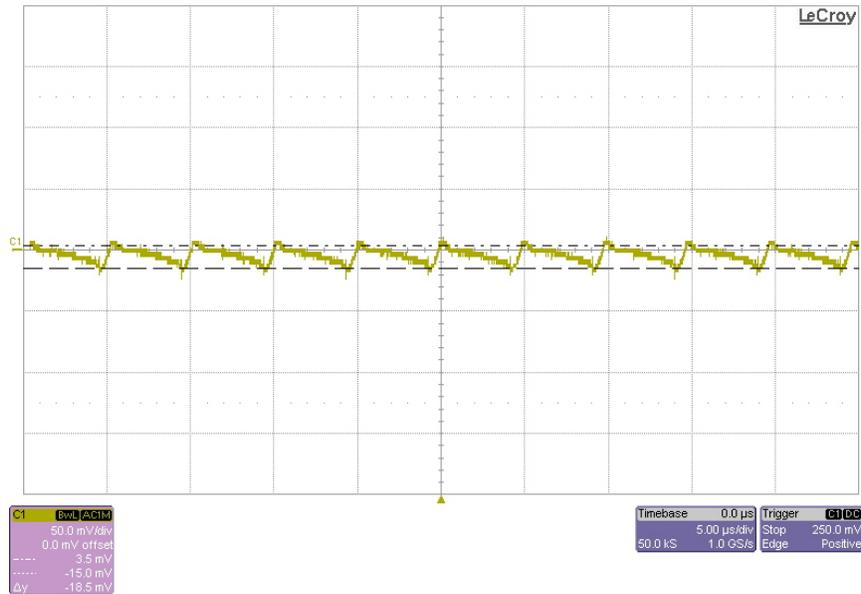
The picture below shows the output voltage ripple of the converter for the 28V output, with no load. The input voltage is 48V.
