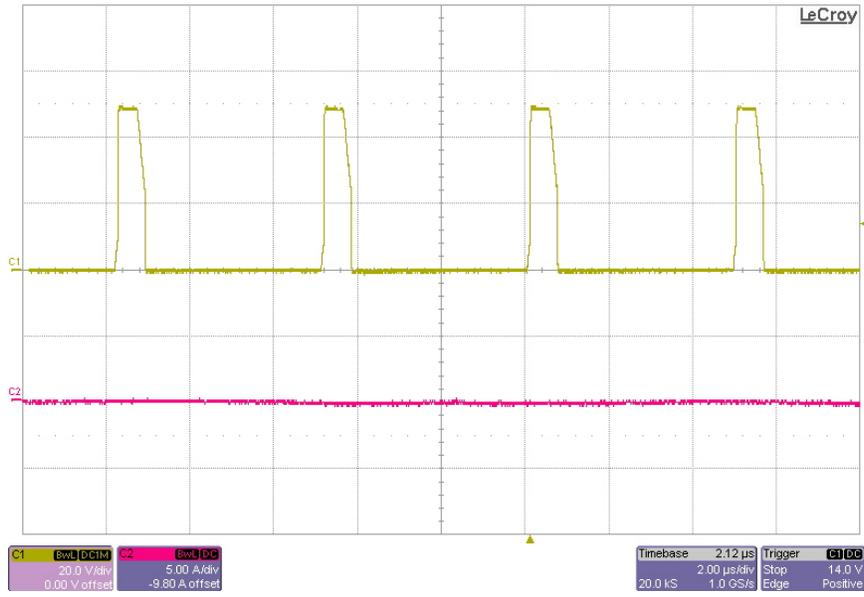
The picture below shows the switching waveform of the converter for the 28V output, with no load. The input voltage is 48V.
