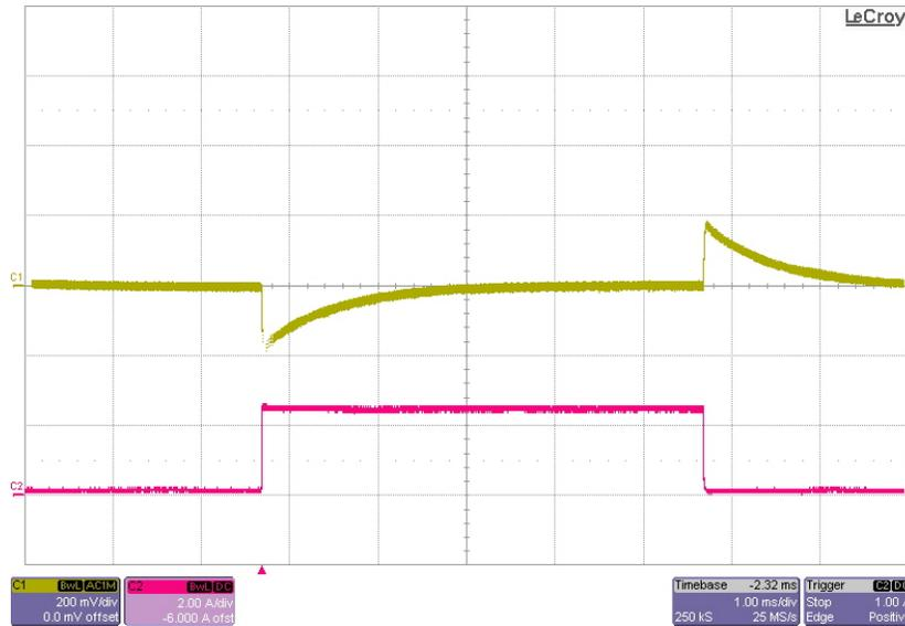
The transient response of the converter is shown in the figures below, for the 28V output, with a full load of 2.5A. The input voltage is 48V. The load is stepped from 100mA to 2.5A.
