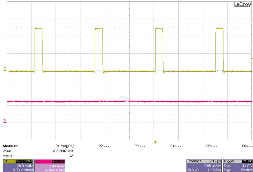
The picture below shows the switching waveform of the converter for the 28V output, with a full load of 2.5A. The input voltage is 48V and the frequency is shown to be 203 kHz.
