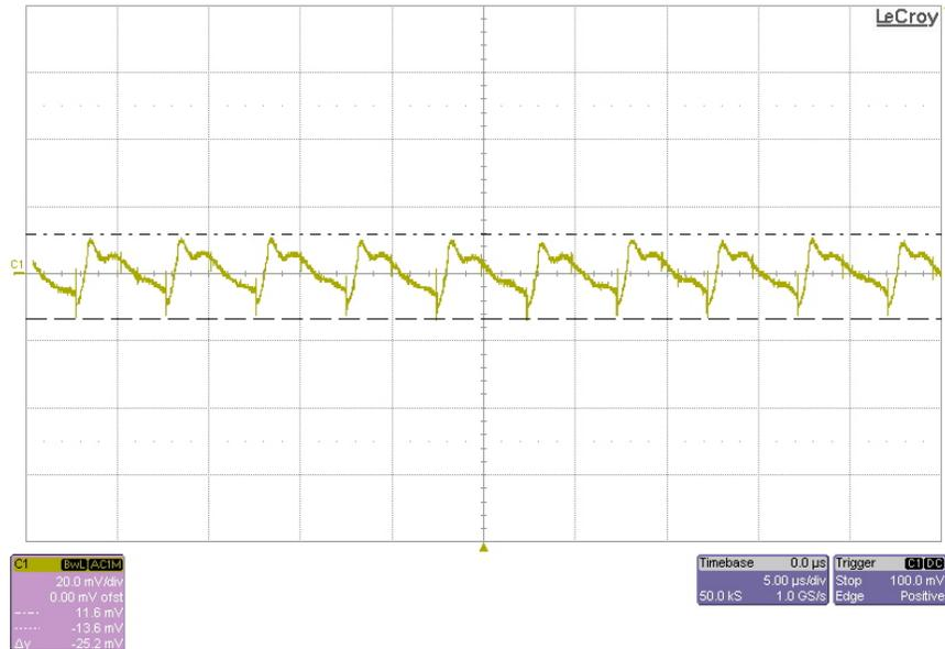
The picture below shows the output voltage ripple of the converter for the 28V output, with a full load of 2.5A. The input voltage is 48V.
