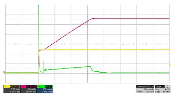
The photo below shows the output voltage startup waveform after the application of 12V in with the 28V output loaded to 0.10A. The input current is shown in green. (5V/DIV, 500mA/DIV, 50mS/DIV)
