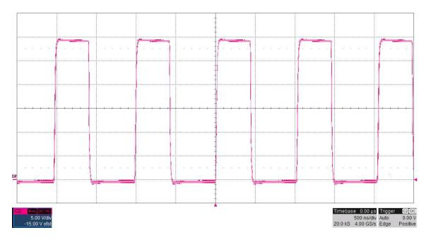
The photo below shows the switch node voltage (SW pin). The input voltage is 12V and the 28V output is loaded to 0.025A. The converter is operating in discontinuous conduction mode. (5V/DIV, 500nS/DIV)
