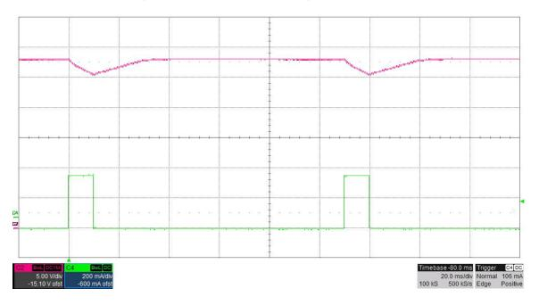
The photo below shows the output voltage when the load current is stepped between 0A and 0.5A. Vin = 12V. (5V/DIV, 200mA/DIV, 20mS/DIV)
