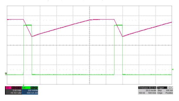
The photo below shows the output voltage when the load current is stepped between 0A and 1.25A. Vin = 12V. (5V/DIV, 200mA/DIV, 20mS/DIV)
