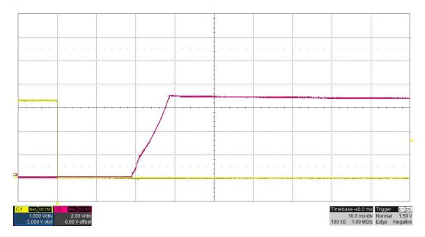
The photo below shows the 6.5V output voltage startup waveform (RED) after the /ENABLE signal (Yellow) is pulled low. Vin is 12V and the output is loaded to 2.5A. (/ENABLE is 1V/DIV, Vout is 2V/DIV, 10mS/DIV)
