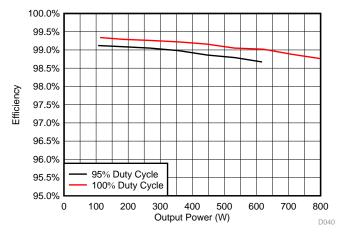
Figure 40. Inverter Efficiency versus Output Power With Heat Sink
