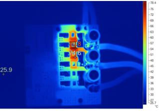
Figure 53. 120-A Peak Current in Motor Winding During Motor Stall
