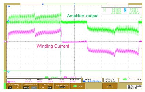
Figure 42. Current Sense Amplifier Output With Winding Current
