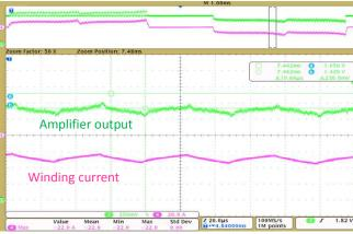
Figure 43. Current Sense Amplifier Output at Positive Winding Current
