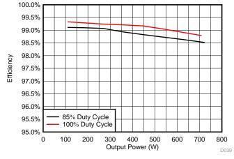
Figure 39. Inverter Efficiency versus Output Power Without Heat Sink
