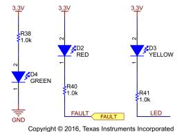
Figure 13. LED Indications Schematic
