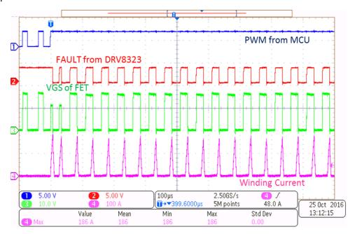
Figure 49. Cycle-by-cycle Overcurrent Protection With Inverter Output Shorted
