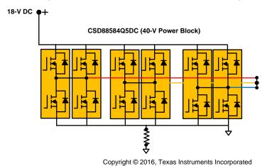
Figure 48. Test Setup to Simulate Inverter Short Circuit
