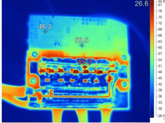
Figure 35. Load Test Results at 18-V DC Input, 42-A<sub>RMS</sub> Winding Current, 100% Duty Cycle
