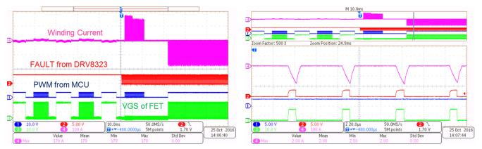
Figure 46. Cycle-by-Cycle Overcurrent Protection With Motor Stall
