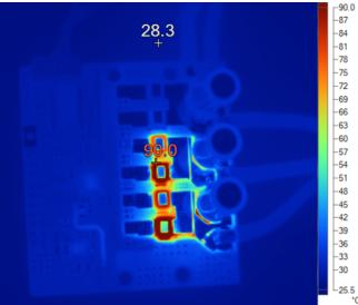
Figure 55. 160-A Peak Current in Motor Winding During Motor Stall
