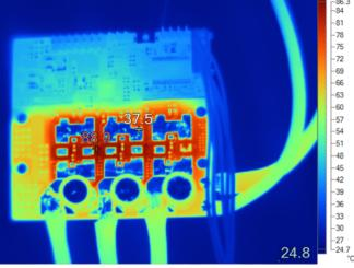
Figure 33. Load Test Results at 18-V DC Input, 31.8-A<sub>RMS</sub> Winding Current, 90% Duty Cycle
