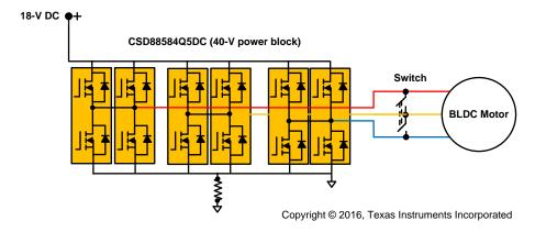
Figure 45. Test Setup to Simulate Stall Current When Motor is Running
