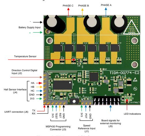
Figure 15. TIDA-00774 PCB Connectors
