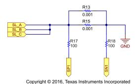
Figure 4. External Shunt for Current Sensing
