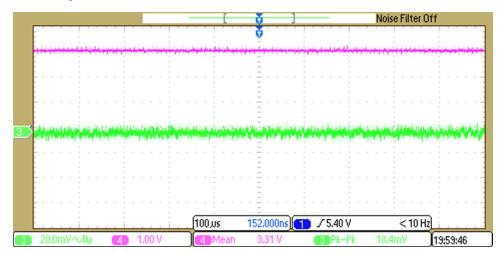
Figure 18. Output Voltage of 3.3 V From Step-Down Converter and 3.3-V Voltage Ripple
