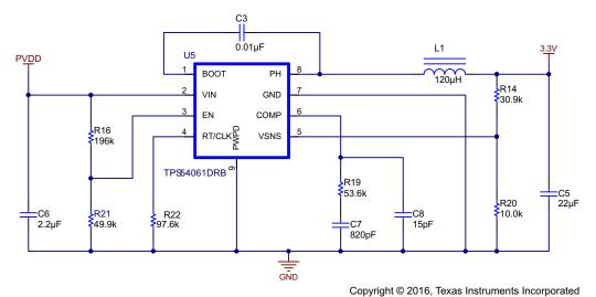
Figure 7. 18-V to 3.3-V DC Converter
