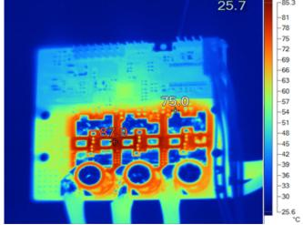
Figure 31. Load Test Results at 18-V DC Input, 33-A<sub>RMS</sub> Winding Current, 100% Duty Cycle
