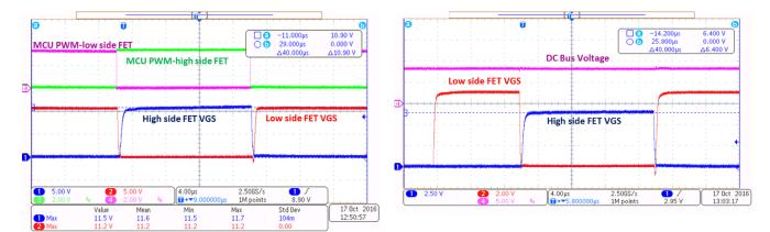
Figure 19. Low-Side and High-Side Gate Drive Voltage at 18-V DC
