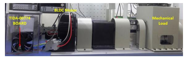
Figure 17. Board and Motor Test Setup
