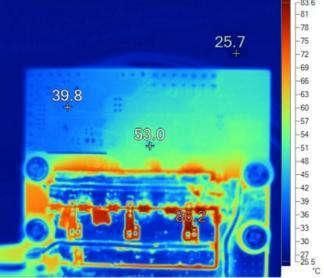
Figure 37. Load Test Results at 18-V DC Input, 48.2-A<sub>RMS</sub> Winding Current, 95% Duty Cycle
