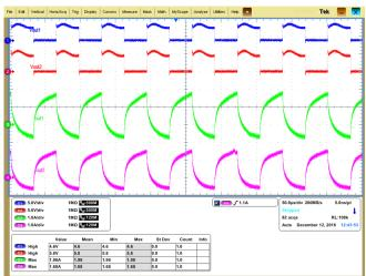
Figure 16. 5-V DRV8850 Board—50% Duty Cycle
