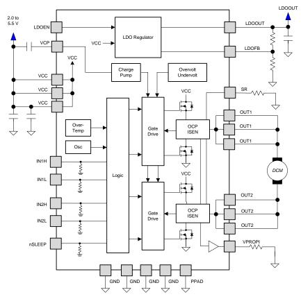
Figure 2. DRV8850 Functional Block Diagram
