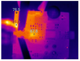
Figure 19. 5-V Discrete Board at 95% Duty Cycle
