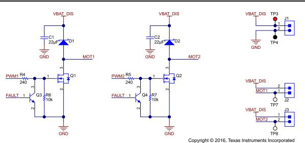
Figure 5. Discrete Implementation Motor Connection
