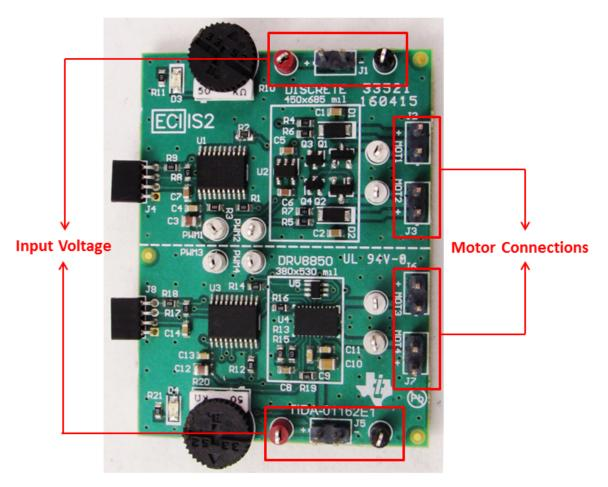
Figure 7. Input and Output Connections
