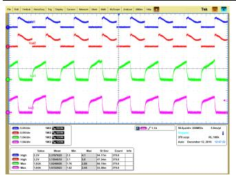
Figure 15. 5-V Discrete Board—50% Duty Cycle
