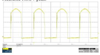
Drain to source, Q13, 48V input, 3.0A load 20V/div, 2usec/div, 750MHz bandwidth
