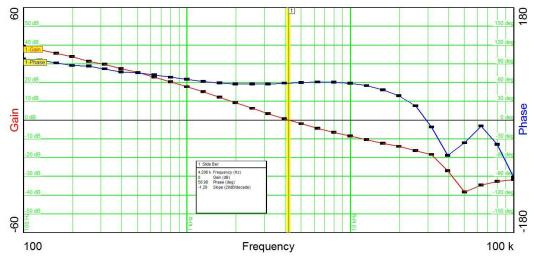
Bandwidth= 4.2 kHz Phase Margin=59 degrees Gain Margin=18dB
