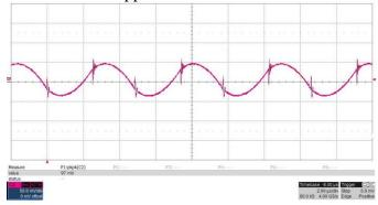
Input Ripple (C68), 10mV/div, 2usec/div
