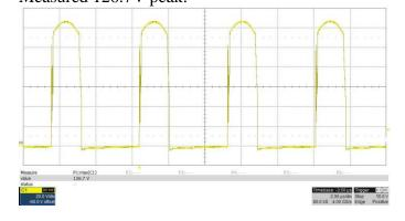
Drain to source, Q13, 38V input, 3.0A load 20V/div, 2usec/div, 750MHz bandwidth
