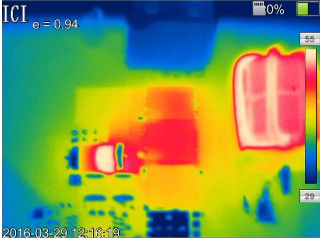
Vin =24V; Iout=12A (max temp 55C)
