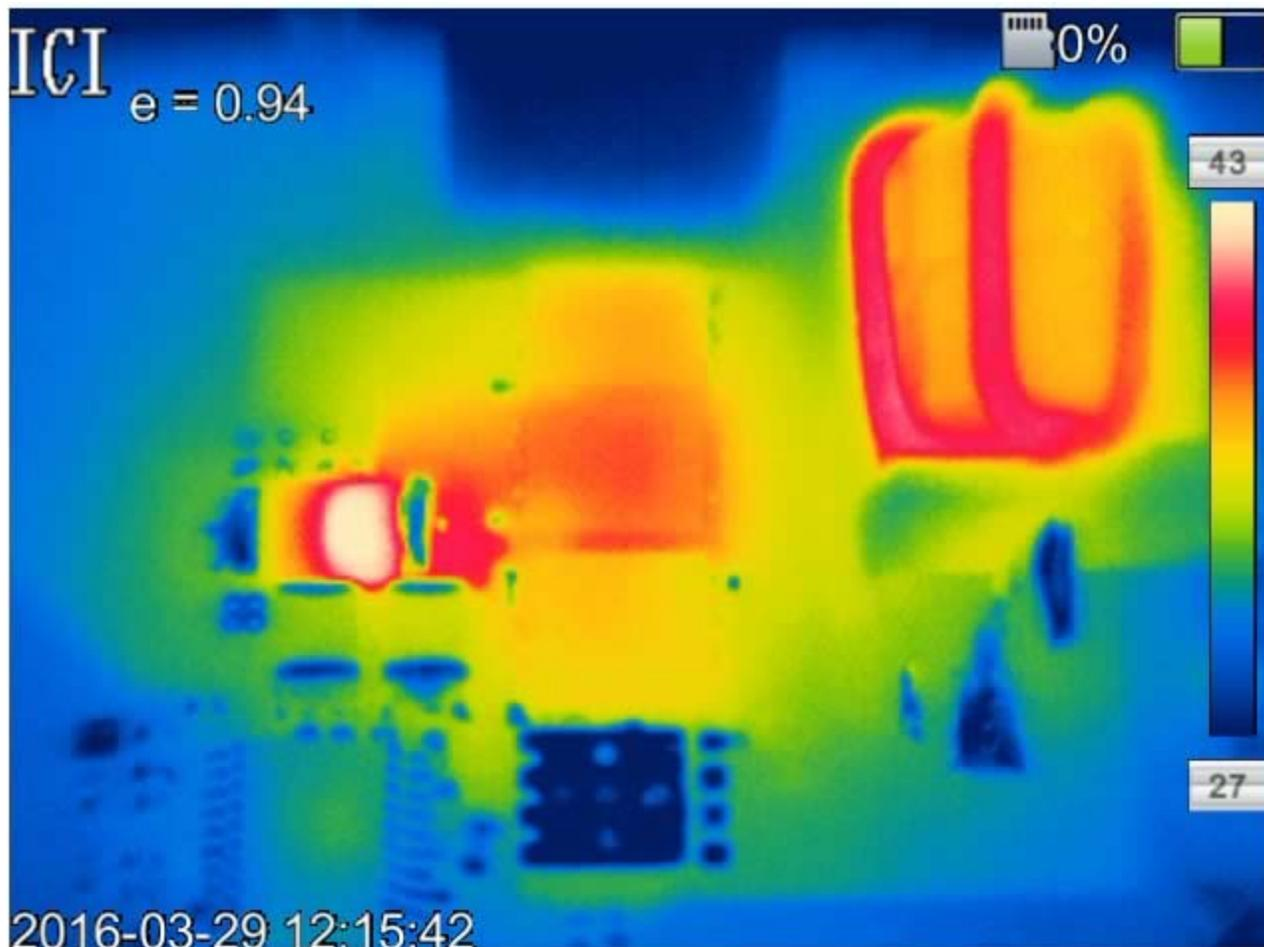
Vin =12V; Iout=12A (max temp 43C)
