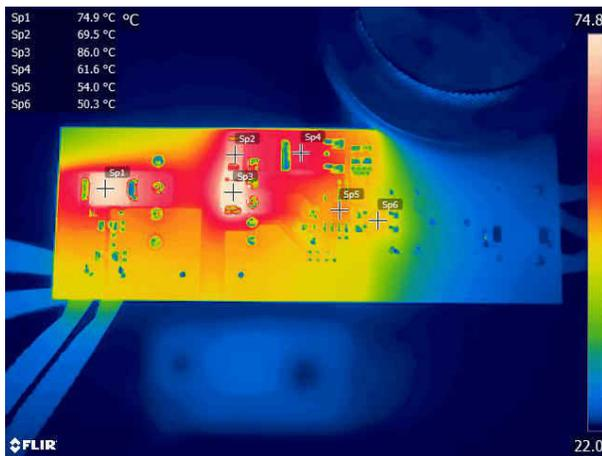
Figure 2-4. Thermal Image, 230-VAC, 50-Hz Bottom
