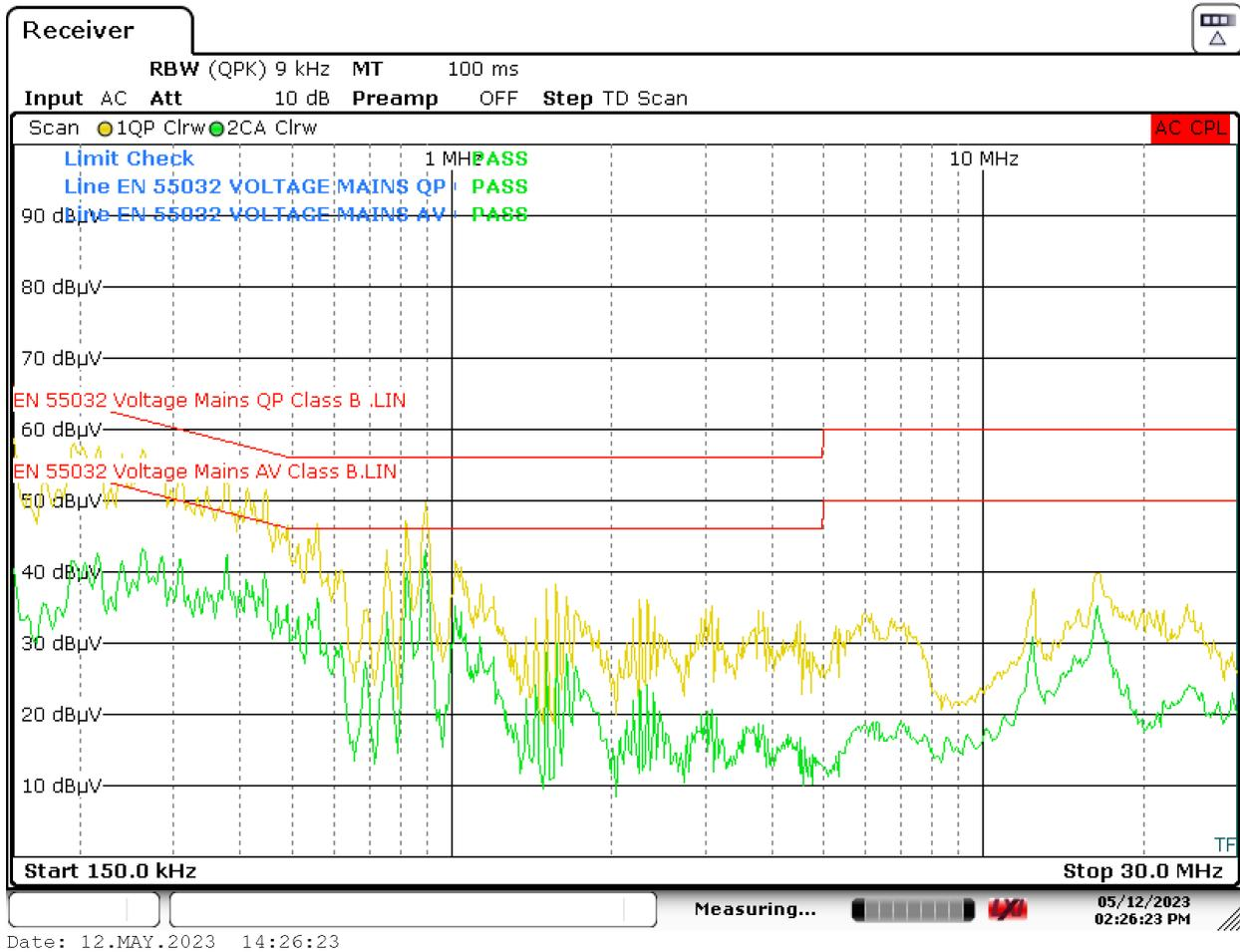
Figure 3-10. Measurement With 230-VAC, 50-Hz Input, Line Neutral Flipped
