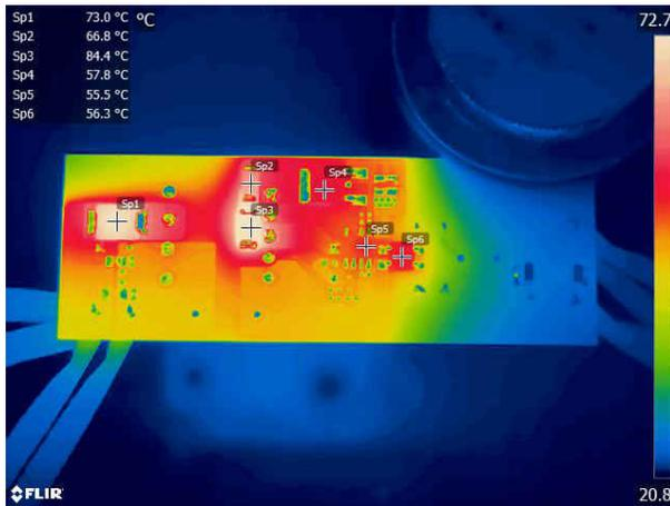
Figure 2-2. Thermal Image, 120-VAC, 60-Hz Bottom
