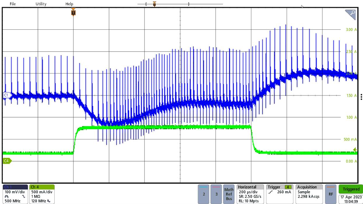
Figure 3-3. Transient Response to a 20% – 80% Load Step
