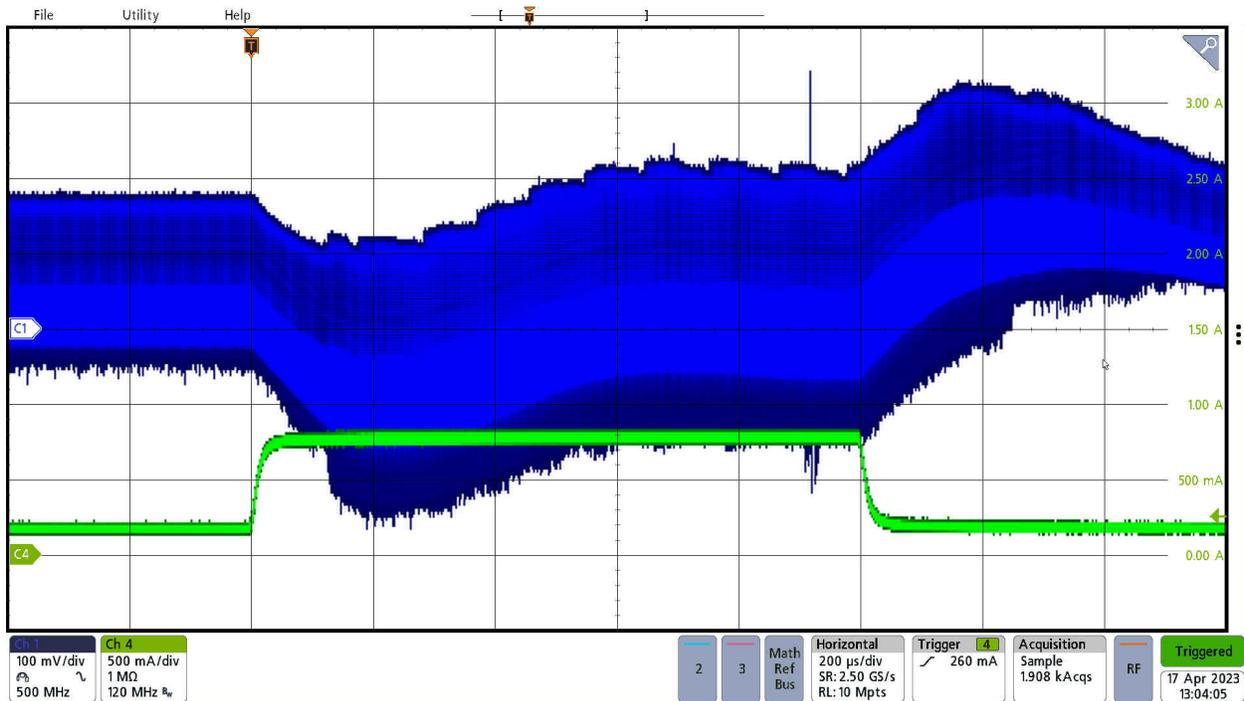
Figure 3-4. Transient Response to a 20% – 80% Load Step With Analog Persist
