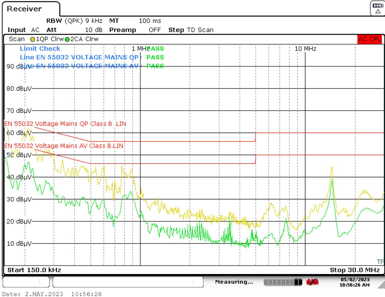
Figure 3-7. Measurement With 120-VAC, 60-Hz Input
