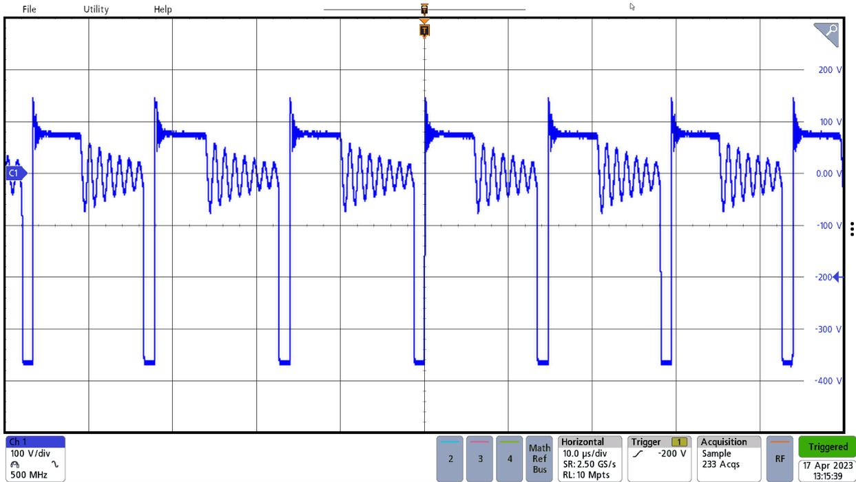
**Figure 3-5. Drain of Primary FET Q1 – 265-VAC, 50-Hz Input, 12-V, 1-A Output**
