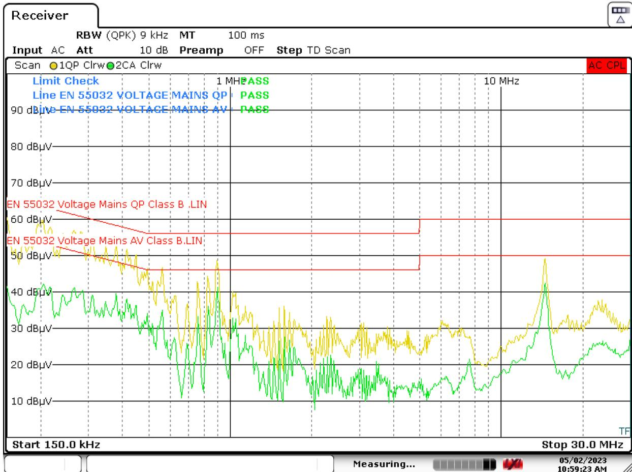
Figure 3-9. Measurement With 230-VAC, 50-Hz Input
