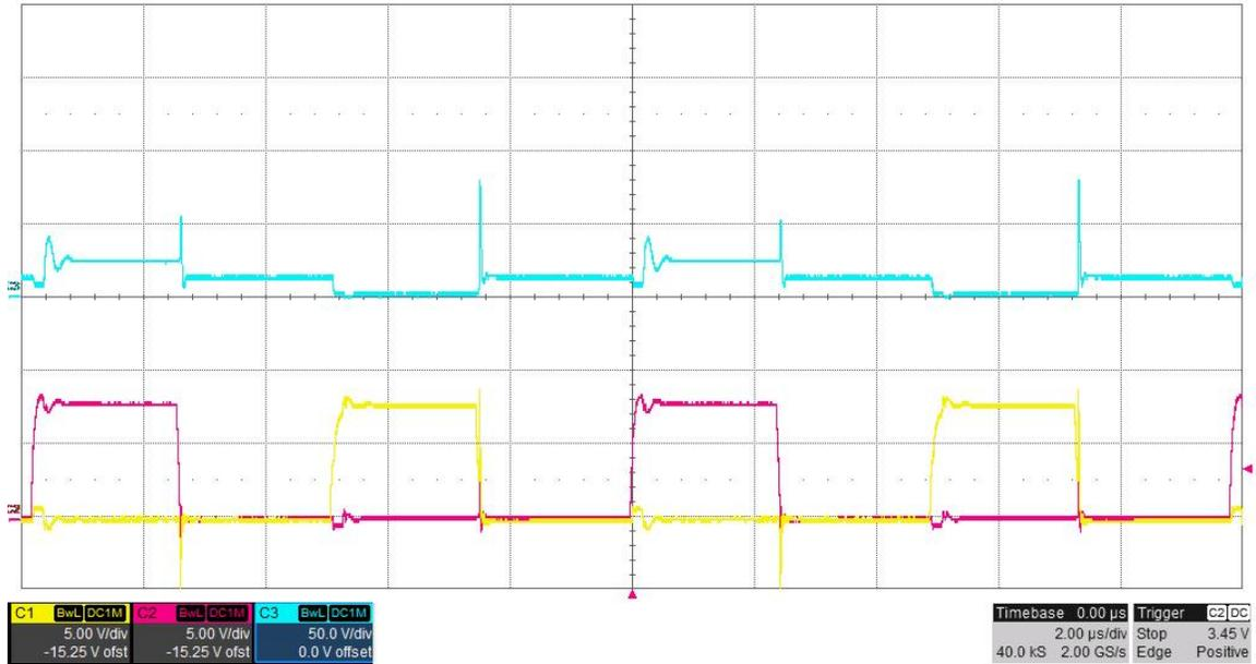
The photo below shows the FET switching voltage and the OUTA and OUTB FET gate driver voltages for an input voltage of 6V. The outputs were loaded differentially with 10 ohms (1A). (5V/DIV, 2uS/DIV)
