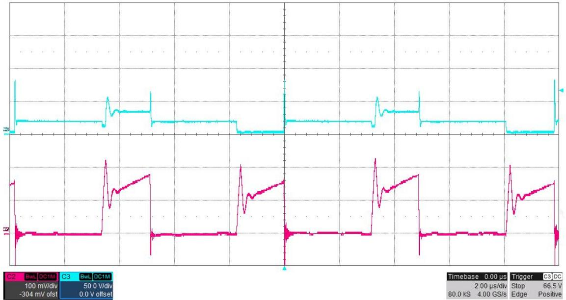
The photo below shows the FET switching voltage and the voltage across R7 for an input voltage of 12V. The outputs were loaded differentially with 10 ohms (5A). (50V/DIV, 100mV/DIV, 2uS/DIV)
