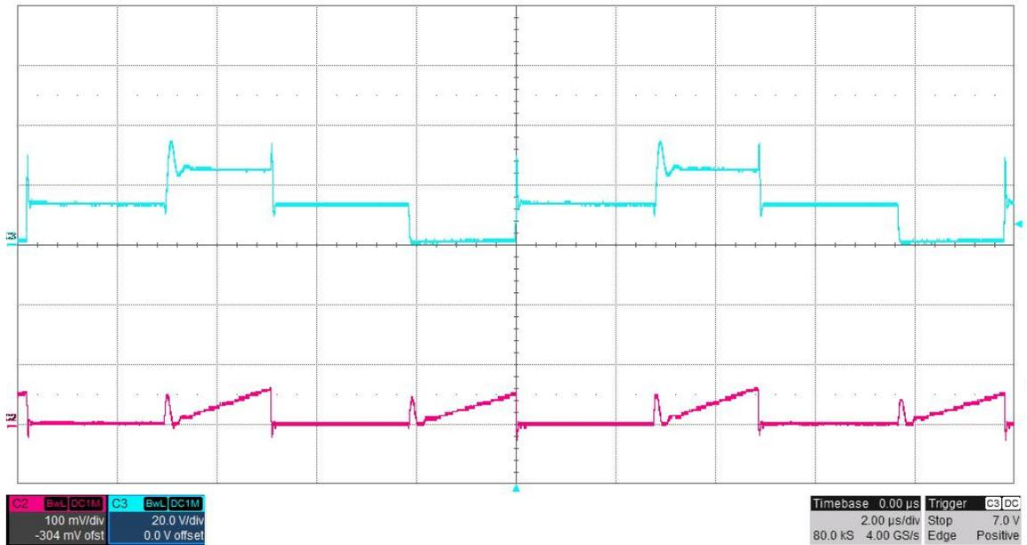
The photo below shows the FET switching voltage and the voltage across R7 for an input voltage of 6V. The outputs were loaded differentially with 10 ohms (5A). (20V/DIV, 100mV/DIV, 2uS/DIV)
