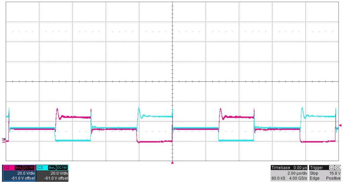
The photo below shows the FET switching voltages for an input voltage of 6V. The outputs were loaded differentially with 10 ohms (5A). (20V/DIV, 2uS/DIV)
