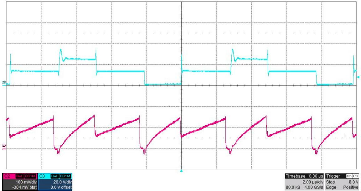
The photo below shows the FET switching voltage and the controller RAMP pin voltage for an input voltage of 6V. The outputs were loaded differentially with 10 ohms (5A). (20V/DIV, 100mV/DIV, 2uS/DIV)
