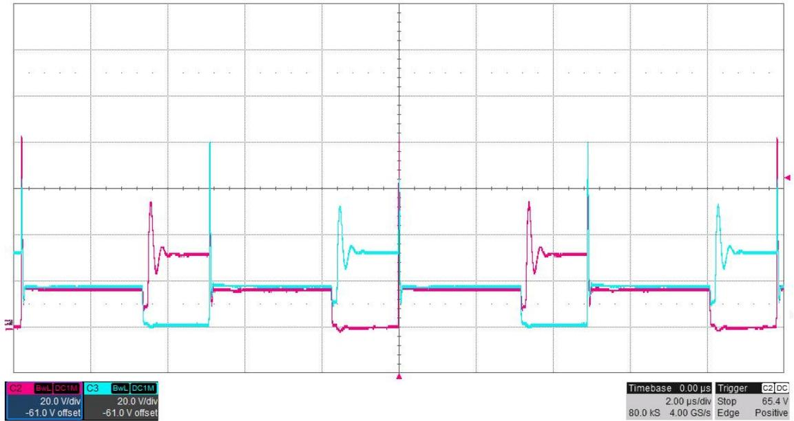
The photo below shows the FET switching voltages for an input voltage of 12V. The outputs were loaded differentially with 10 ohms (5A). (20V/DIV, 2uS/DIV)
