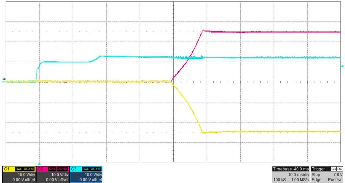
The photo below shows the output voltage startup waveform after the application of 12V in. The +25V/-25V outputs were loaded differentially with 10 ohms (5A). (10V/DIV, 10mS/DIV)
