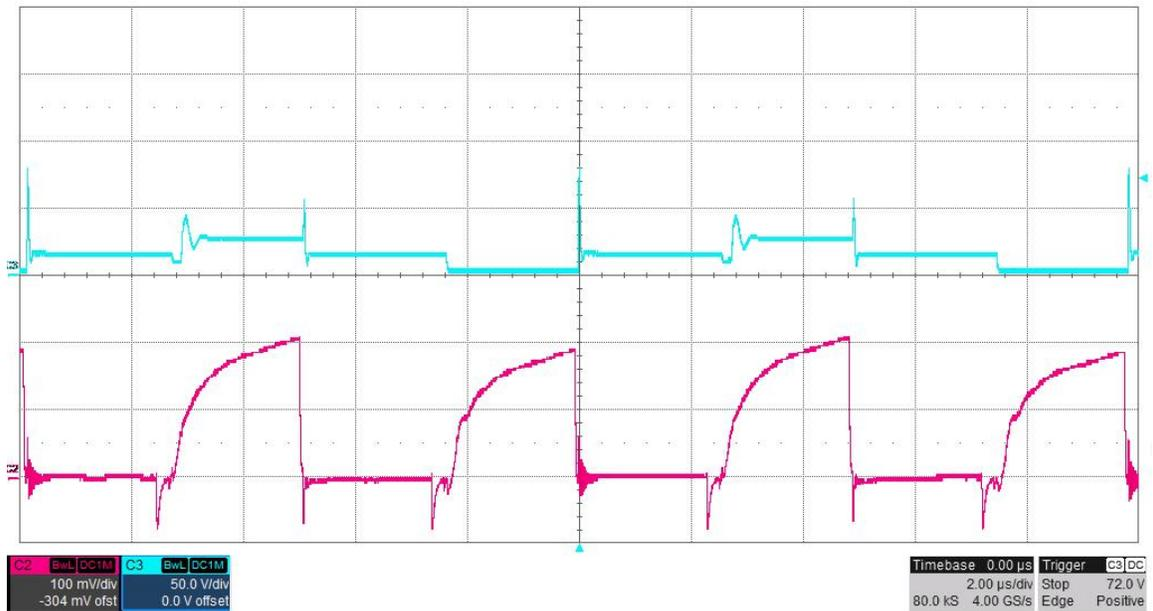
The photo below shows the FET switching voltage and the controller CS pin voltage for an input voltage of 12V. The outputs were loaded differentially with 50 ohms (1A). (20V/DIV, 100mV/DIV, 2uS/DIV)
