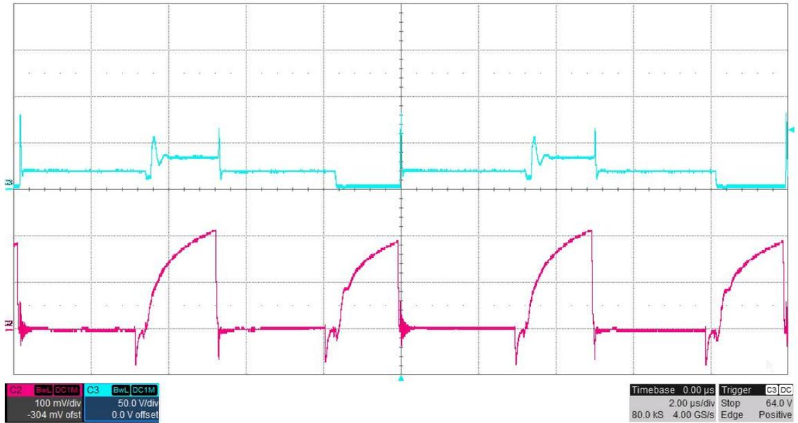
The photo below shows the FET switching voltage and the controller CS pin voltage for an input voltage of 12V. The outputs were loaded differentially with 10 ohms (5A). (50V/DIV, 100mV/DIV, 2uS/DIV)
