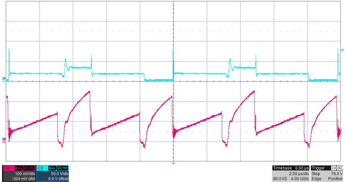
The photo below shows the FET switching voltage and the controller RAMP pin voltage for an input voltage of 12V. The outputs were loaded differentially with 10 ohms (5A). (50V/DIV, 100mV/DIV, 2uS/DIV)
