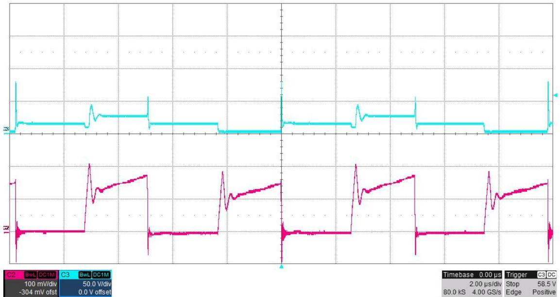
The photo below shows the FET switching voltage and the voltage across R7 for an input voltage of 12V. The outputs were loaded differentially with 50 ohms (1A). (20V/DIV, 100mV/DIV, 2uS/DIV)
