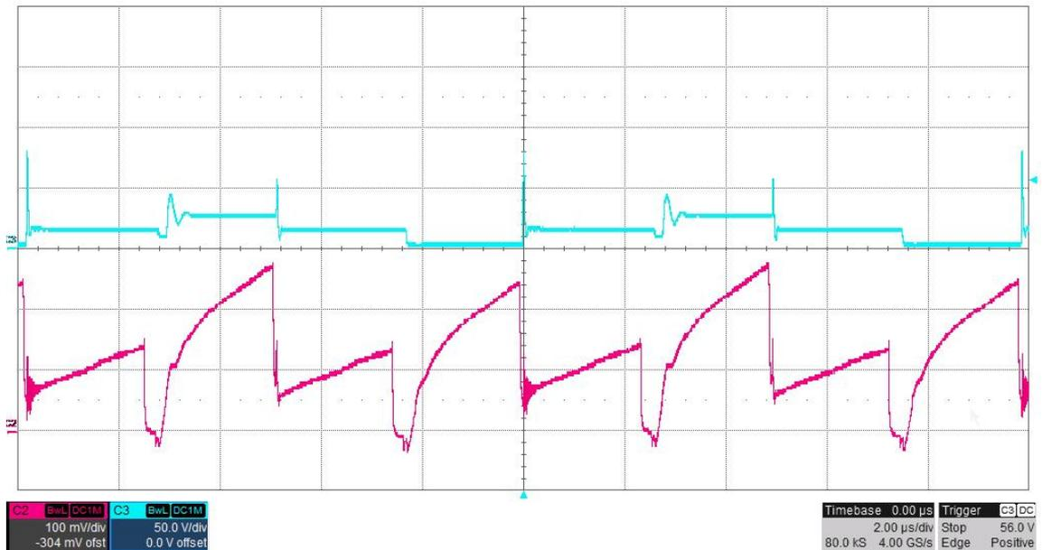
The photo below shows the FET switching voltage and the controller RAMP pin voltage for an input voltage of 12V. The outputs were loaded differentially with 50 ohms (1A). (20V/DIV, 100mV/DIV, 2uS/DIV)
