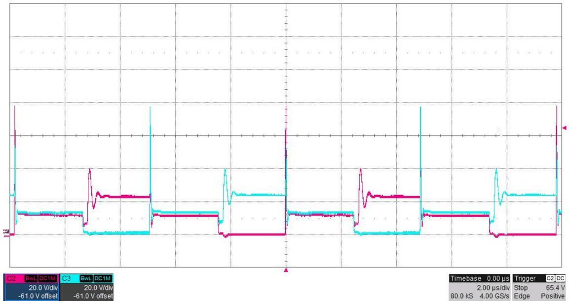
The photo below shows the FET switching voltages for an input voltage of 12V. The outputs were loaded differentially with 50 ohms (1A). (20V/DIV, 2uS/DIV)
