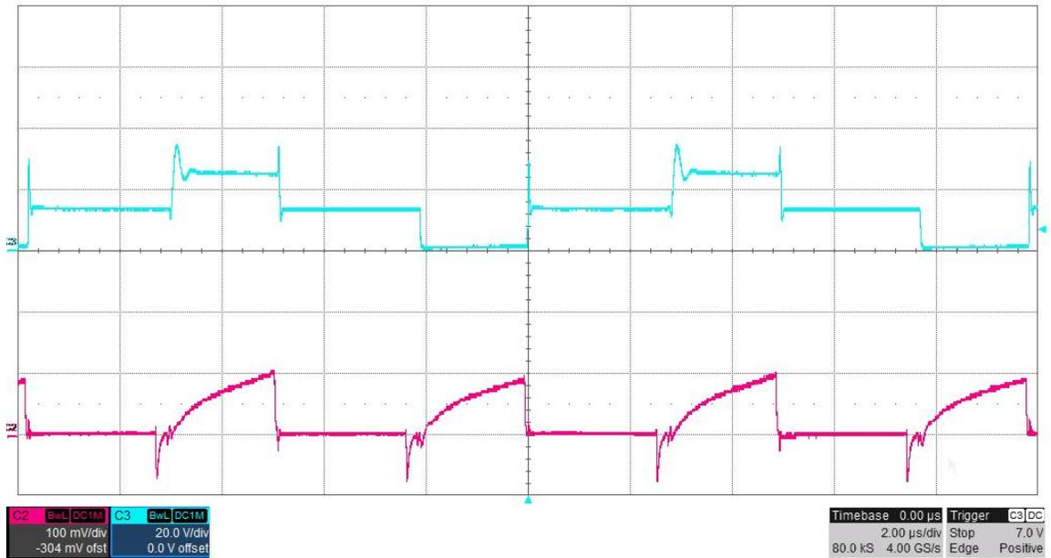
The photo below shows the FET switching voltage and the controller CS pin voltage for an input voltage of 6V. The outputs were loaded differentially with 10 ohms (5A). (20V/DIV, 100mV/DIV, 2uS/DIV)
