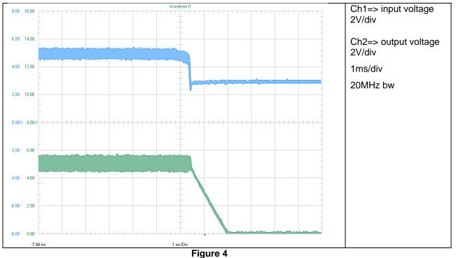
The shutdown waveform is shown in the Figure 5. The input voltage was set to 10V. The power supply was disconnected.
