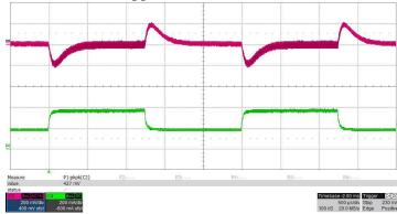
Output Load Step; 0mA to 360mA load step; Slew Rate = 250mA/usec 500mV/div, 200mA/div, 500usec/div
