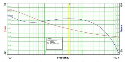
Bandwidth: 4.5 KHz Phase Margin: 70 degrees Gain Margin: 14dB
