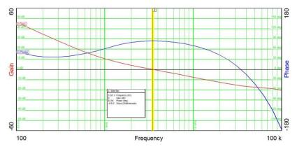
Bandwidth: 3.5 KHz Phase Margin: 83 degrees Gain Margin: 17dB
