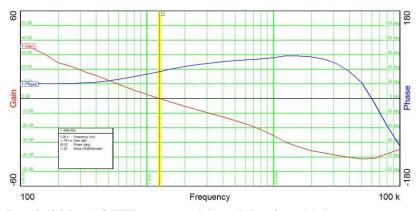
Bandwidth: 1.2 KHz Phase Margin: 55 degrees Gain Margin: 41dB
