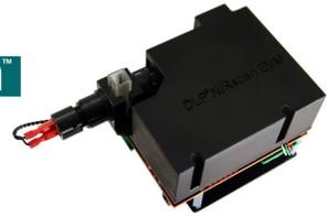
The **DLP NIRscan™ Nano** EVM offers a battery-operated portable solution for your spectroscopy system designs. The Bluetooth-enabled EVM features the DLP2010NIR DMD and is optimized for material sensing in the 900 – 1700nm wavelength range.
