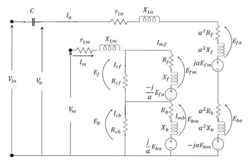
Figure 4: Equivalent circuit model for a SPIM [3]
