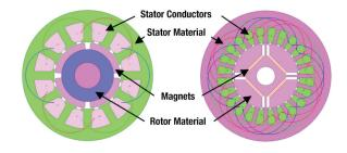
Figure 9: Example of three-phase BLDC motor cross-section: SM-PMSM (left); IPMSM (right)
