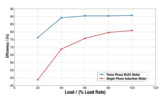
Figure 12: Efficiency comparison\*
