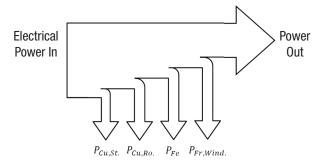
Figure 6: Losses in a single-phase induction motor [02]
