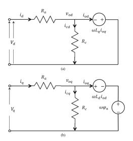
Figure 10: Rotor reference frame loss model of a BLDC motor
