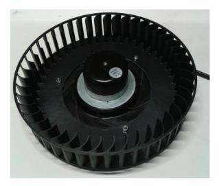
Figure 14: Three-phase BLDC motor with fan blades used in the experiment
