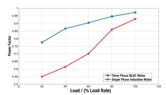
Figure 13: Power factor comparison\*
