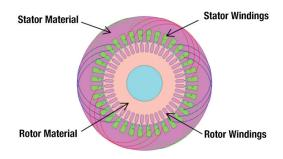
Figure 7: Example three-phase ACIM cross-section
