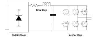
Figure 1: Drive stage for three-phase systems
