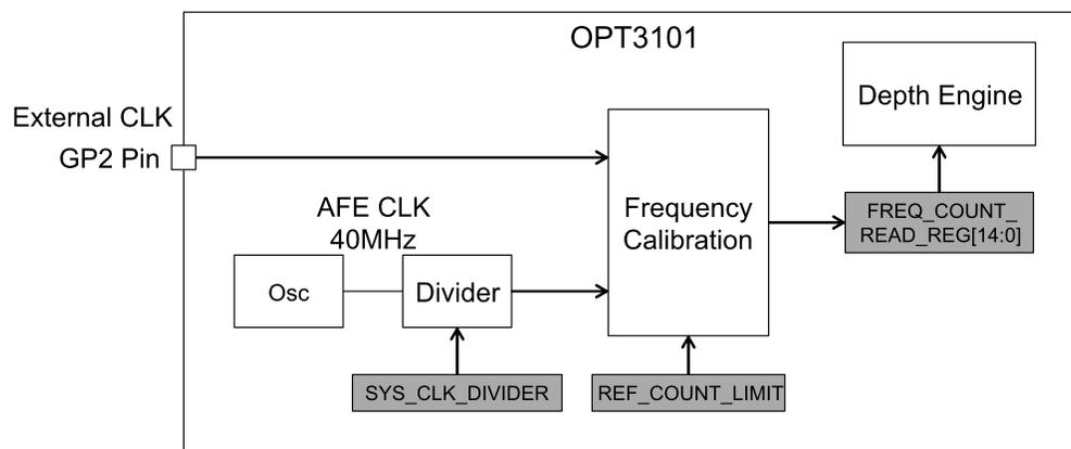
Figure 3. Frequency Calibration Block Diagram
