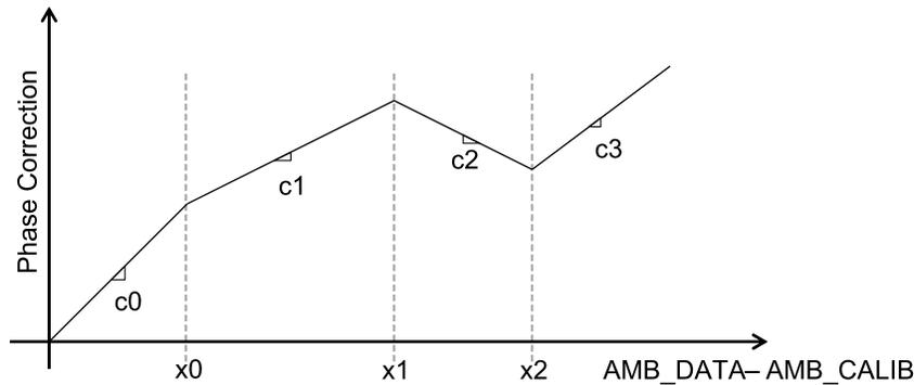
Figure 8. PWL Based Correction for Ambient Dependent Phase
