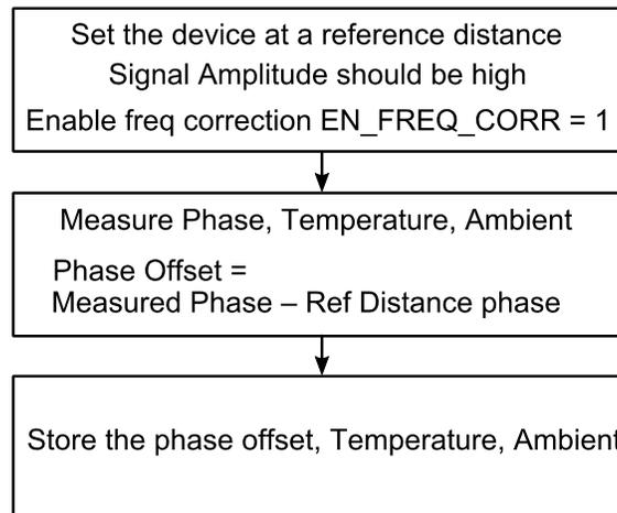
**Figure 5. Phase Offset Calibration Procedure**
