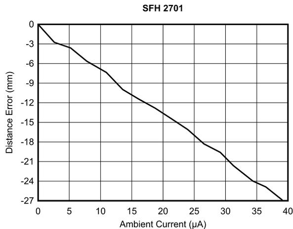
**Figure 6. Distance Error With Ambient Current: SFH2701 as Photodiode**
