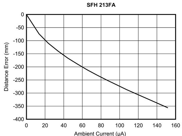
**Figure 7. Distance Error With Ambient Current: SFH213FA as Photodiode**
