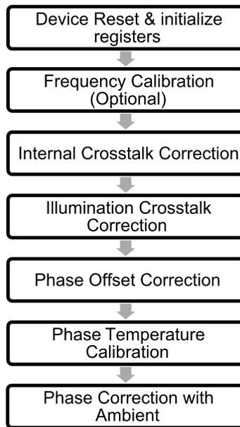
Figure 2. OPT3101 System Calibration Steps
