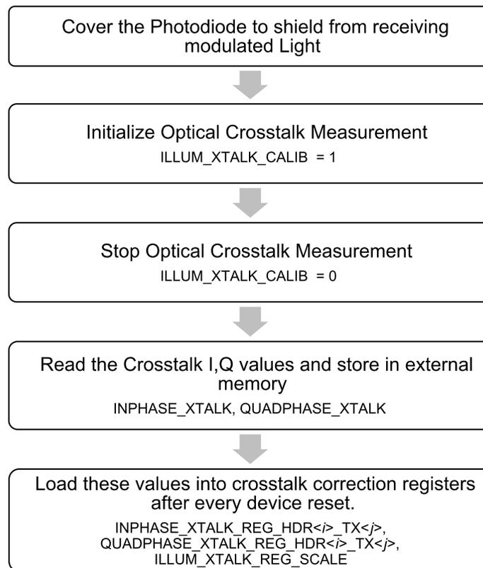
Figure 4. Illumination Crosstalk Calibration Procedure
