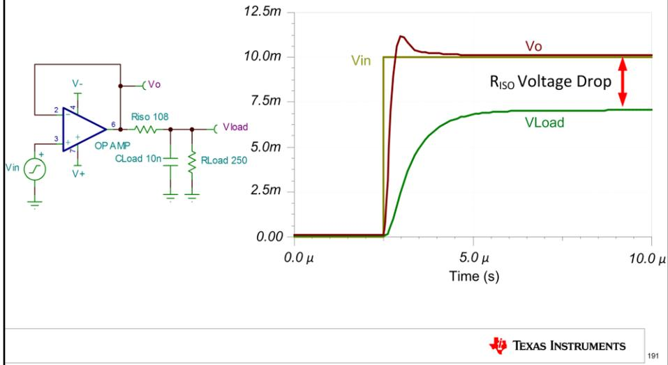
While the Riso circuit is both simple to implement and design it has a big disadvantage in precision circuits. The voltage drop from Riso is dependent on the output current or output load, and may be significant compared to the desired signal. As shown here a 10mV signal has over 3mV (30%) of error due to a 250 $\Omega$  output load.
