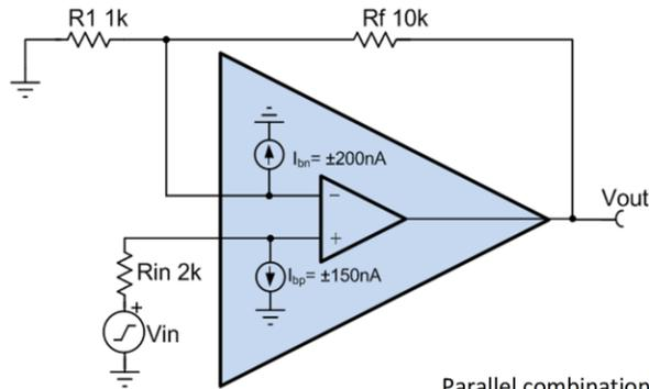
$$R_{eq} = \frac{R_f \cdot R_1}{R_f + R_1} = 0.909k\Omega$$
