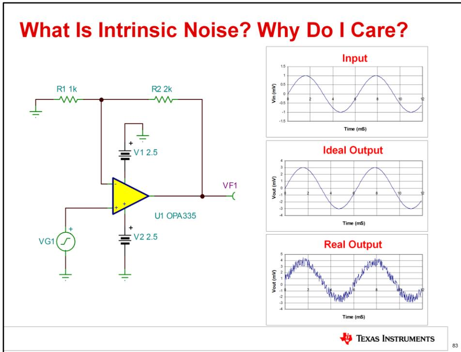
Noise can be defined as an unwanted signal that combines with a desired signal to result in an error. In audio, for example, noise can be noticed as a hiss or popping sound. In a sensor system, noise can be an error in the measured sensor output, such as pressure or temperature.
