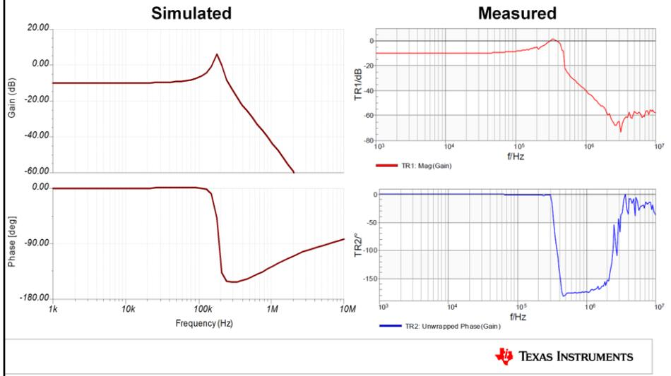
In addition to oscilloscopes, gain/phase analyzers can be used to measure the frequency response of a circuit which can also be used to identify stability issues. These results compare a circuit's simulated gain/phase response versus the measured response.
