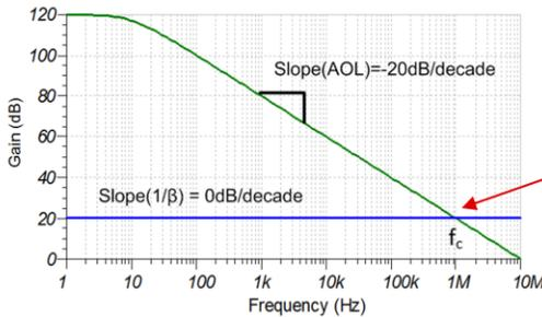
$$\text{Rate of Closure} = \left| \text{Slope}(A_{OL}) - \text{Slope}\left(\frac{1}{\beta}\right) \right|$$
