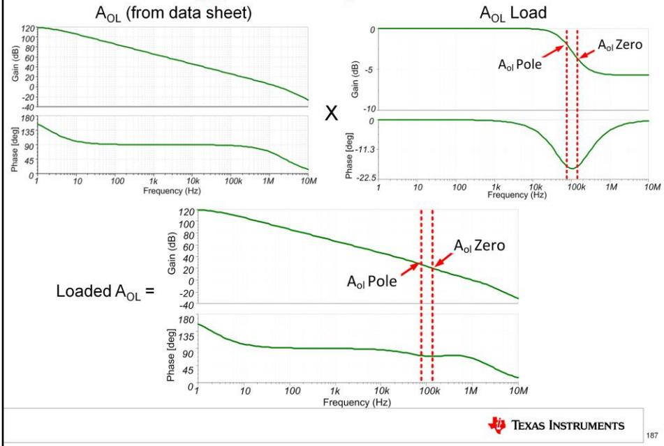
Adding the A<sub>OL</sub> and A<sub>OL</sub> load curves together as before, we can again see that the zero added by R<sub>ISO</sub> cancels the pole in the A<sub>OL</sub> curve and restores the phase margin to an acceptable level for stability.
