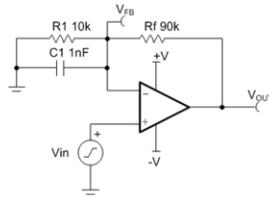
$$\frac{1}{\beta} = \frac{V_{OUT}}{V_{FB}} = 10 \left( \frac{f}{f_c} + 1 \right)$$
