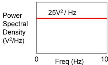
You must integrate the **Power** spectral density curve to get noise
