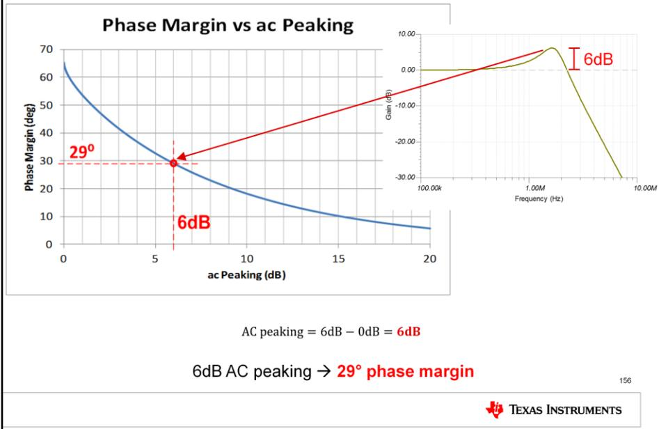
In AC Gain/Phase plots, the amount of ac peaking relative to the DC gain can be used to indirectly measure the phase margin of a circuit. In this example, the AC transfer function is peaking at 6dB, while the DC gain is 0dB. A total peaking of 6dB again results in 29 degrees of phase margin.
