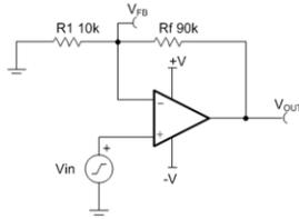
$$\frac{1}{\beta} = \frac{V_{OUT}}{V_{FB}} = \frac{R_F}{R_1} + 1 = 10 \text{ V/V}$$
