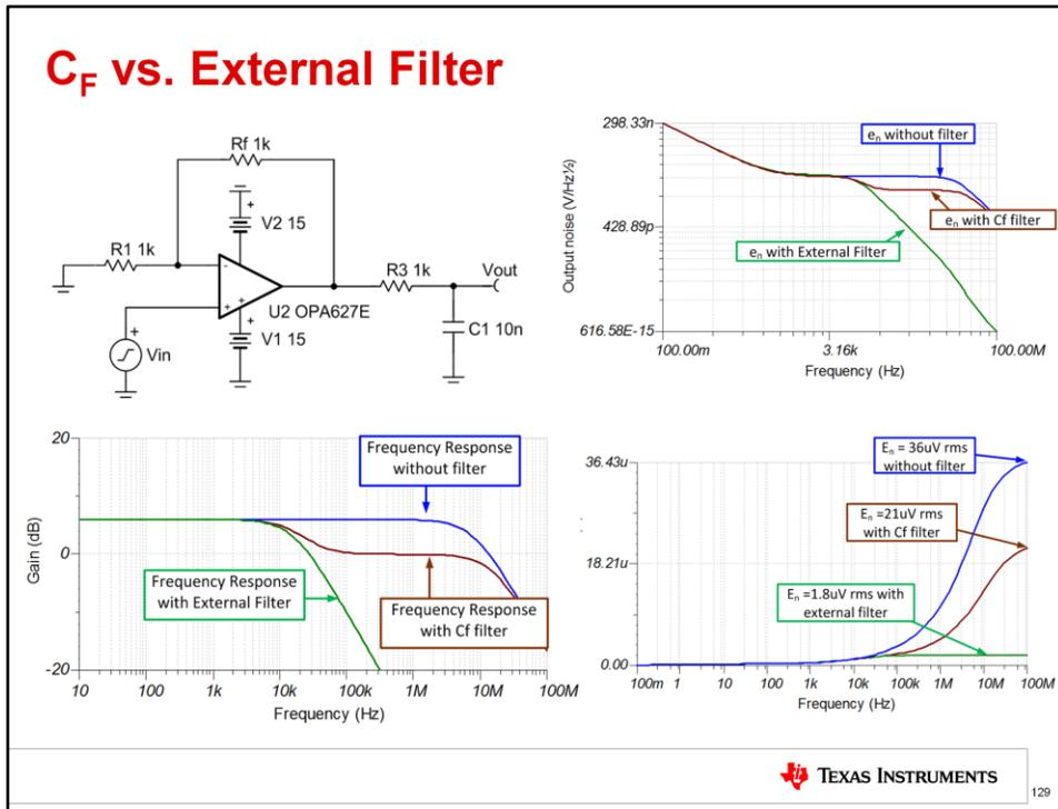
Using an external filter, which is a filter outside the op amp feedback loop, is the most effective way to reduce noise in circuits with low gain.
