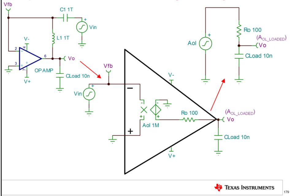
If we take a look at a simplified representation of the open-loop circuit, we see that the input signal passes through the  $A_{ol}$  gain block and then the series open-loop output impedance,  $R_o$ , before reaching the op-amp output,  $V_o$ . With a capacitor,  $C_{load}$ , on  $V_o$ , the op-amp loaded  $A_{ol}$  curve is divided down by an RC voltage divider.
