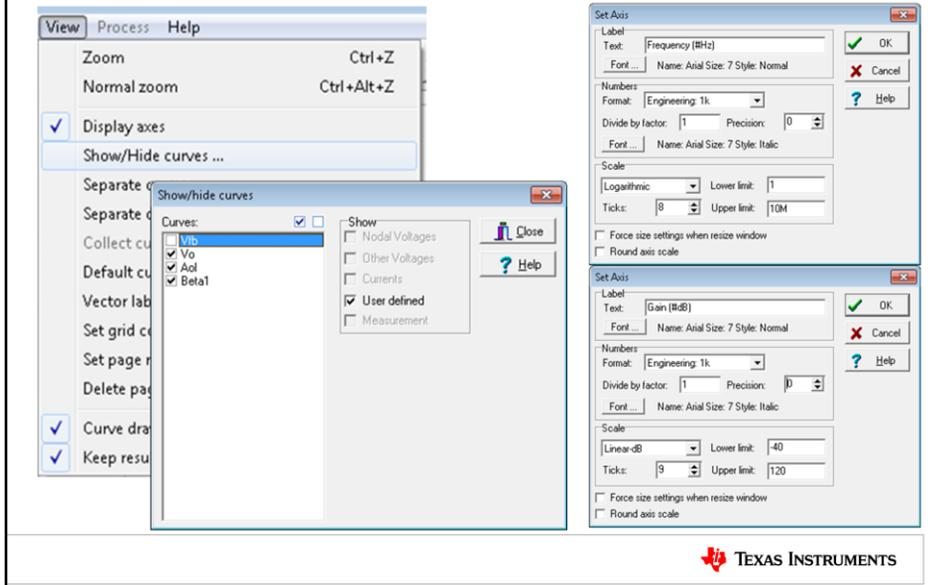
Click View, then Show/Hide curves. Select only the curves Vo, Aol, and Beta1. Then, double-click the x-axis and y-axis to bring up the “Set Axis” window. Change the x-axis to a logarithmic scale, 8 ticks, lower limit 1Hz, upper limit 10MHz. Change the y-axis to a linear-in-dB scale, 9 ticks, lower limit -40dB, upper limit 120dB.
