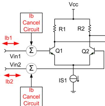
The input bias currents are mirrored and summed back in to cancel the bias current. This has the effect of significantly reducing input  $I_B$ . Note that when this is done,  $I_B$  can flow in both directions. Also,  $I_{B\_OS}$  is no longer smaller than  $I_B$ .
