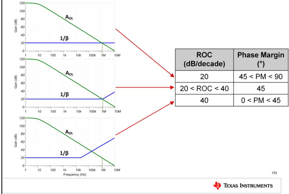
As shown in the previous slides, rate of closure and phase margin are closely connected. We can predict one value based on the other, and this slide gives three different examples of rate of closure and their corresponding phase margins.
