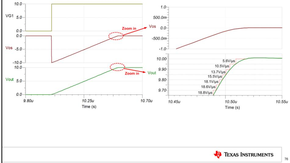
Let's take a closer look at the output of the non-inverting buffer circuit with a 10V step applied to the input.
