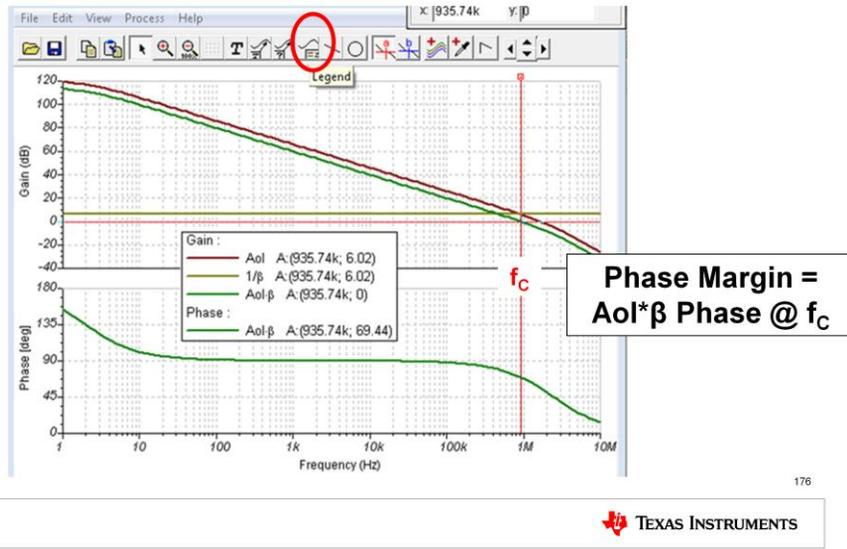
The final step is to measure the phase margin on the curves. The easiest method is to place a cursor on the  $A_{ol}\beta$  curve and then type "0" into the "y:" text box to set the cursor to the  $f_c$  frequency. Then click the "Legend" button and place it on the screen, which will display the phase of  $A_{ol}\beta$  at  $f_c$ . This is the phase margin.
