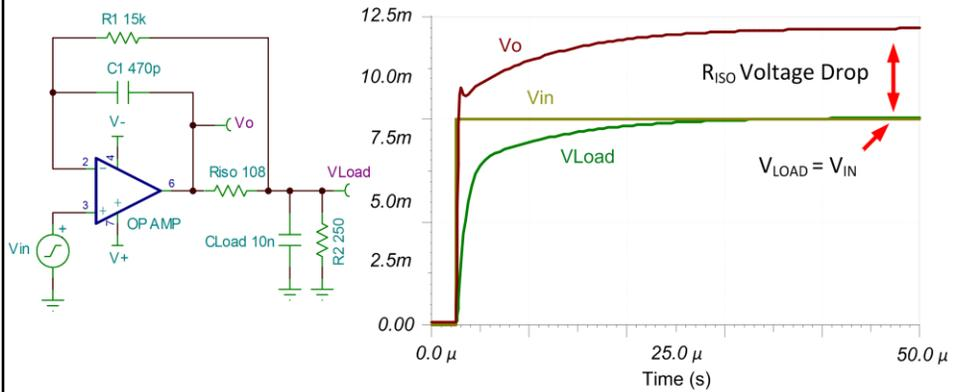
The results show that the output and load voltage arrive at the final level without excessive overshoot or ringing, indicating a stable system. The increase in  $V_o$  to overcome the voltage drop from  $R_{iso}$  can also be clearly seen here.
