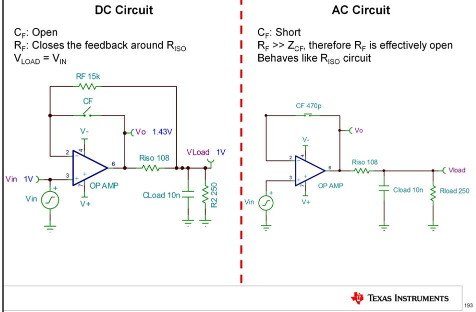
The Riso + dual feedback circuit works by having an equivalent circuit at both DC and AC.
