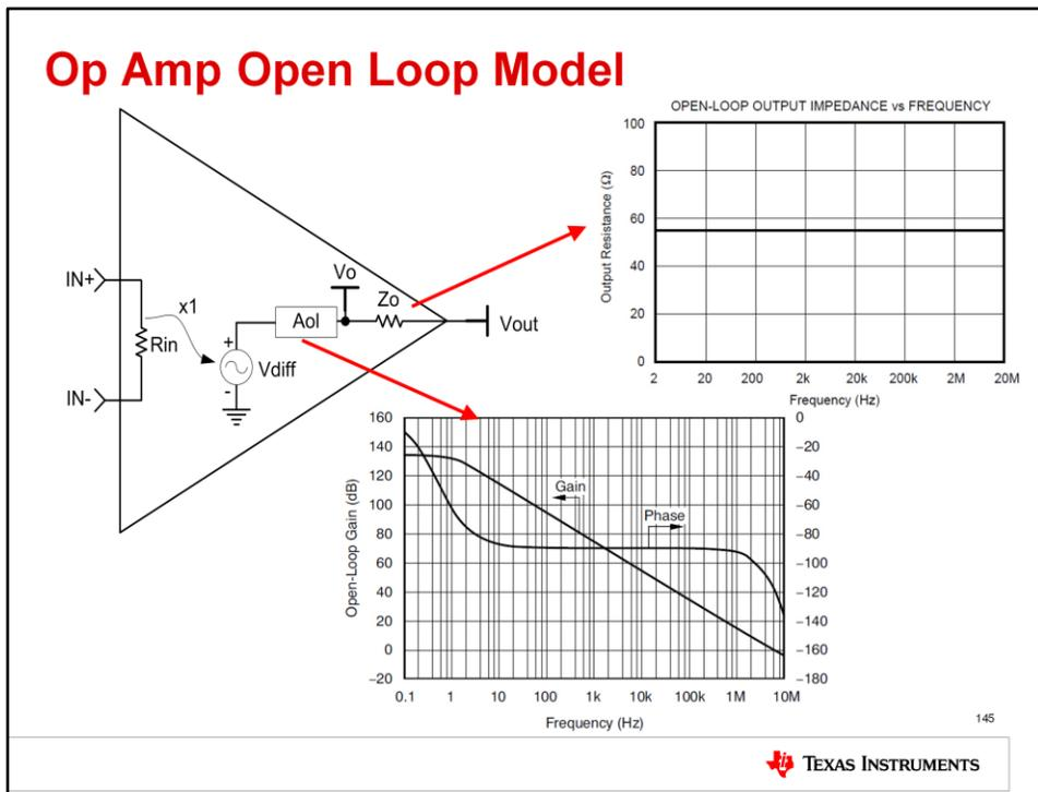
It is helpful to use an intuitive model for the op amp when performing ac stability analysis because of the complexity of modern op amps. In this simplified “stability” model, the differential input voltage applied to the inputs is passed to the amplifier output stage where it passes through the amplifier open-loop gain, followed by the open-loop output impedance before it reaches the output terminal.
