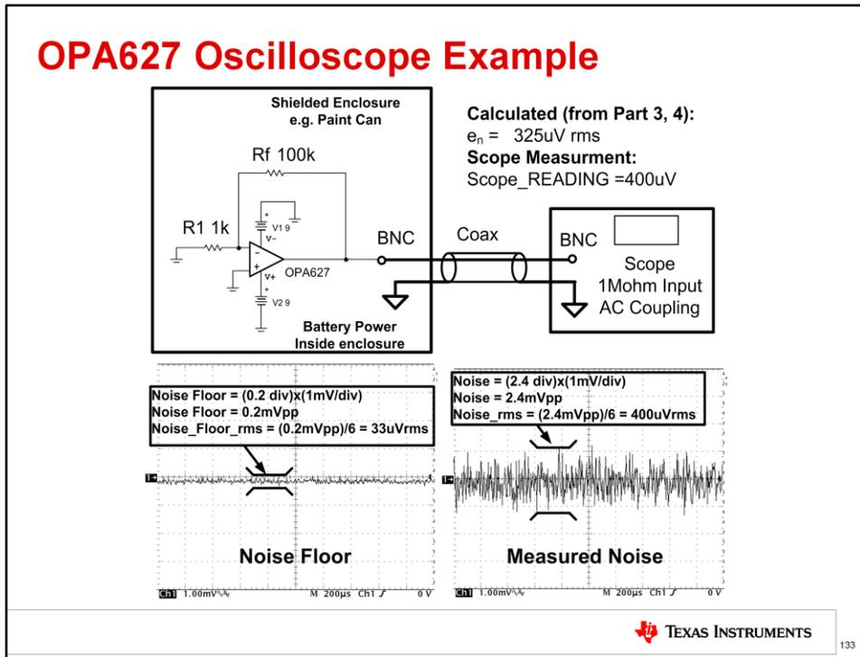
Let's now apply all of these real-world techniques to the OPA627 example circuit from our hand calculations and simulations. This circuit was connected directly to an oscilloscope with a BNC cable. As previously mentioned, the direct BNC connection is better than a 10x scope probe because the noise floor is ten times better.
