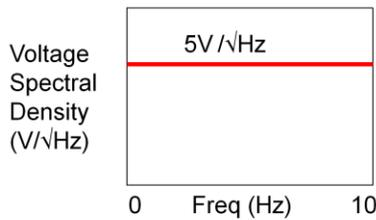
You can't integrate the **Voltage** spectral density curve to get noise
