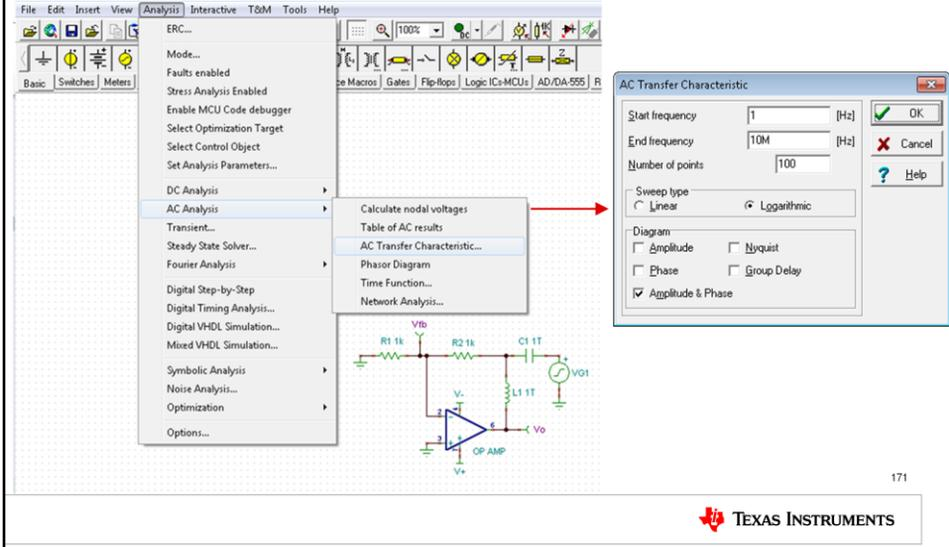
Once you've verified the DC functionality of the circuit, perform an AC transfer characteristic analysis over the op-amp bandwidth. Click Analysis, AC Analysis, AC Transfer Characteristic to do this.
