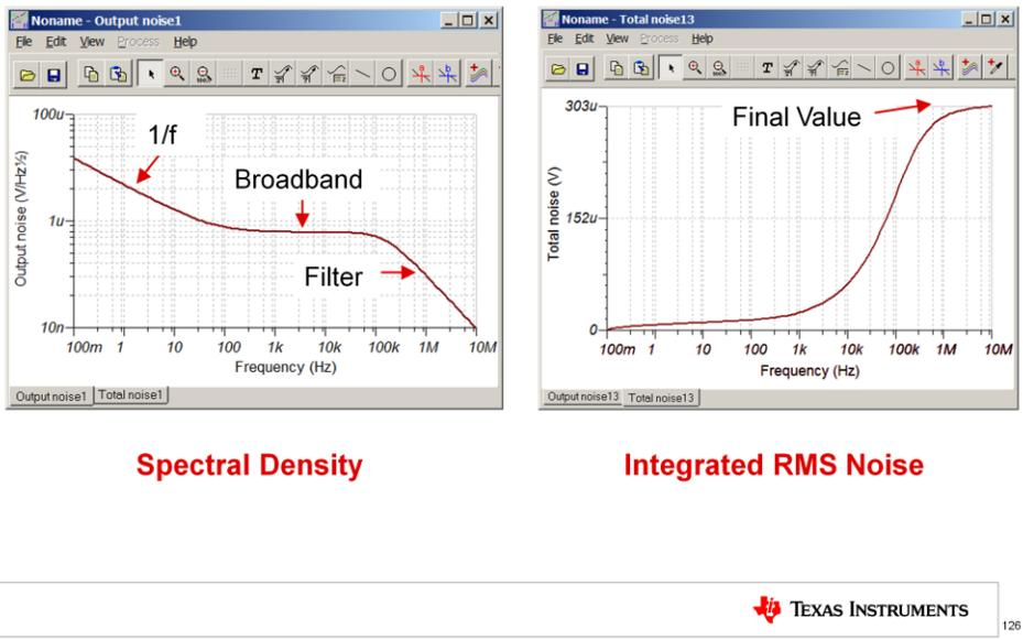
This slide shows the simulation results. The graph on the left is the spectral density plot, called “Output Noise” by TINA-TI. Note that the 1/f, broadband and filtered regions are clearly visible. The filtered region results purely from the op amp’s inherent bandwidth limitations, since there is no filter on the circuit.
