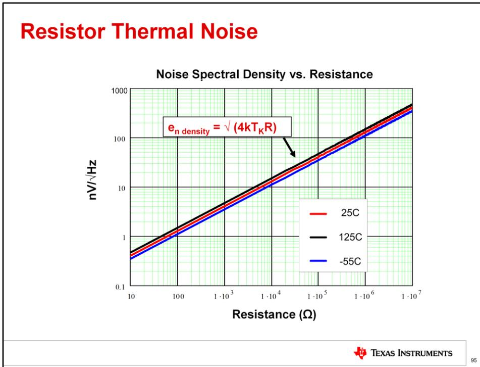
This plot was generated using the equation given in the last slide. Note that the equation was divided by the square root of bandwidth to give a spectral density, which is useful because it provides a quick way of comparing resistor noise to op-amp noise. Remember, most op-amps specify noise in nV/√(Hz).
