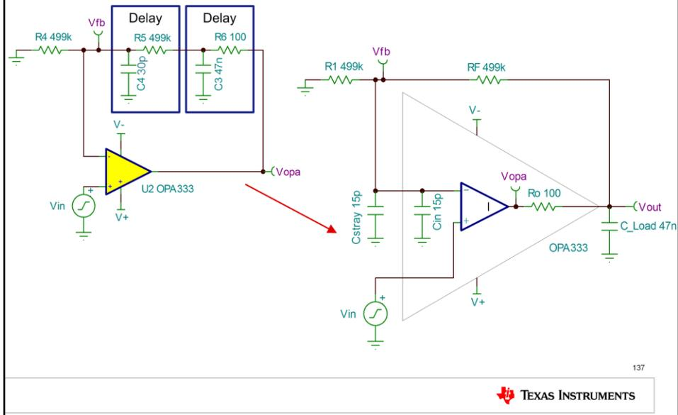
While the op amp circuit with the RC delay elements in the feedback path looks strange and unrealistic, many standard op amp circuits inadvertently create the same situation when external circuit components interact with non-ideal op-amp properties.
