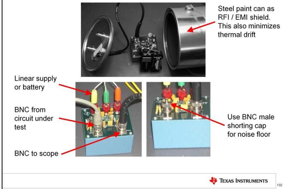
In addition to the proper configuration of oscilloscopes and spectrum analyzers, other aspects of your test setup can also have a huge impact on the quality of your noise measurement.
