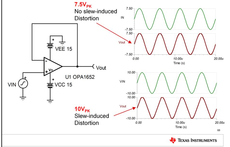
Let's simulate the conditions of the previous slide. With 7.5Vpk output, the response is sinusoidal with minimal distortion. However, with 10Vpk output, in a condition outside the full power bandwidth curve, the device is slew-rate limited and the output distorts.
