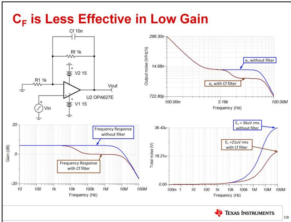
In this example the closed-loop gain is  $2\text{V}/\text{V}$  or  $6\text{dB}$ . The filter behaves in the same way, except that the effective attenuation when the capacitor is acting like a short is only  $6\text{dB}$ . In general, this type of filter will reduce the gain from the dc gain to a gain of  $1\text{V}/\text{V}$ . Thus, this filter is most effective for circuits with high gain.
