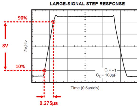
$$\text{Slew\_Rate} = \frac{\Delta V_{\text{out}}}{\Delta \text{Time}} = \frac{(V_{\text{out}90\%} - V_{\text{out}10\%})}{(t_{90\%} - t_{10\%})} = \frac{(9\text{V} - 1\text{V})}{(0.625\mu\text{s} - 0.35\mu\text{s})} = 29 \frac{\text{V}}{\mu\text{s}}$$
