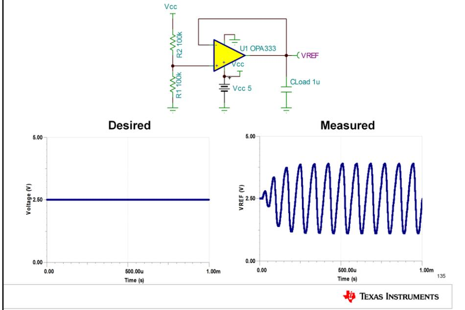
Here is an example of what can happen if a circuit's stability is not verified before going to production. An op amp circuit that is unstable will have an unpredictable or unexpected output with poor transient performance. This typically results in large overshoots and ringing when changes occur on the input or load, but may also result in sustained oscillations. Often stability problems are caused by connecting a capacitor to the output or to the inverting input of the amplifier.
