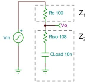
$$\frac{V_O}{V_{IN}} = \frac{Z_2}{Z_2 + Z_1}$$
