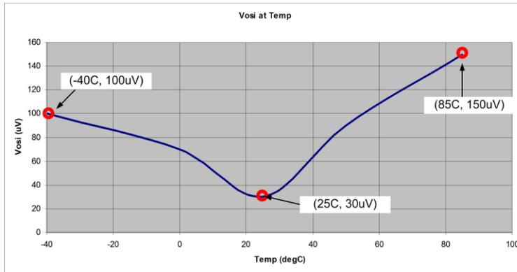
$$\frac{\Delta V_{os}}{\Delta T} = \frac{|V_{os}(T_1) - V_{os}(25C)| + |V_{os}(T_2) - V_{os}(25C)|}{|T_1 - T_2|}$$
