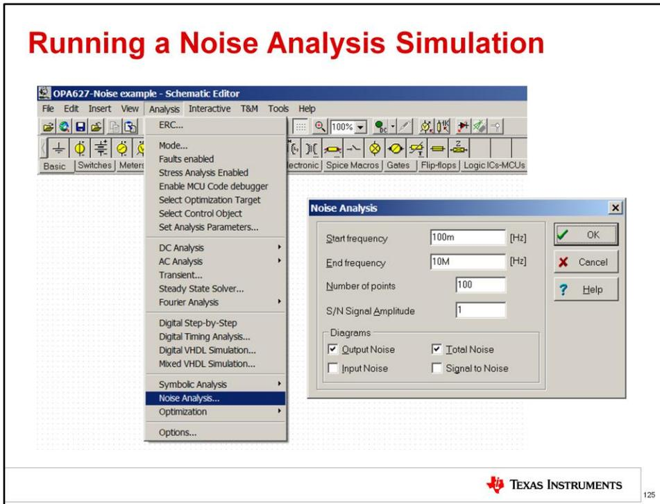
To run a noise analysis simulation in Tina SPICE, click “Analysis” in the menu bar, then click “Noise Analysis.” This brings up the “Noise Analysis” window. Enter the Start frequency and End frequency according to your application. In this example, we are analyzing the same circuit from the hand calculation in Noise 3. The bandwidth of this example circuit is 158kHz.
