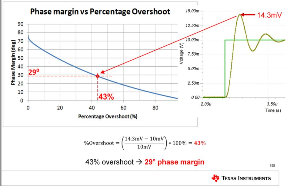
In the time domain the percent overshoot to a step input can be used to indirectly calculate the phase margin. In this example, a 10mV step was applied. The output overshoot reached 14.3mV, or 4.3mV above the intended output. This corresponds to a percent overshoot of 43%. Using the phase margin vs. percentage overshoot plot, we can see that 43% of overshoot results in only 29 degrees of phase margin.
