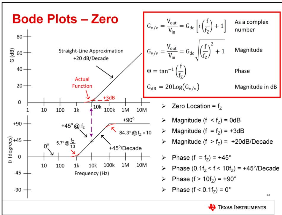
This slide illustrates the equations for a zero and its associated response. Looking at the equations, you can see that the first equation represents a zero as a complex number. Complex numbers have a real and imaginary part. For practical circuits the complex function is converted to a magnitude and phase. The second equation shows the magnitude and the third equation shows the phase. Taking 20 Log10 of the magnitude function gives the magnitude in dB.
