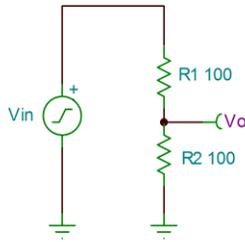
$$\frac{V_O}{V_{IN}} = \frac{R_2}{R_2 + R_1}$$
