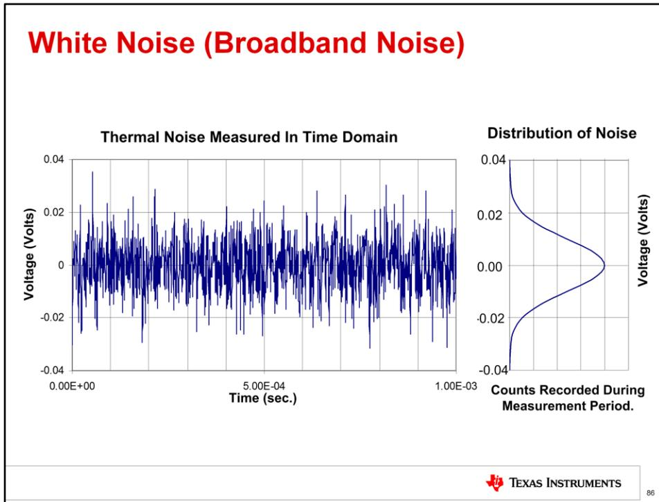
This slide shows the time domain waveform for white noise, also known as broadband noise. The time domain waveform is what you would see if you measured noise with an oscilloscope. Notice that the horizontal axis is 1ms, full scale. Taking the reciprocal of the full-scale time gives a frequency of 1kHz. In general, broadband noise is considered to be in the middle to high frequency range; that is, frequencies greater than 1kHz. In the next slide we'll consider lower frequency noise sources.
