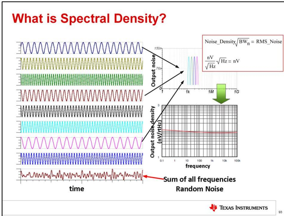
Do you remember that white light is the combination of all colors? Well, white noise is the combination of all frequencies. This figure shows that when you add several signals of different frequencies together in the time domain, the result is a random looking signal. In the frequency domain, each one of these signals looks like an impulse. Combining an infinite number of these signals across all frequencies creates what is called a noise spectral density curve.
