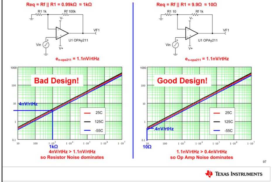
Let's compare resistor/thermal noise to op amp noise in two different circuits.
