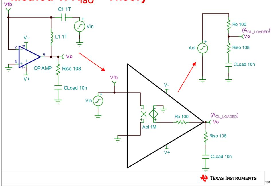
We can look at the  $R_{ISO}$  circuit the same way we looked at the original circuit. Here we see another voltage divider on the  $A_{ol}$  output. This time there are two elements,  $R_{iso}$  and  $C_{Load}$ , on the bottom of the divider and  $R_o$  on the top leg of the divider.
