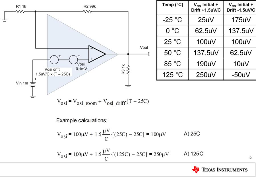
Offset drift calculations can be done in a similar manner. Notice that we have two sources: one for the initial offset and one for the offset drift. The offset drift source will be zero at 25C. As the temperature deviates from 25C, the temperature difference will be multiplied by the offset drift to generate the additional offset voltage.
