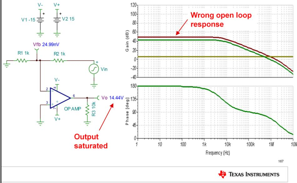
However, a circuit without feedback will not simulate properly because the output will go to one rail or the other. This causes incorrect Aol or output characteristics to be displayed. As shown here, the op-amp output is near the positive rail, resulting in an erroneously Aol curve.
