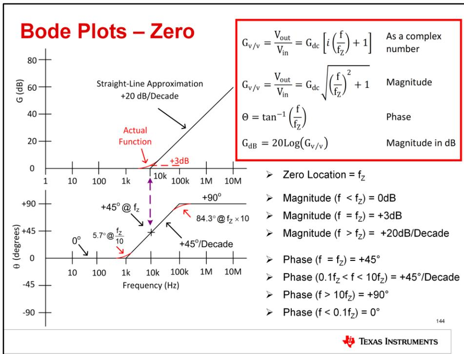
This slide, also from the op-amp bandwidth lecture, illustrates the equations for a zero and its associated magnitude and phase response on Bode plots. A zero causes a positive 20dB/decade increase in the slope of the magnitude response after the zero frequency,  $f_z$ . The zero also causes a positive 90 degree phase shift in the phase response beginning roughly a decade before  $f_z$  and ending roughly a decade afterwards.
