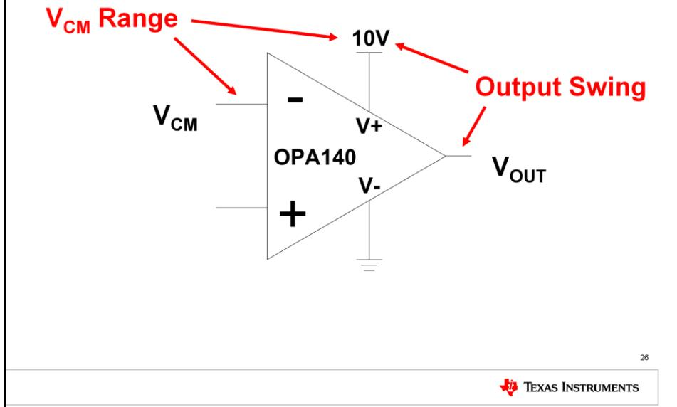
Common mode input voltage range is also known as input voltage swing. This term describes the range of input common mode voltages that can be used for normal linear operation of the amplifier. The common mode input voltage range is always defined relative to the positive supply and the negative supply. When you exceed the common mode input range, the output becomes nonlinear.
