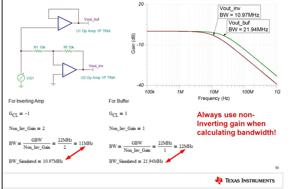
Earlier we calculated closed loop bandwidth for a non-inverting configuration using the gain bandwidth product. You might be surprised to learn that the bandwidth calculation for the *inverting* configuration is calculated using the *non-inverting gain*. Note that the non-inverting gain is typically referred to as noise gain.
