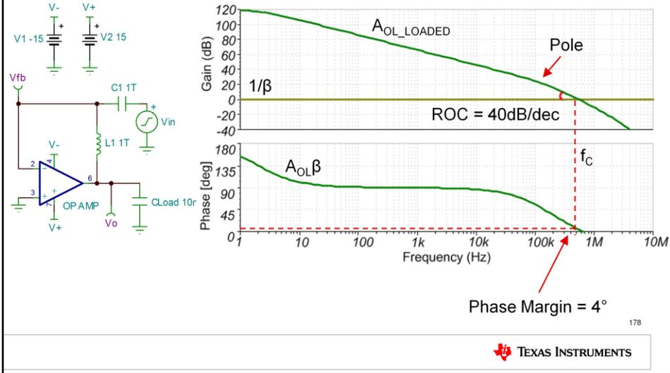
Using the steps shown previously, we ran an open-loop simulation on the circuit shown here with a 10nF capacitor on the op amp output. As the results show, the 10nF capacitive load results in a pole in the  $A_{ol}$  curve which degrades the  $A_{ol}*\beta$  phase to only 4 degrees at  $f_c$ . Let's examine why this happens.
