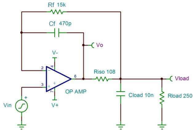
A solution to the voltage drop problem from the  $R_{iso}$  circuit is to implement the “ $R_{iso}$  + Dual Feedback” circuit shown here.
