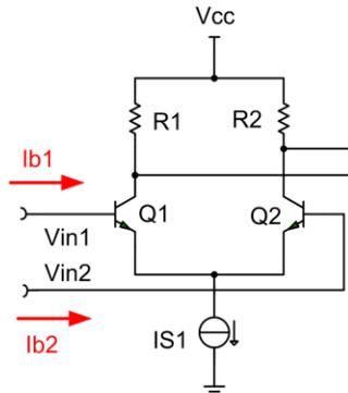
Bias current in bipolar amplifiers is from input transistor base current. It is typically larger than in FET-input amplifiers and it flows into the input terminals.
