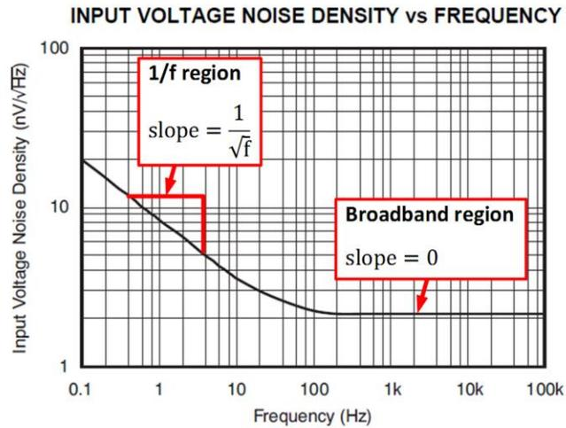
The spectral density curve has two regions: the 1/f region and the broadband region. 1/f noise occurs at low frequency, and has a slope of one divided by the square root of frequency for both voltage and current spectral density. Remember that power spectral density is voltage spectral density squared, so for power spectral density the slope of 1/f noise is equal to one divided by frequency. This is where it gets the name 1/f. Broadband, or white noise, has a flat spectral density.
