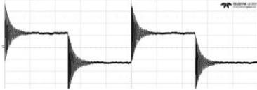
Sustained Output Oscillation with DC Input
