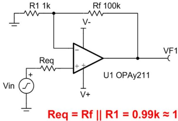
The parallel combination of  $R_f$  and  $R_1$  act like a resistance on the op amp's non-inverting input.
