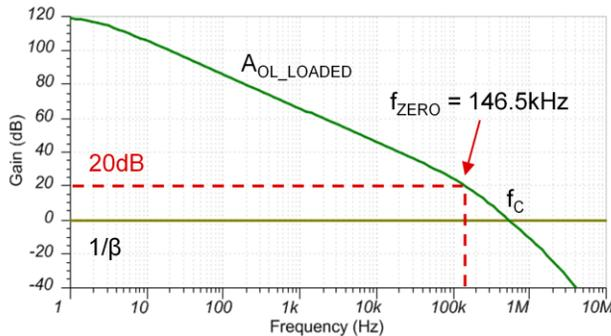
To design the  $R_{iso}$  circuit for between 60 and 90 degrees of phase margin (depending on the op amp unity-gain phase margin and location of the  $A_{ol}$  pole), first find the frequency where the Loaded  $A_{ol}$  curve is equal to 20dB,  $f(A_{ol} = 20\text{dB})$ . Using the  $R_{iso}$  equations shown on the left and plugging in the values for  $C_{load}$  and  $f(A_{ol} = 20\text{dB})$ , the  $R_{iso}$  value is calculated to be  $108\Omega$  in this example.
