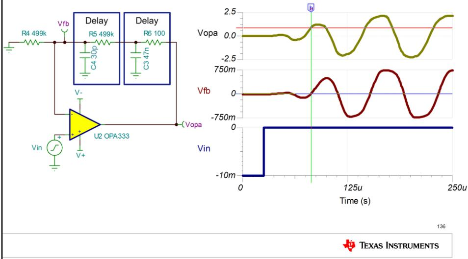
Too much delay between the amplifier output and the inverting feedback node is a straightforward way to visualize the root cause of op amp stability issues.
