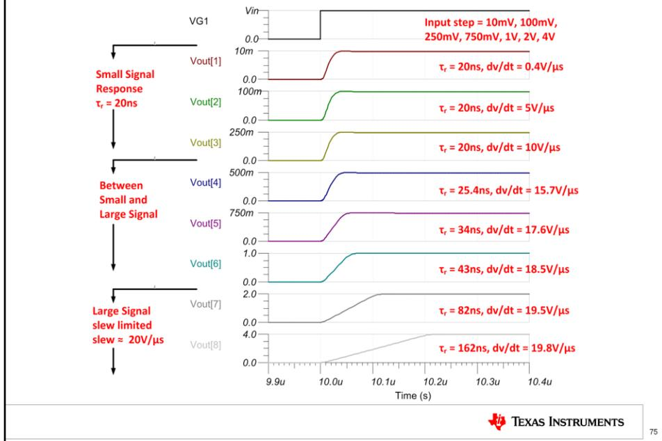
This figure illustrates the output of the non-inverting buffer circuit from the previous slide, versus different input step sizes.
