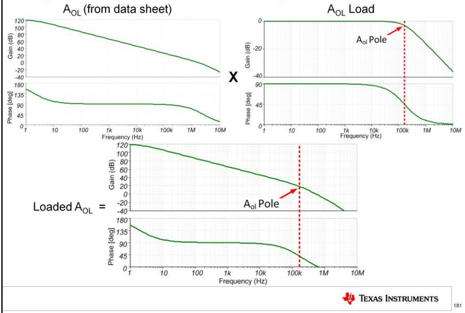
If the original op amp A<sub>OL</sub> curve and the A<sub>OL</sub> load curve are combined, the result is the loaded A<sub>OL</sub> curve shown on the bottom. As shown, the pole from the interaction of R<sub>o</sub> and C<sub>load</sub> causes a change to a -40dB/decade A<sub>OL</sub> magnitude slope and a degraded unity-gain phase margin.
