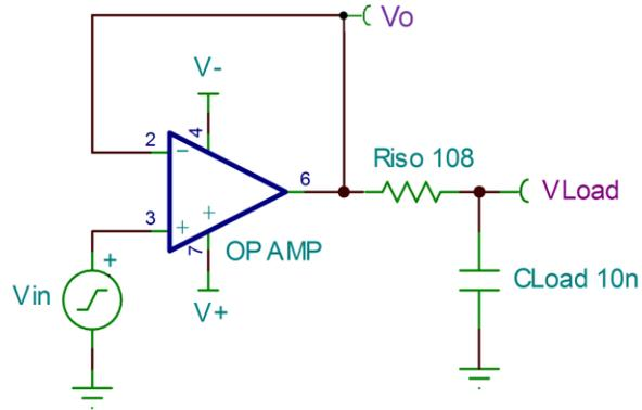
The Riso method is quite simple. It works by adding a zero to the Aol curve to cancel the pole from  $R_o$  and  $C_{load}$ .
