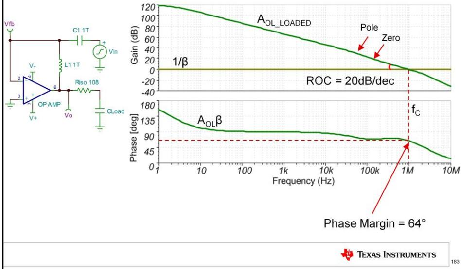
Looking at the open-loop results from the “Riso” compensation method, a zero can be seen cancelling the pole from Riso and Cload. This results in a return to a 20dB/decade Aol slope and significantly improved phase margin.
