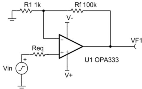
$$f_c = \frac{GBW}{\text{Gain}} = \frac{350\text{kHz}}{101} = 3.5\text{kHz}$$
