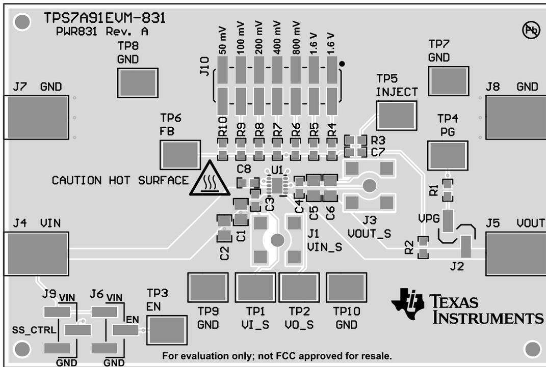
Figure 1. Assembly Layer
