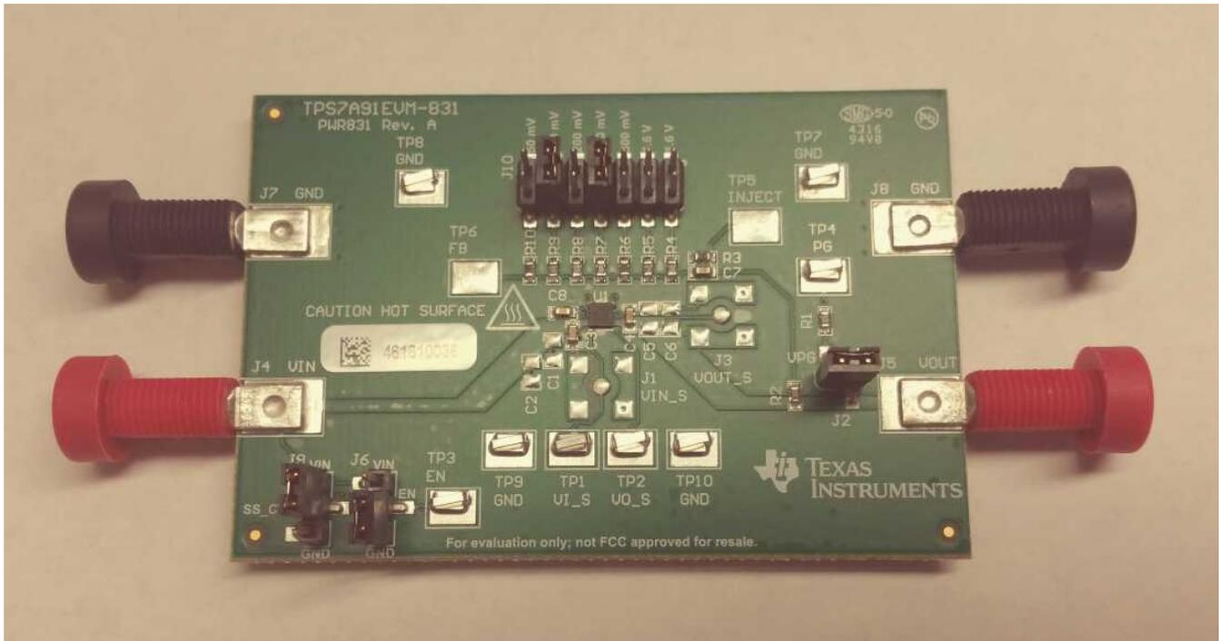
This user's guide describes the operational use of the TPS7A91EVM-831 evaluation module (EVM) as a reference design for engineering demonstration and evaluation of the TPS7A9101DSK, low-dropout linear regulator (LDO). Included in this user's guide are setup and operating instructions, thermal and layout guidelines, a printed-circuit-board (PCB) layout, a schematic diagram, and a bill of materials (BOM).
