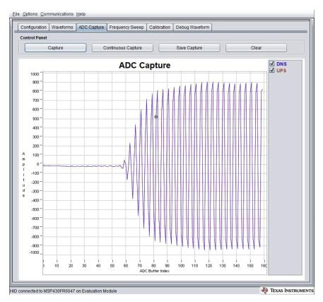
Figure 4-8. Gap Between Pulse Start and ADC Capture Set Too Short
