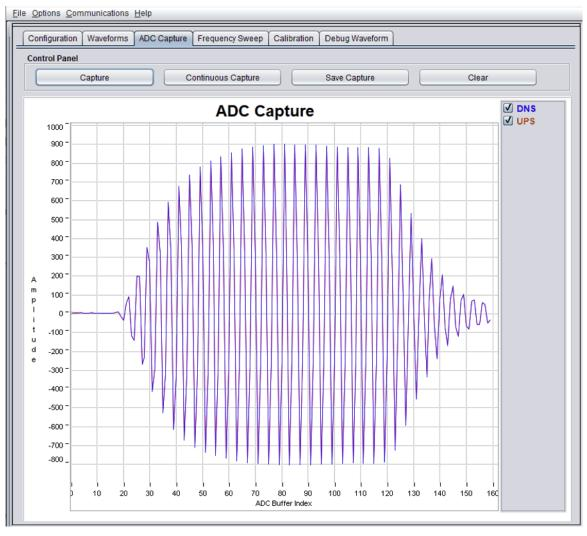
Figure 4-6. Captured ADC Signal
