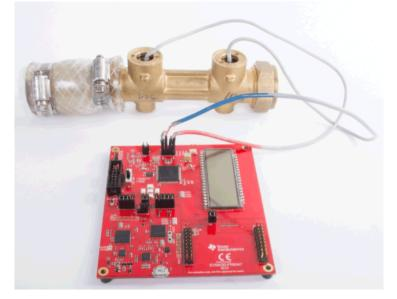
Figure 2-1. EVM430-FR6047 Connected to Flow Meter
