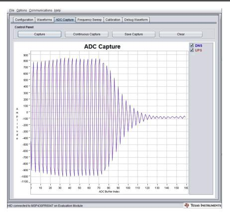
Figure 4-7. Gap Between Pulse Start and ADC Capture Set Too Long
