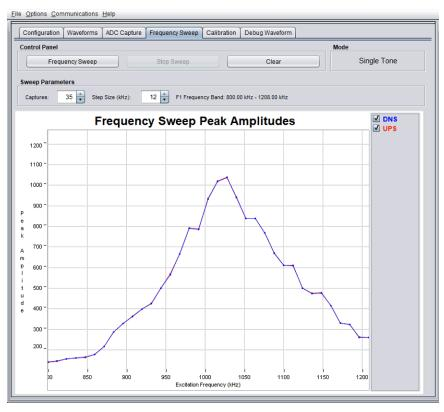
Figure 4-11. Frequency Sweep Peak Amplitudes
