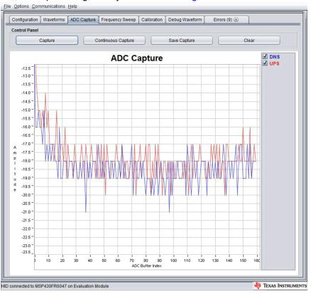
Figure 4-9. Captured ADC Signal With No Water or Bad Connection
