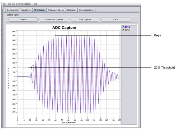
Figure 4-5. Representative Captured Waveform With Interpolation
