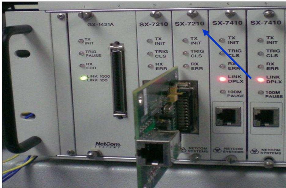
Figure 4. MII Card Connected to the SmartBits 2000
