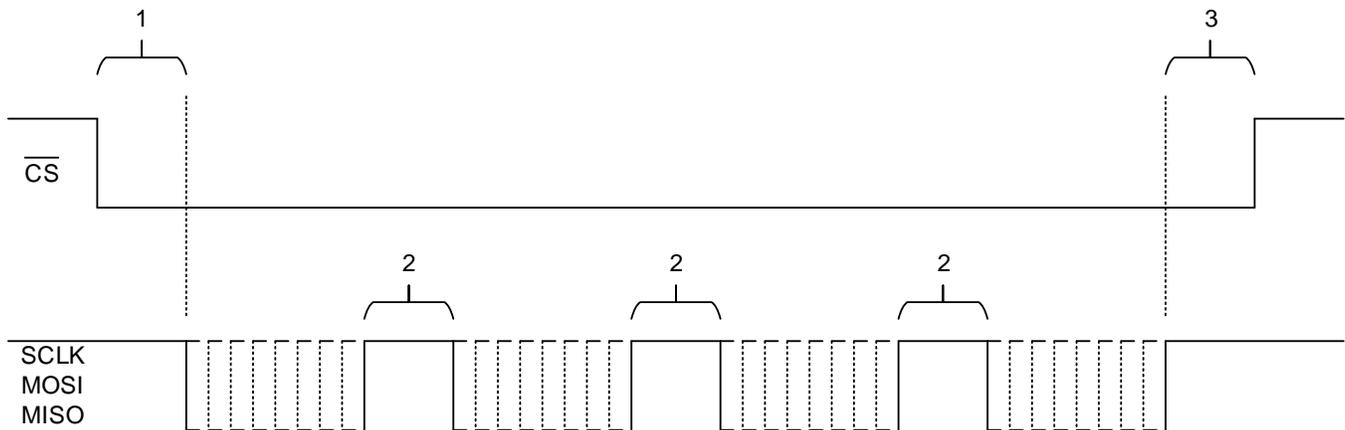
**Figure 13. An Example Inefficient SPI Transfer**
