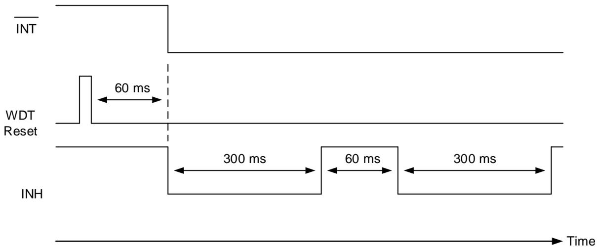
**Figure 4. Example Watchdog Timer Behavior (60 ms and INH output)**
