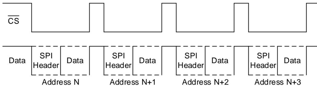
**Figure 15. Inefficient Transfer of Large Data**
