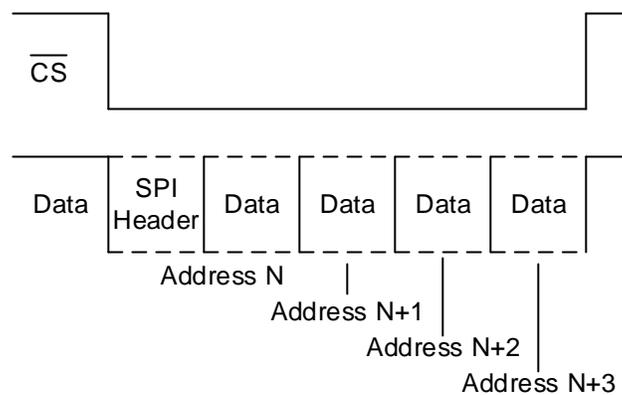
**Figure 16. Efficient Transfer of Large Data**
