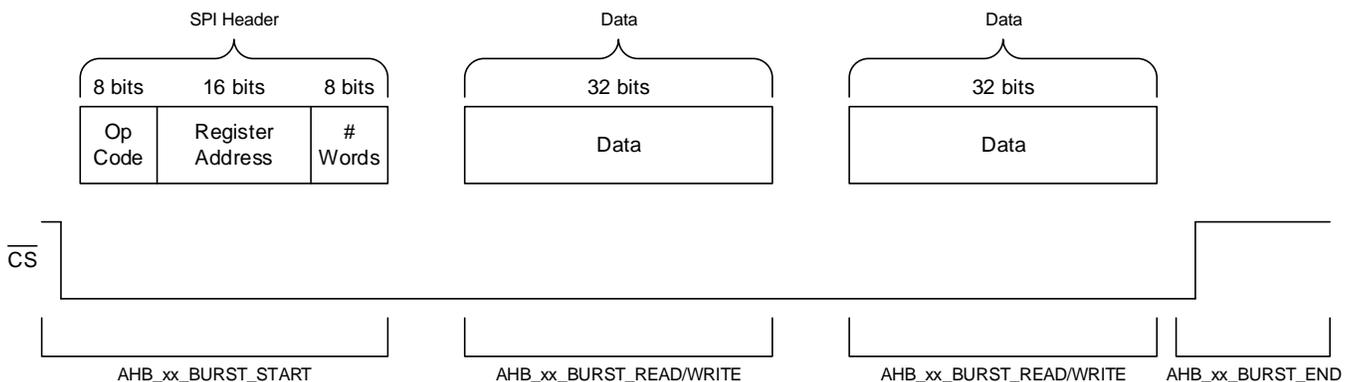
**Figure 21. Multi-word SPI Packet Example**
