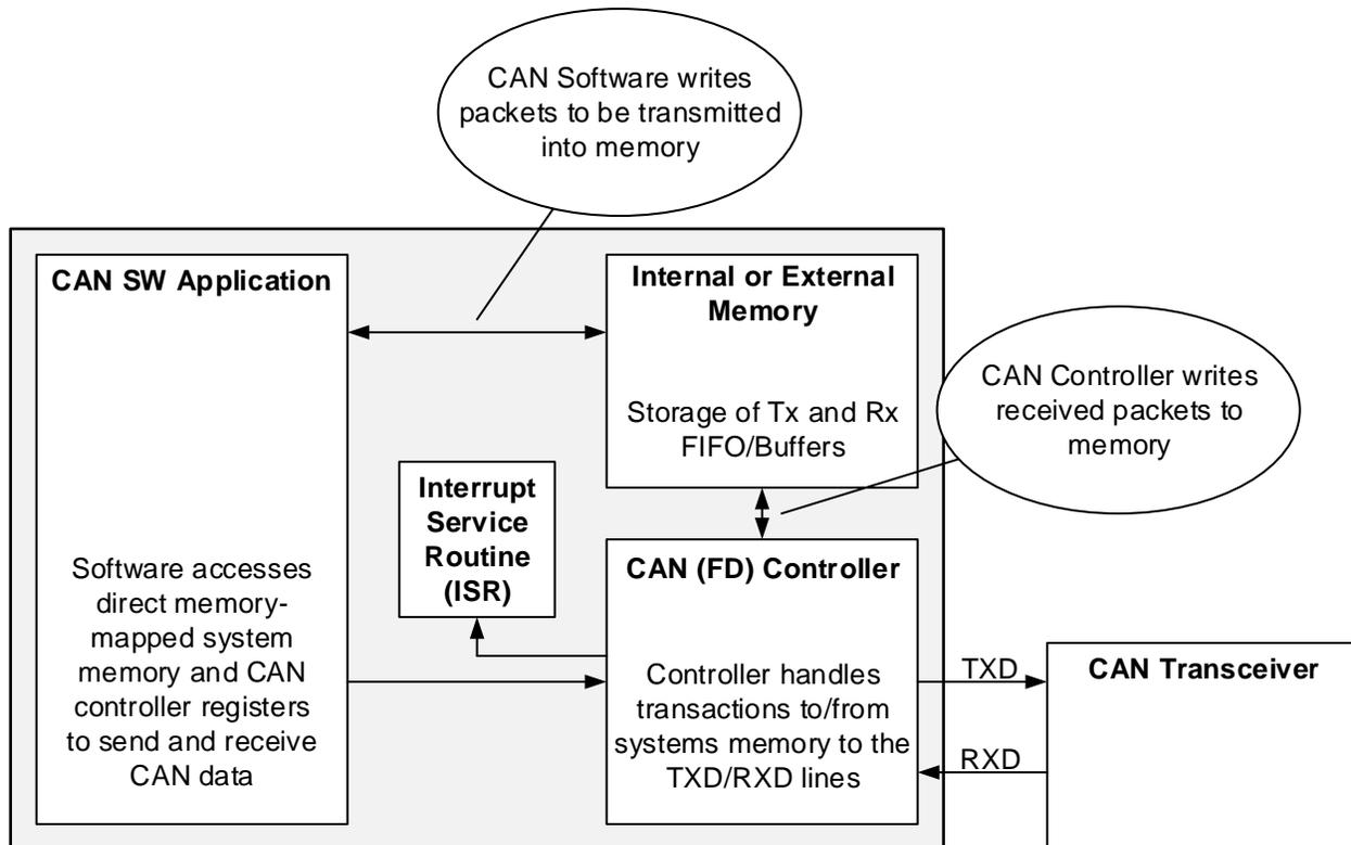
**Figure 1. Integrated CAN Application**
