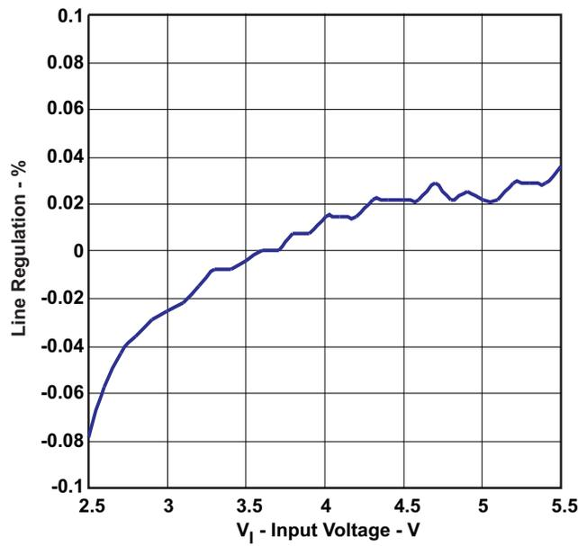
Figure 5. Line Regulation ( $V_{OUT} = 1.4V$ ,  $I_{OUT} = 1.5A$ )
