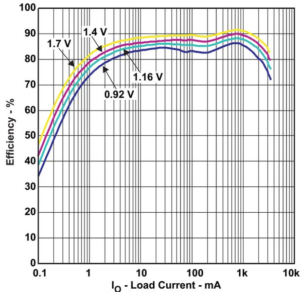
Figure 3. Efficiency vs. Output Current ( $V_{IN} = 3.6V$ ,  $V_{OUT} = 0.92, 1.16, 1.4, 1.7$ )
