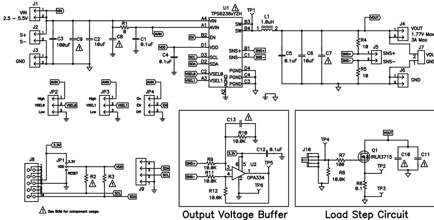
Figure 17. TPS6236xEVM-655 Schematic
