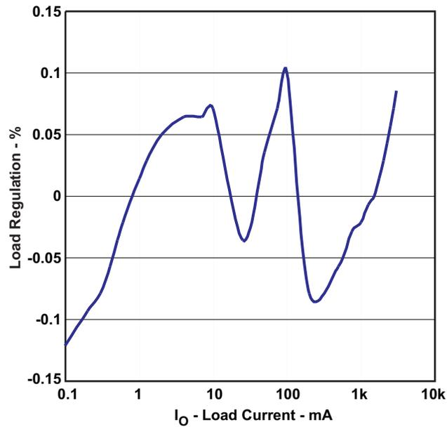
Figure 4. Load Regulation ( $V_{OUT} = 1.4V$ ,  $V_{IN} = 3.6V$ )
