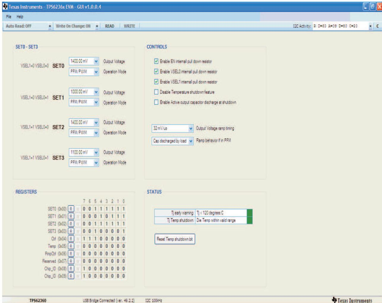
Figure 1. TPS6236x Software Main Panel
