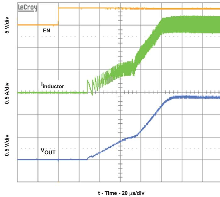
Figure 6. Start-up ( $V_{IN} = 3.6V$ ,  $V_{OUT} = 1.4V$ ,  $I_{OUT} = 1.5A$ )
