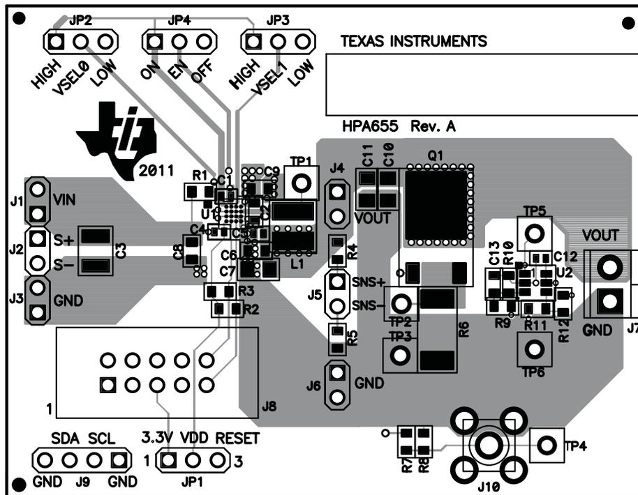
Figure 12. Assembly Layer
