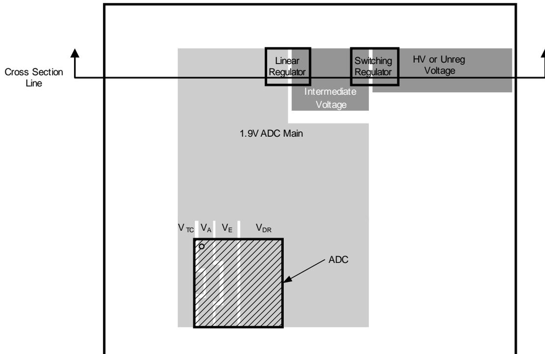
Figure 11. ADC Regulators and Power Planes
