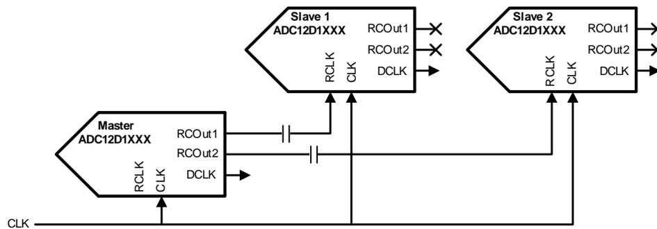
**Figure 7. AC-Coupling the AutoSync RCLKs**
