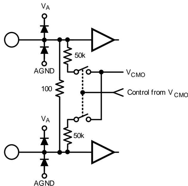
**Figure 1. Analog-Input Equivalent Circuit**
