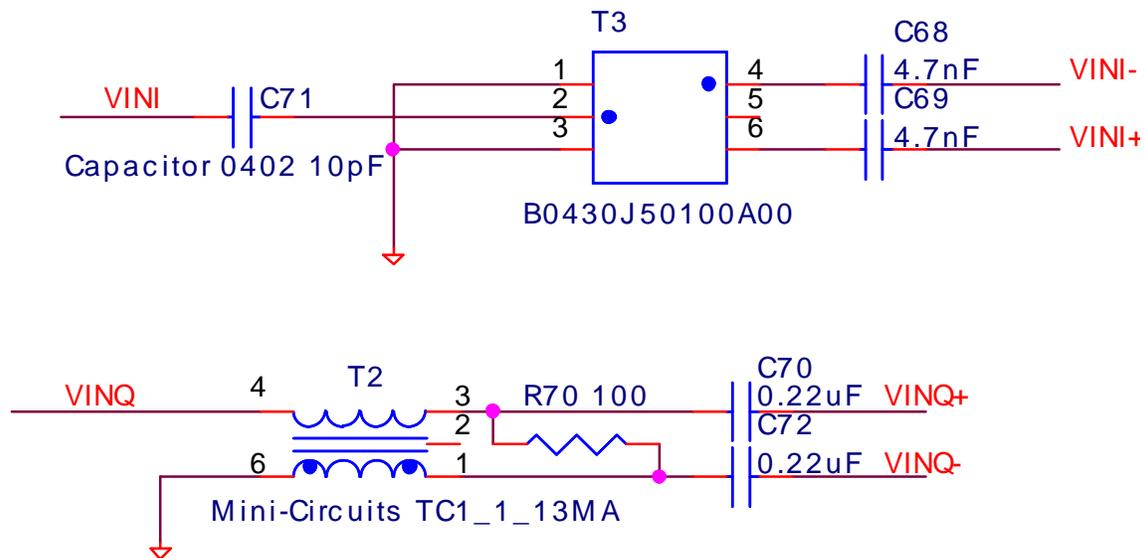
Figure 2. Balun Driving Analog-Input Schematics
