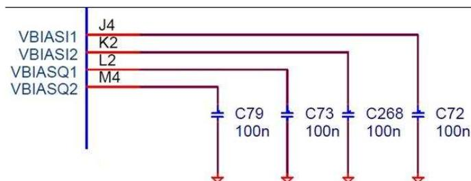
**Figure 13. VbiasI and VbiasQ in ADC1xDxxx(RF)RB**
