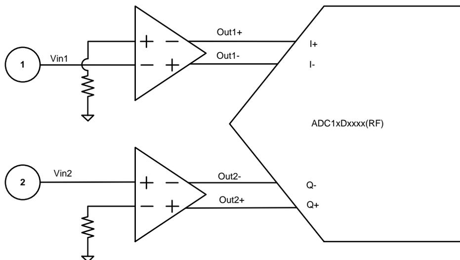
**Figure 5. Driving the ADC With Differential Amplifiers to Maintain Polarity**
