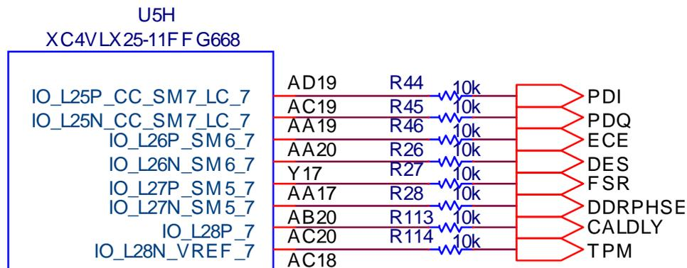
Figure 9. FPGA Driving the Control Pins on the ADC1xDxxxx(RF)RB
