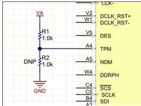
Figure 8. Example of Control Pin Set by Rails
