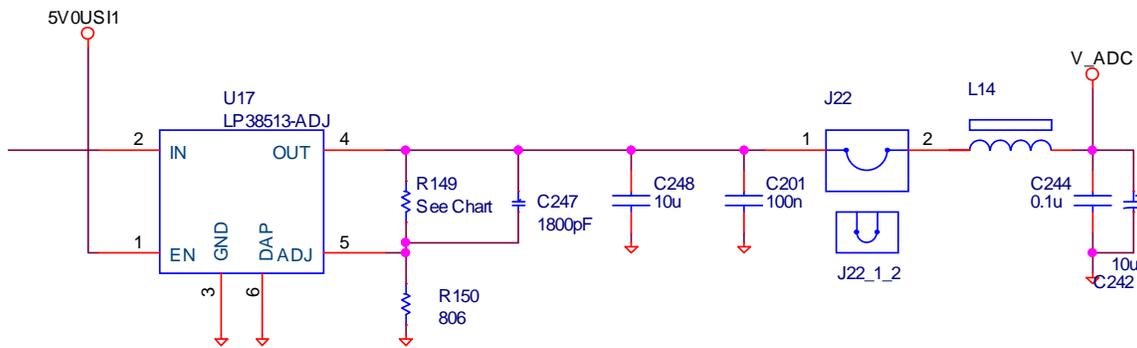
Figure 10. LDO Supplies ADC Power On the ADC1xDxxxx(RF)RB
