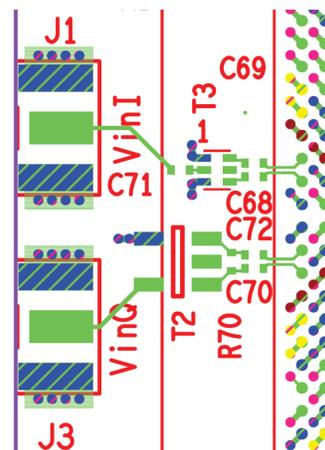
Example Balun Circuits for Analog Inputs
