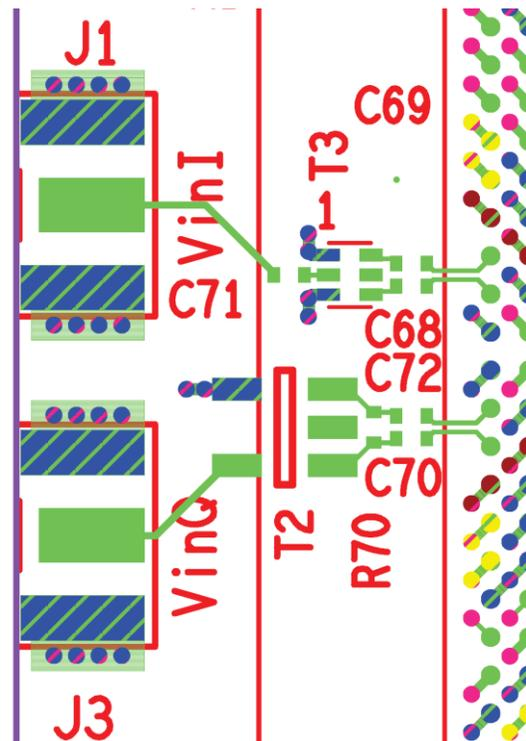
Figure 3. Balun Driving Analog-Input Layout
