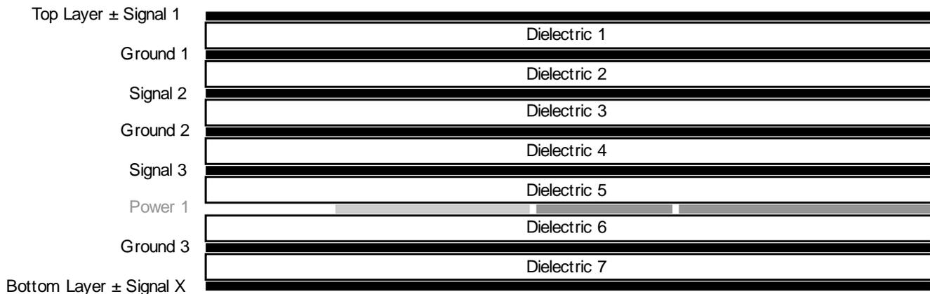
**Figure 12. ADC1xDxxx(RF)RB Stack Up**
