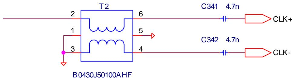
Figure 6. Driving the Sampling Clock on the ADC1xDxxxx(RF)RB
