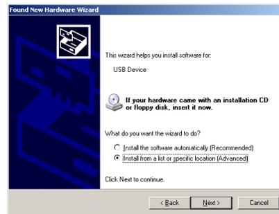
Figure 10: Install driver from specific location
