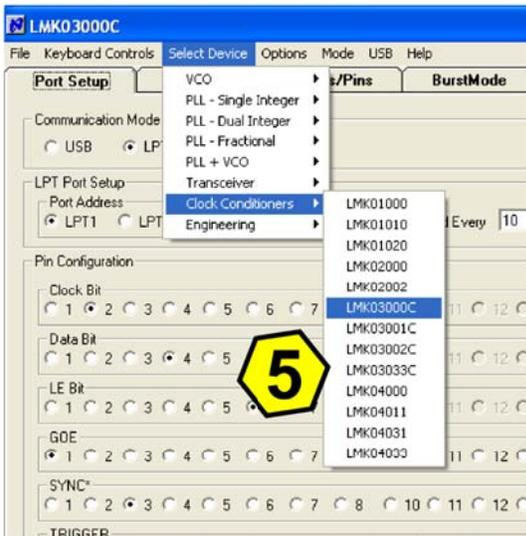
Figure 2 - Selecting the evaluation board to be used.
