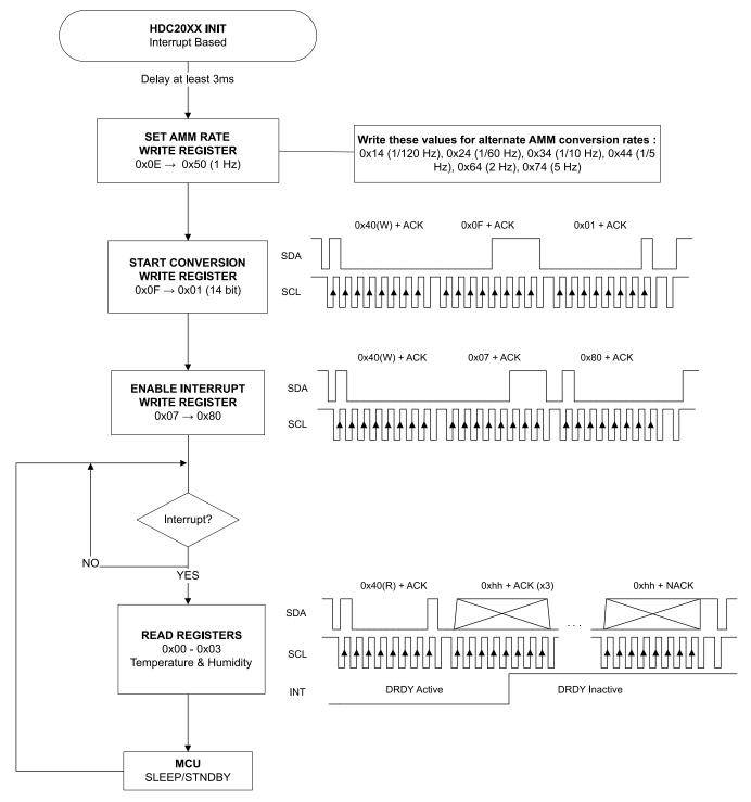
Figure 3-3. Flowchart for continuous data acquisition when using interrupt based polling
