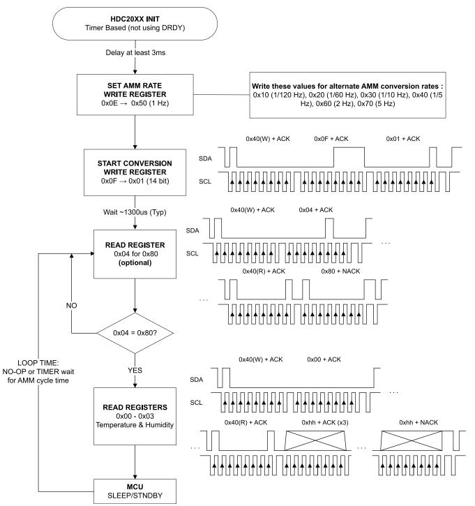
Figure 3-2. Flowchart for continuous data acquisition when using timer based polling
