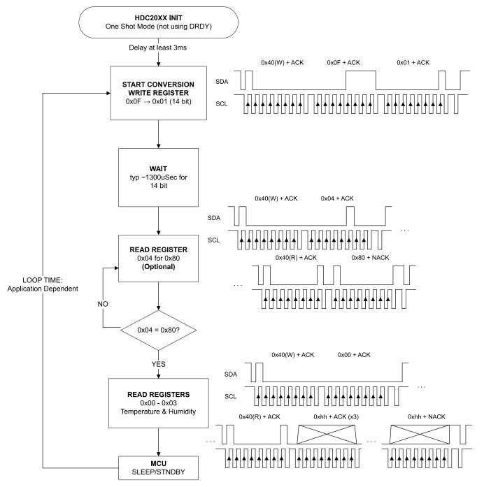
Figure 3-1. Flowchart for single data acquisition mode
