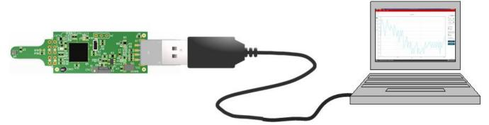
Figure 16. TMP117EVM Connection Diagram
