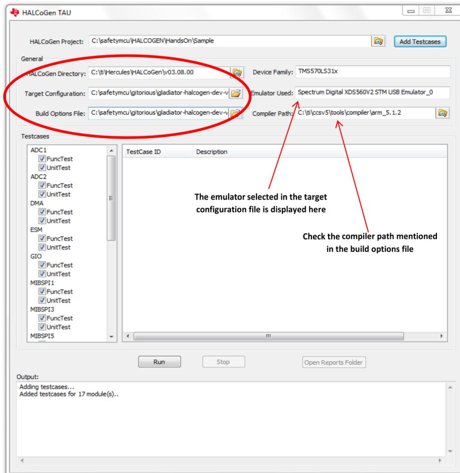
Figure 8. Target and Build Option Selection
