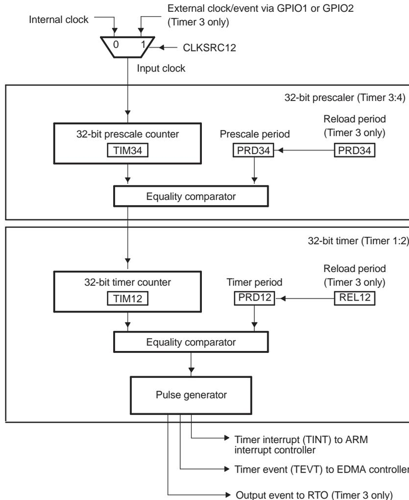
**Figure 5. Dual 32-Bit Timers Chained Mode Example**
