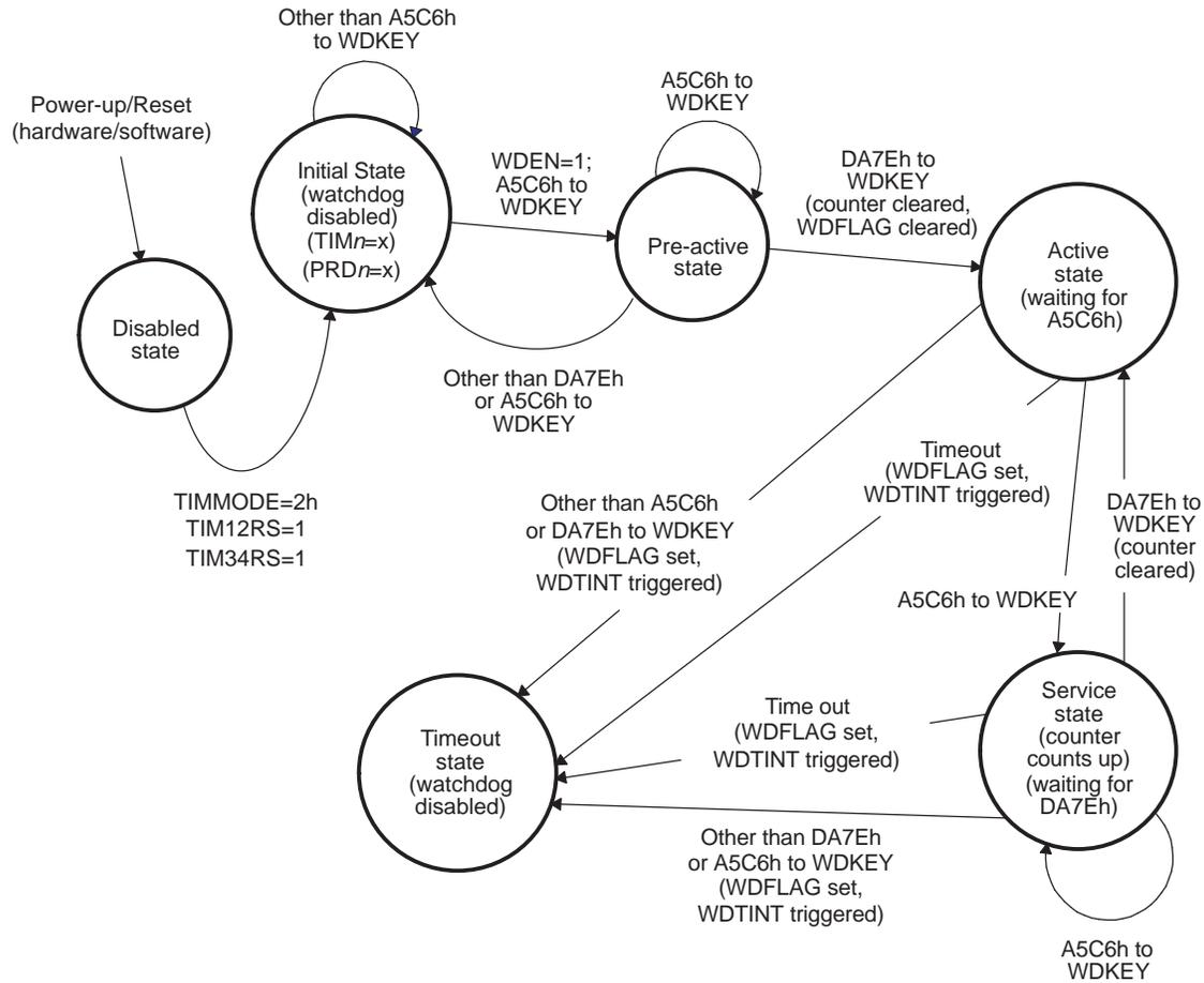
To prevent a watchdog timeout event, the timer has to be serviced periodically by writing A5C6h followed by DA7Eh to the watchdog timer service key (WDKEY) bits in WDTCR before the timer finishes counting up. Both A5C6h and DA7Eh are allowed to be written to the WDKEY bits, but only the correct sequence of A5C6h followed by DA7Eh to the WDKEY bits services the watchdog timer. Any other writes to the WDKEY bits triggers the watchdog timeout event immediately.
