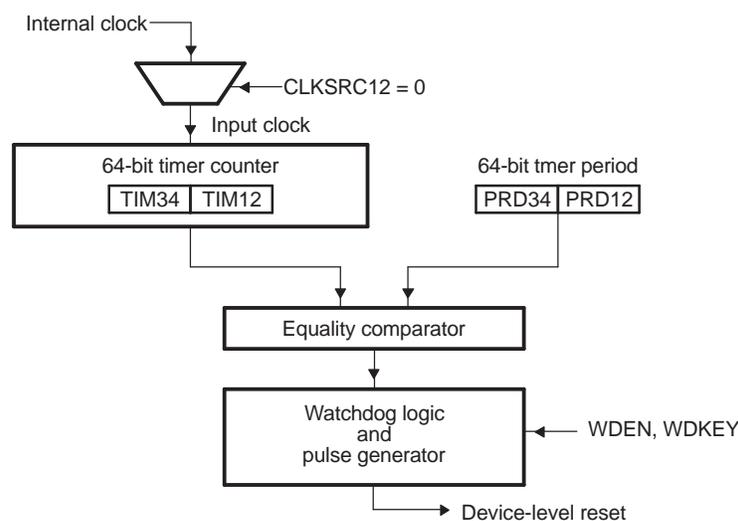
**Figure 10. Watchdog Timer Operation State Diagram**
