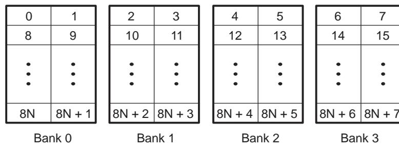
For devices that have more than one memory space ([Figure 5-2](#)), an access to bank 0 in one memory space does not interfere with an access to bank 0 in another memory space, and no pipeline stall occurs.
