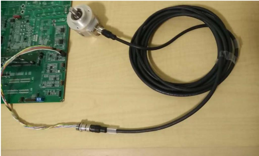
**Figure 10. M12 Heidenhain Cable Connects to the Encoder**
