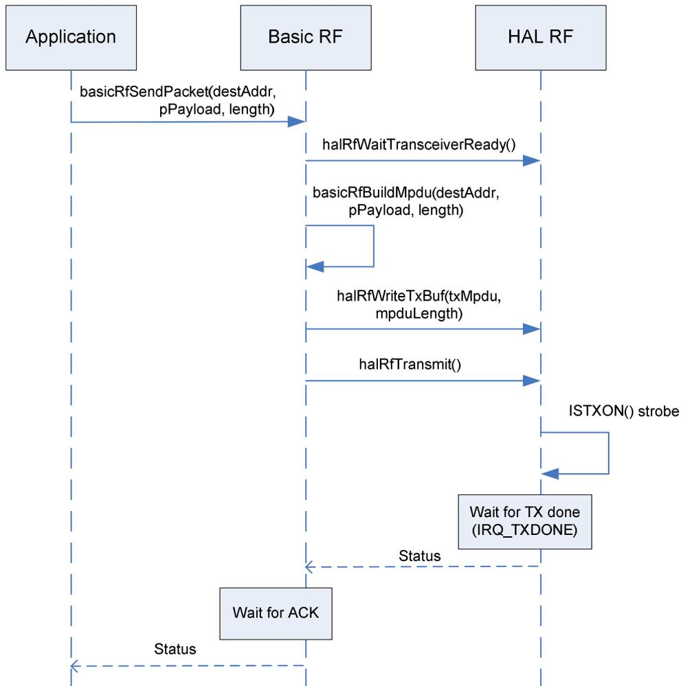
Figure 9 Packet transmission
