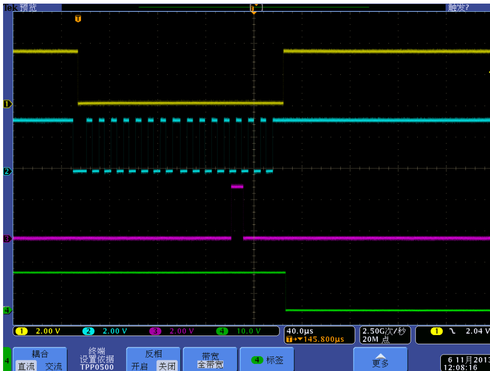
Fig 4, Send output data to turn on OUT4 of #1 with a 12V relay connected
