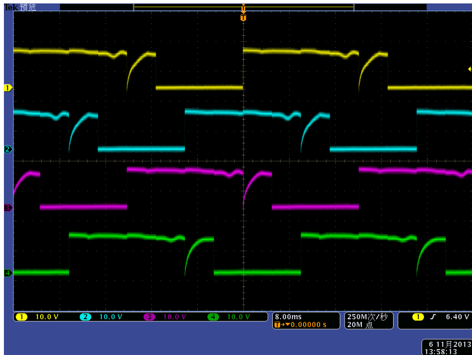
(Yellow: OUT1 #1; Blue: OUT2 #1; Purple: OUT3 #1; Green: OUT4 of #1) Fig 21, Half step commutation output pattern with stepper connected
