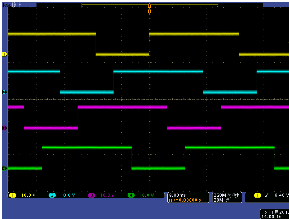
(Yellow: OUT1 #1; Blue: OUT2 #1; Purple: OUT3 #1; Green: OUT4 of #1) Fig 19, Half step commutation output pattern without motor connected
