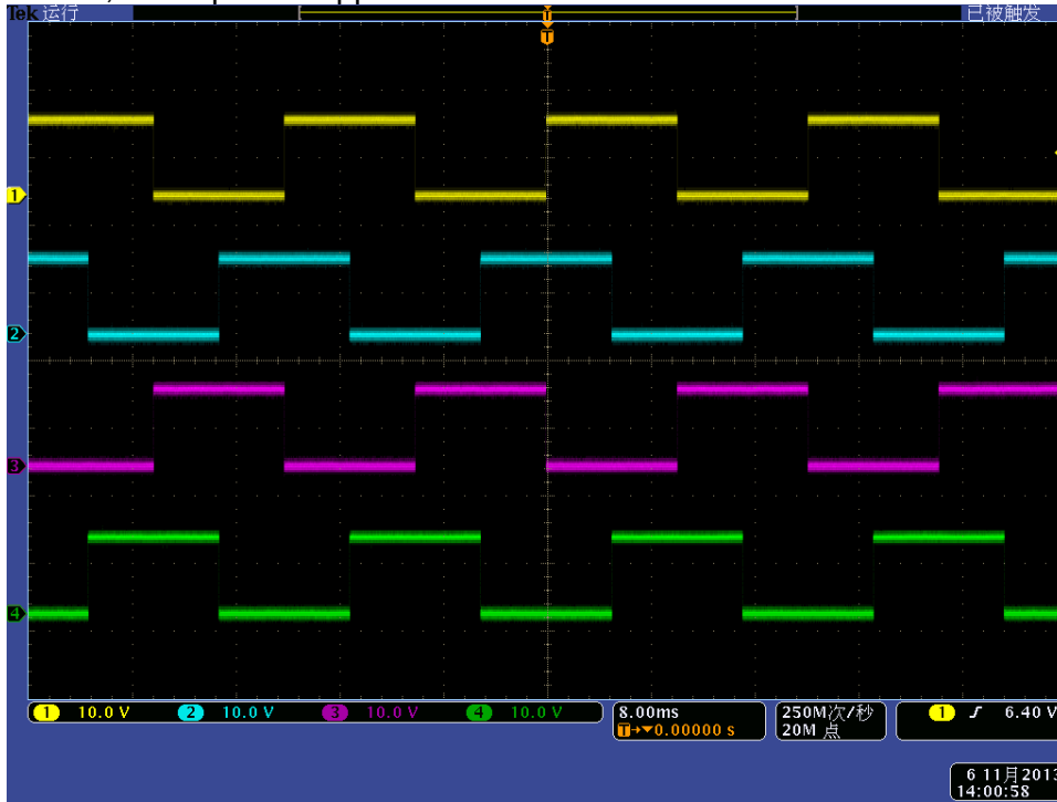
(Yellow: OUT1 #1; Blue: OUT2 #1; Purple: OUT3 #1; Green: OUT4 of #1) Fig 18, Full step commutation output pattern without motor connected
