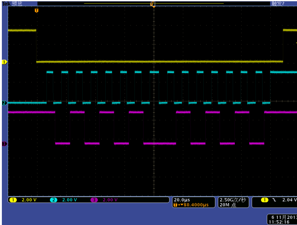
Fig 1, Send 0x55 (#1) and 0xAA (#2) to two DRV8860s in daisy chain connection.
