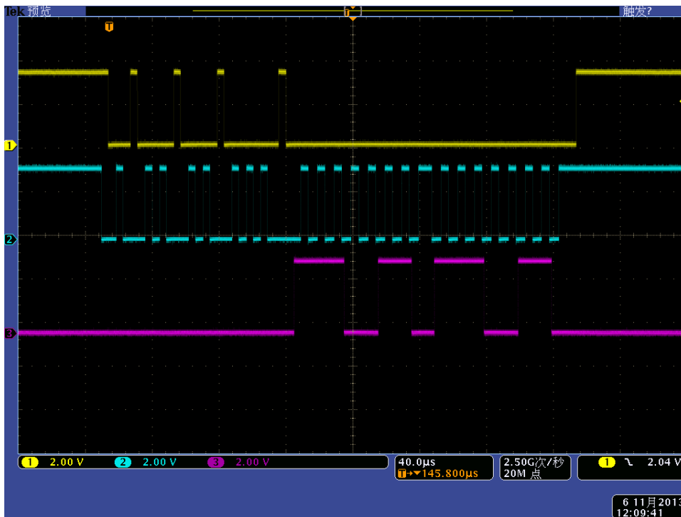
Fig 5, Send control register for 30ms energizing time followed by 75% duty
