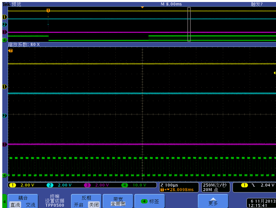
Fig 8, OUT4 output with 30ms energizing time followed by 50% PWM duty. (Control register: 0xC6)
