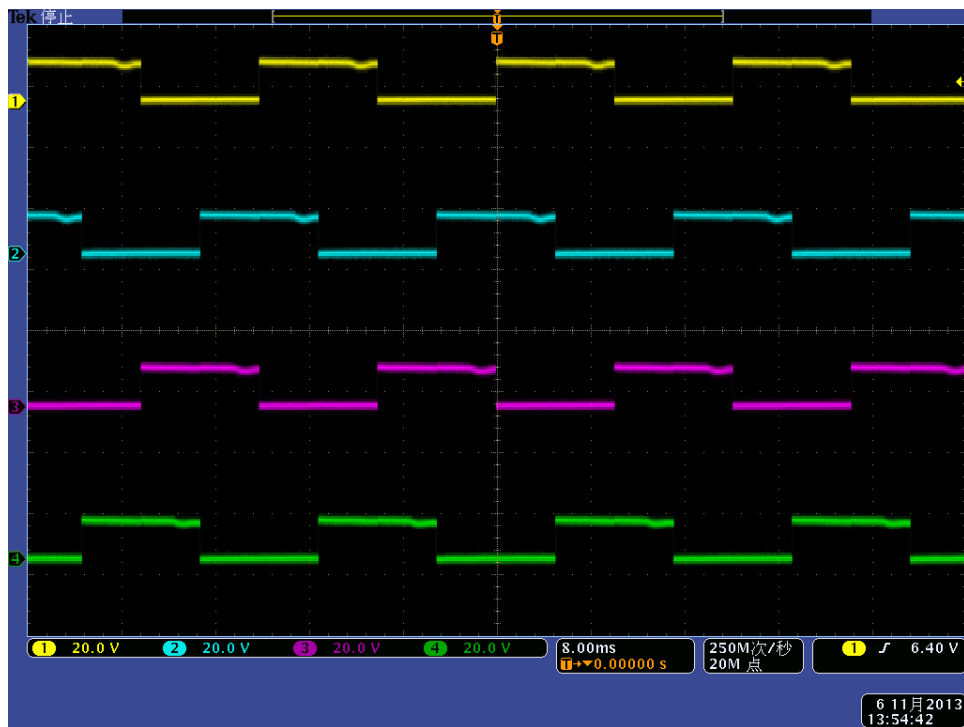
(Yellow: OUT1 #1; Blue: OUT2 #1; Purple: OUT3 #1; Green: OUT4 of #1) Fig 20, Full step commutation output pattern with stepper connected
