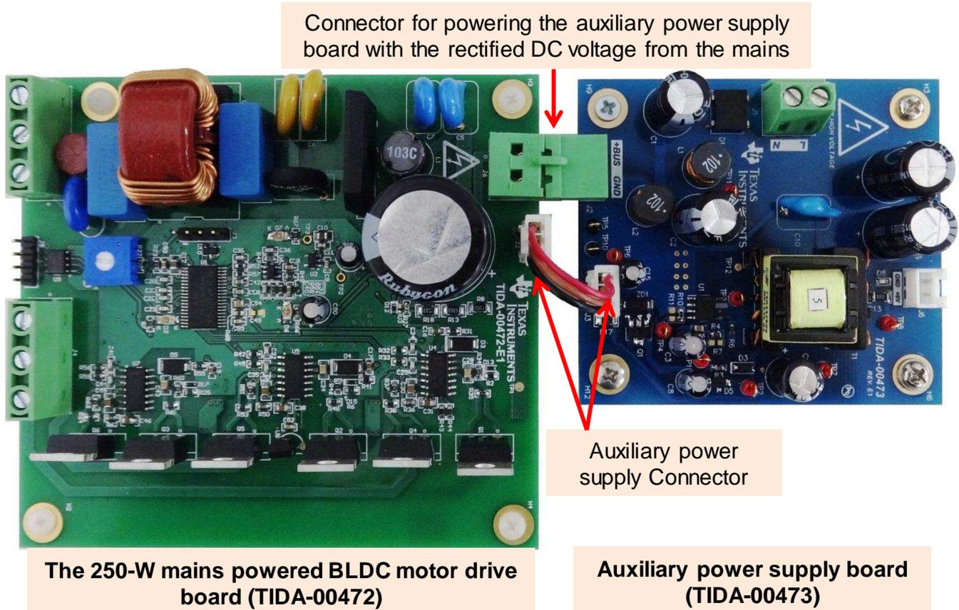
**Figure 20. Interfacing TIDA-00472 and TIDA-00473**
