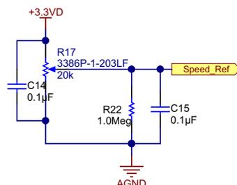
Figure 15. Potentiometer Connection for Speed Control
