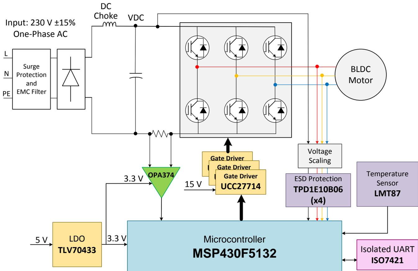
Figure 1. Block Diagram of Mains-Powered 250-W BLDC Drive (TIDA-00472)
