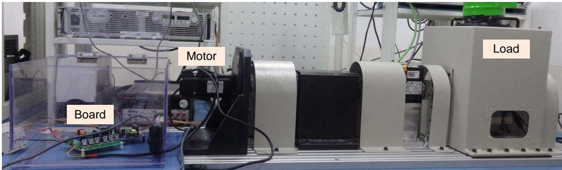
Figure 29. Test Setup for Board and Motor
