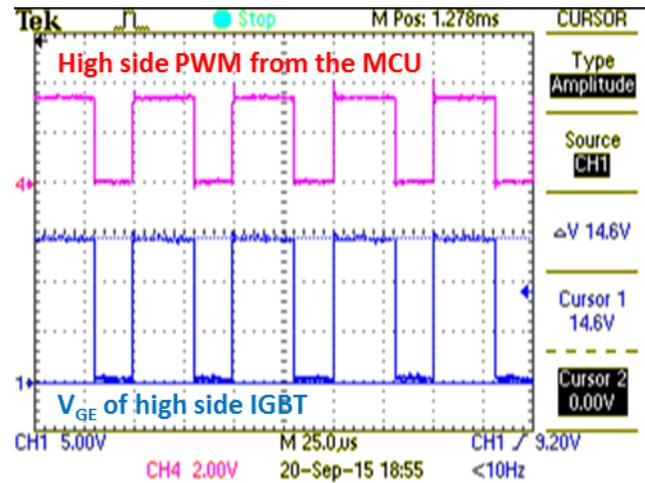
Figure 32.  $V_{GE}$  of High Side IGBT and PWM From MCU
