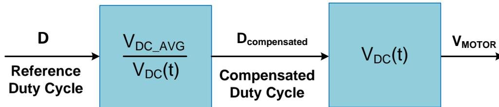
Figure 11. DC-Bus Voltage Ripple Compensation
