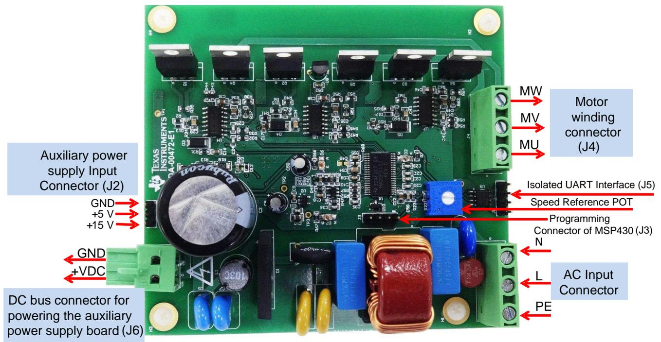
Figure 17. TIDA-00472 PCB Connectors
