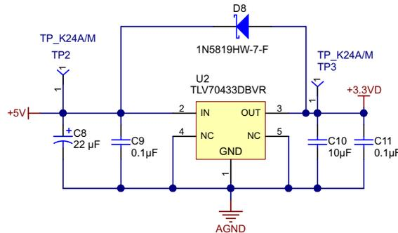
Figure 13. 3.3-V Power Supply Using LDO TLV70433
