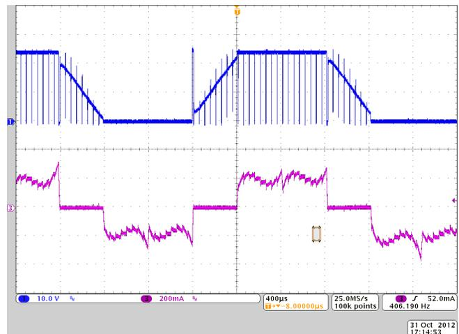
Figure 24. Typical Waveform for Optimum Flux Threshold
