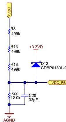
Figure 7. DC-Bus Voltage Sensing
