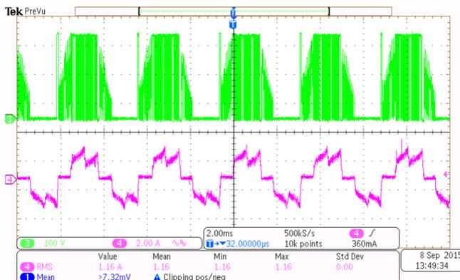
Figure 33. Winding Voltage and Winding Current of Motor at 250-W Inverter Power
