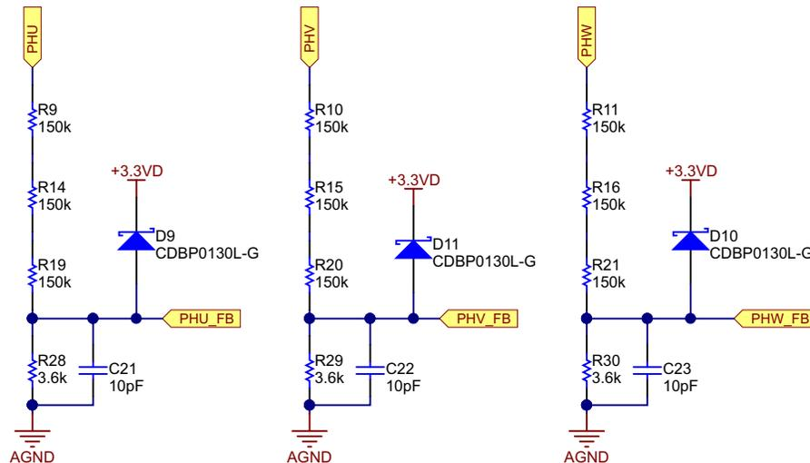
Figure 6. Motor-Winding Voltage Sensing
