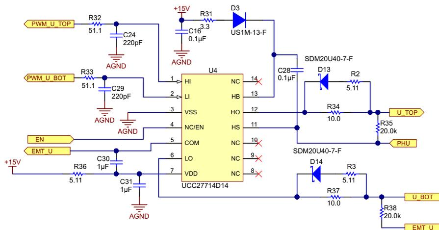
Figure 5. Gate Driver Circuit Using UCC27714
