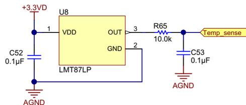
Figure 14. Heat Sink Temperature Sensor
