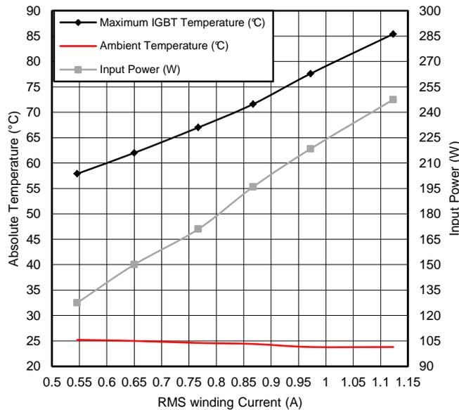
Figure 41. IGBT Temperature at Different Power Levels
