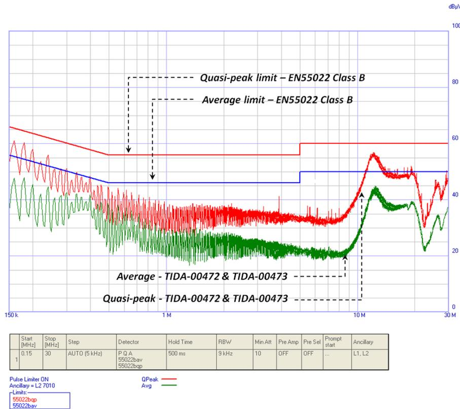
Figure 53. Conducted Emission Test Results as Per EN55022 Class B—Average and Quasi-Peak Detector Output
