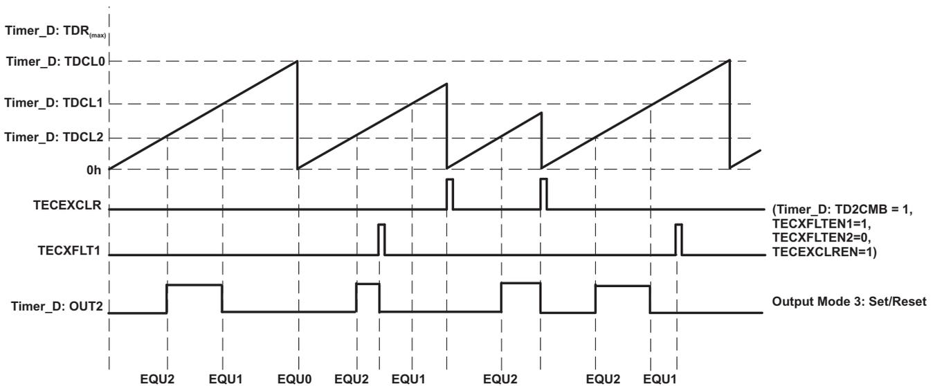
Figure 12. External Input Events Resetting Timer\_D Output
