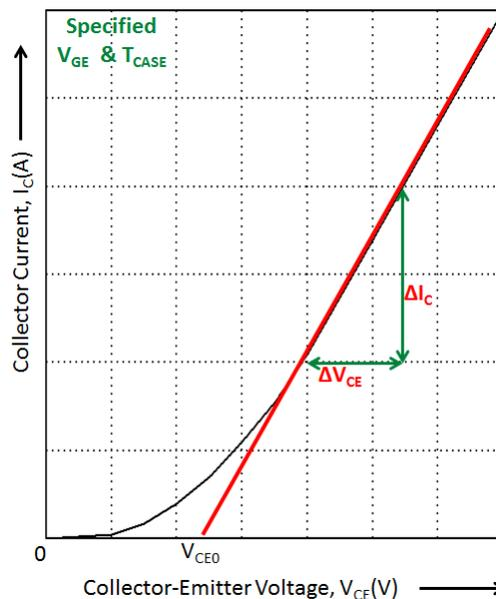
**Figure 4. Modeling of IGBT for Loss Calculation**
