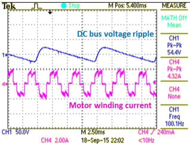
Figure 35. DC-Bus Voltage Ripple and Winding Current of Motor at 250-W Inverter Power
