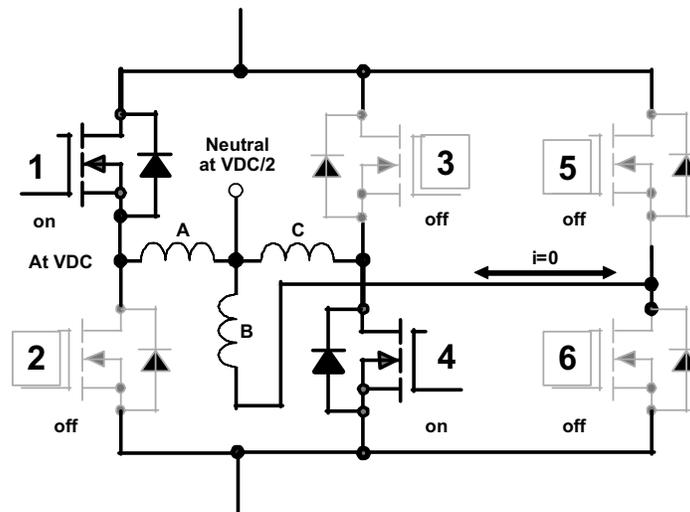
Figure 22. Motor Neutral voltage During PWM On-Period
