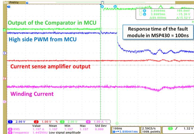
Figure 48. Response Time When Comparator Goes High to PWM Shutdown
