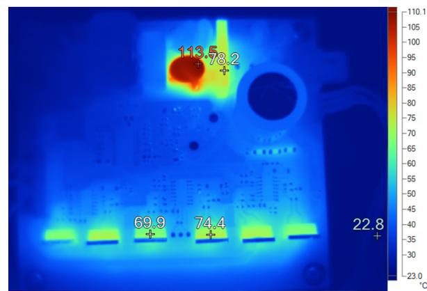
Figure 40. Thermal Image of Board at 200-W Inverter Power
