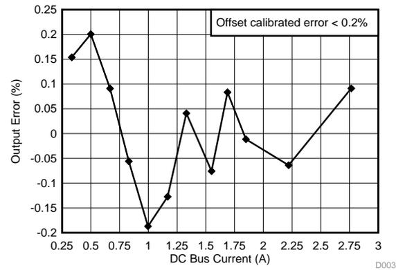
Figure 44. Offset Calibrated Output Error of Current Sense Amplifier
