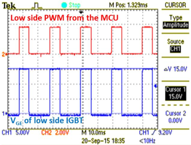
Figure 31.  $V_{GE}$  of Low Side IGBT and PWM From MCU
