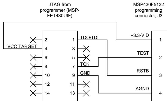
**Figure 19. Programming Interface Between the Programmer Kit and MSP430F5132**
