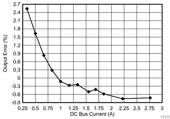
Figure 43. Uncalibrated Output Error of Current Sense Amplifier
