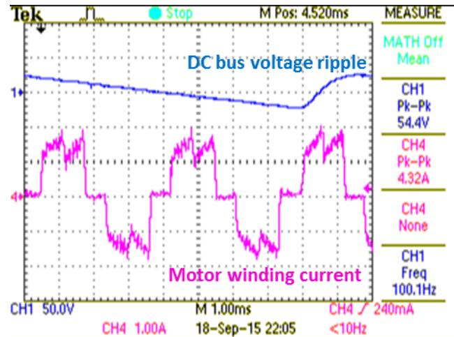
Figure 36. DC-Bus Voltage Ripple and Winding Current of Motor at 250-W Inverter Power (Zoomed-In to One Cycle of Voltage Ripple)
