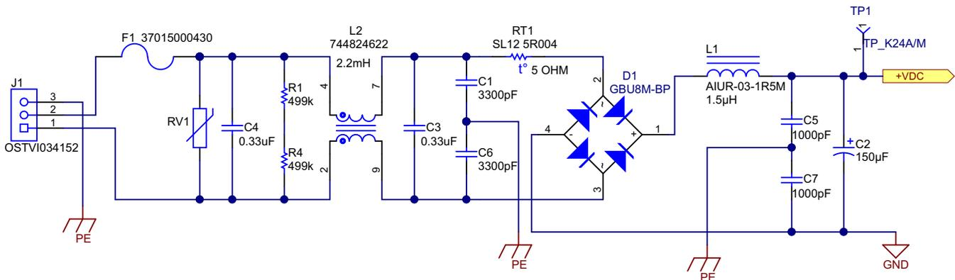
Figure 2. AC-DC Converter Schematic
