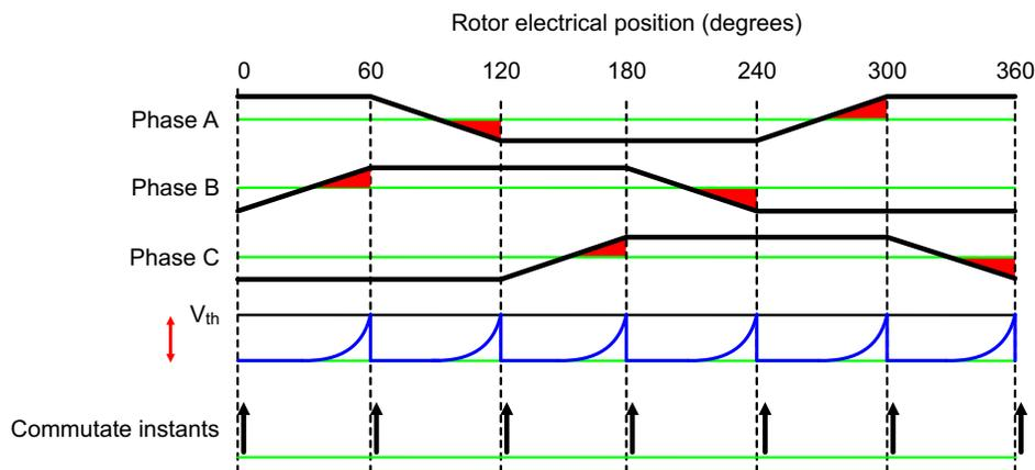
**Figure 21. InstaSPIN-BLDC—BEMF Integration Method to Determine Commutation Instant**
