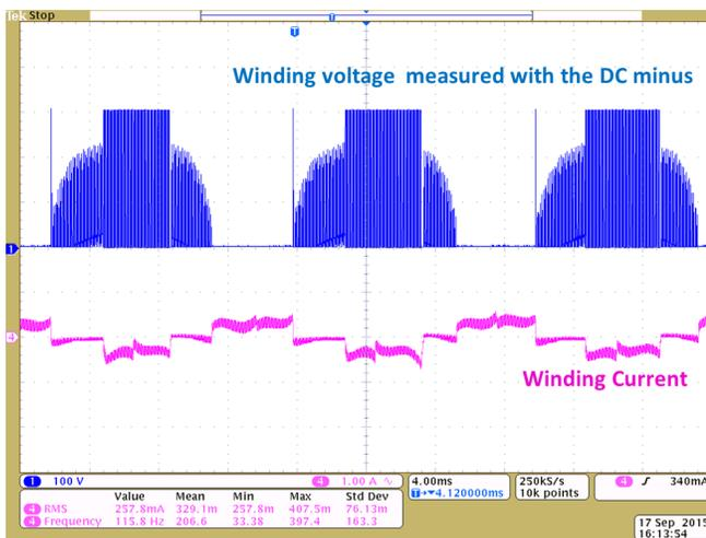
Figure 49. Winding Voltage and Winding Current of Motor at 1000 RPM
