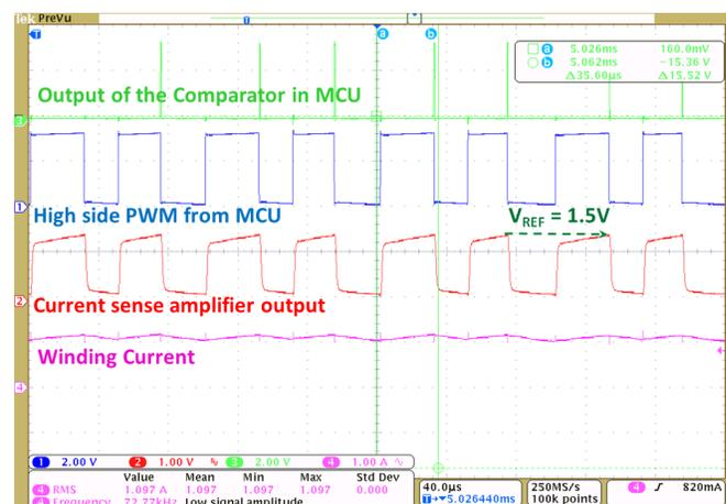
Figure 46. Cycle-By-Cycle Current Limit—PWM Shutdown With Comparator Output
