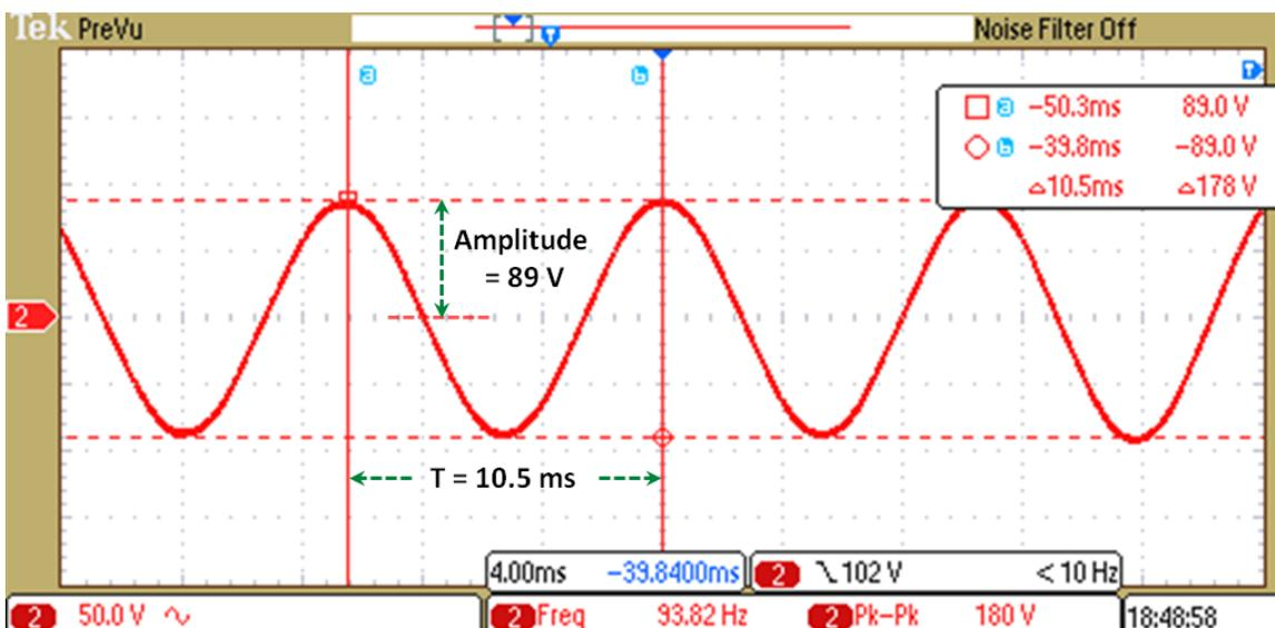
Figure 26. Example BEMF Waveform for Calculating  $K_e$
