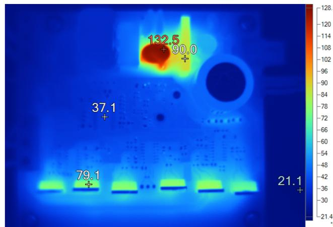
Figure 37. Thermal Image of Board at 250-W Inverter Power
