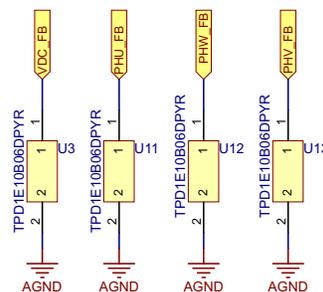
Figure 8. ESD Protection on Voltage Sensing Lines
