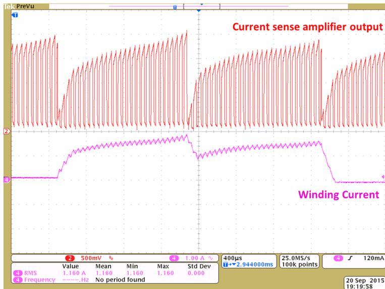
Figure 42. Motor Winding Current and Current Sense Amplifier Output
