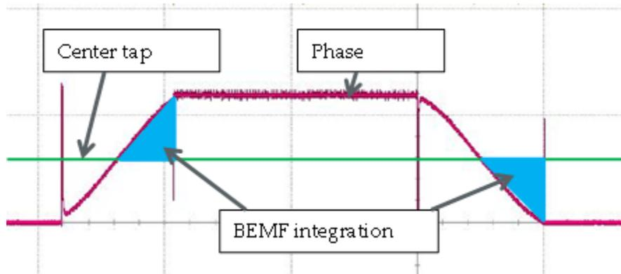
Figure 27. Phase Voltage Waveform Showing BEMF Integration Zone
