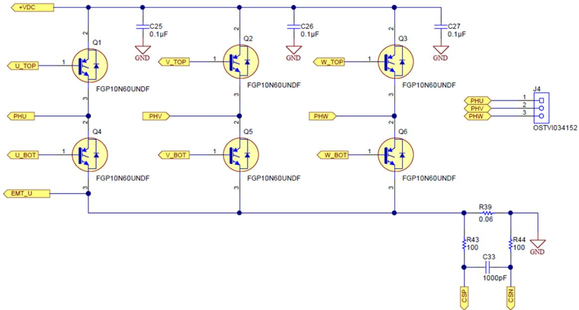
Figure 3. Three-Phase Inverter of Power Stage
