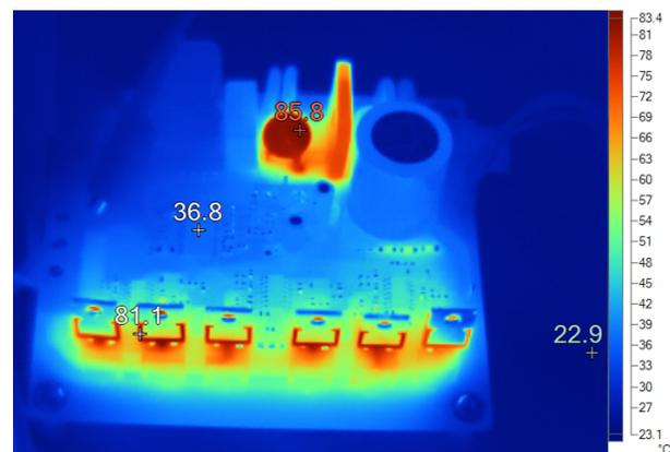
Figure 34. Thermal Image of Board at 250-W Inverter Power and 300-V DC Input
