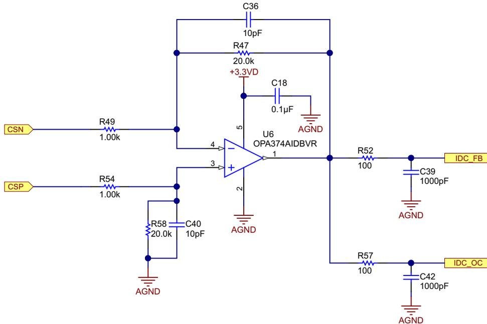
Figure 9. Current Sense Amplifier Using OPA374
