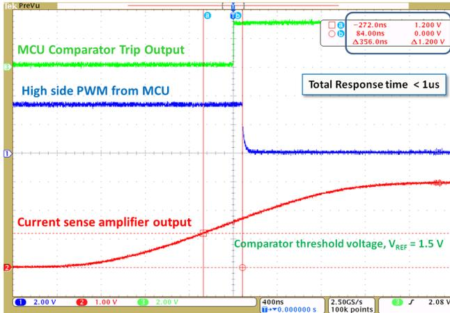
Figure 47. Total Response Time of Cycle-By-Cycle Current Limit Protection
