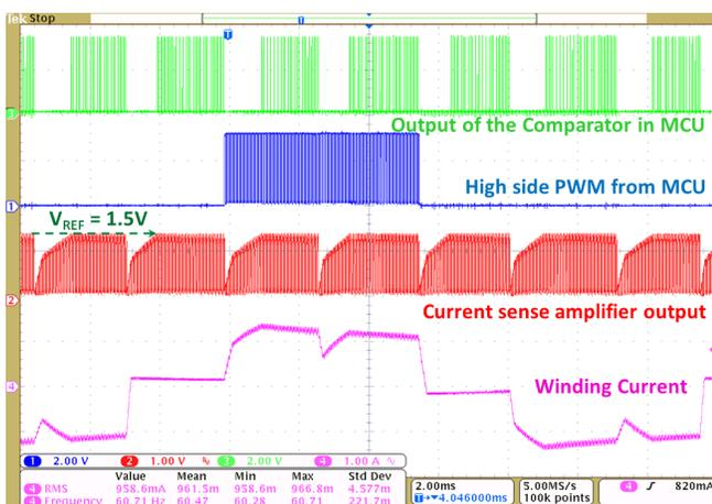
Figure 45. Cycle-By-Cycle Current Limit Using Hardware Features of MSP430F5132
