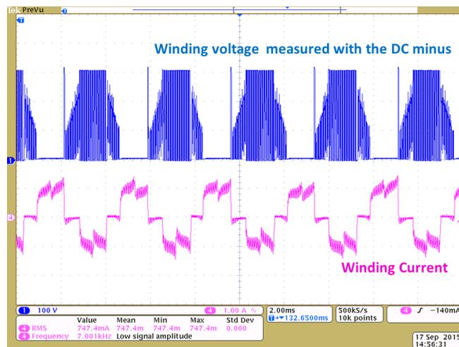
Figure 50. Winding Voltage and Winding Current of Motor at 4000 RPM
