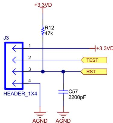
**Figure 18. Four-Pin Programming Connector Provided in TIDA-00472 Board**
