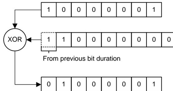
**Figure 14. Calculation of Edges in a Bit Period**
