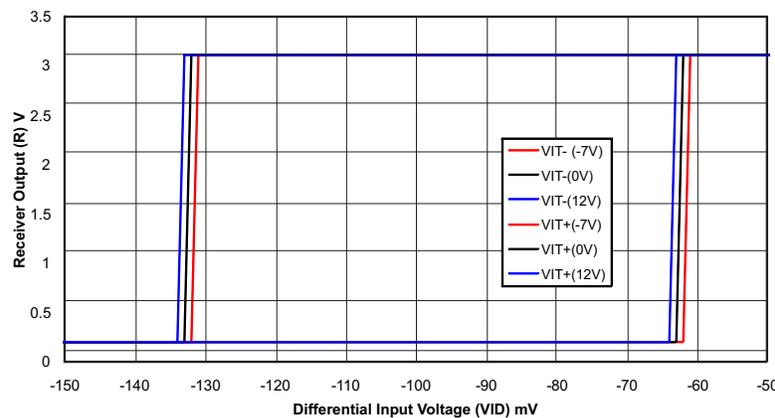
**Figure 12. Input Voltage Hysteresis of SN65HVD78 Transceiver**
