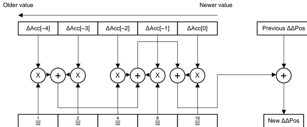
**Figure 16. Estimation Algorithm for  $\Delta\Delta$ Position**
