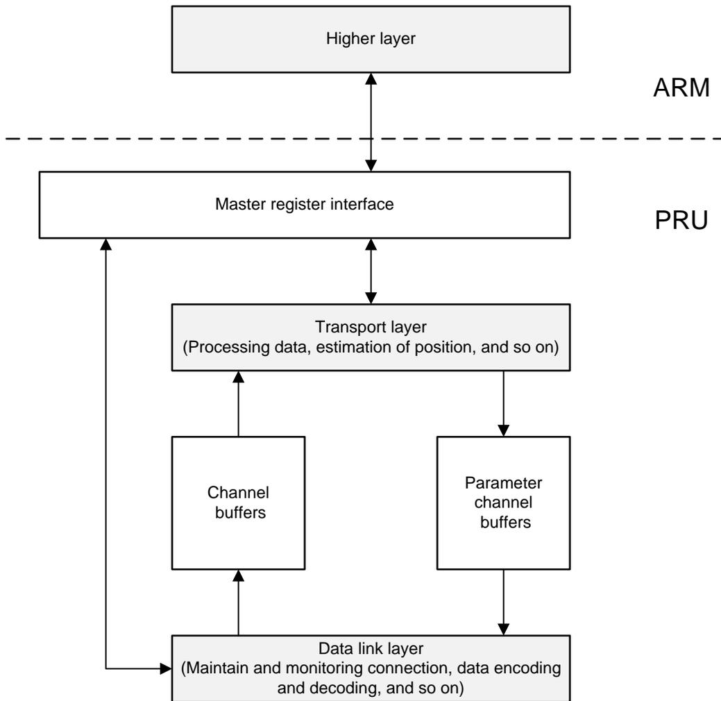
**Figure 9. Firmware Architecture**
