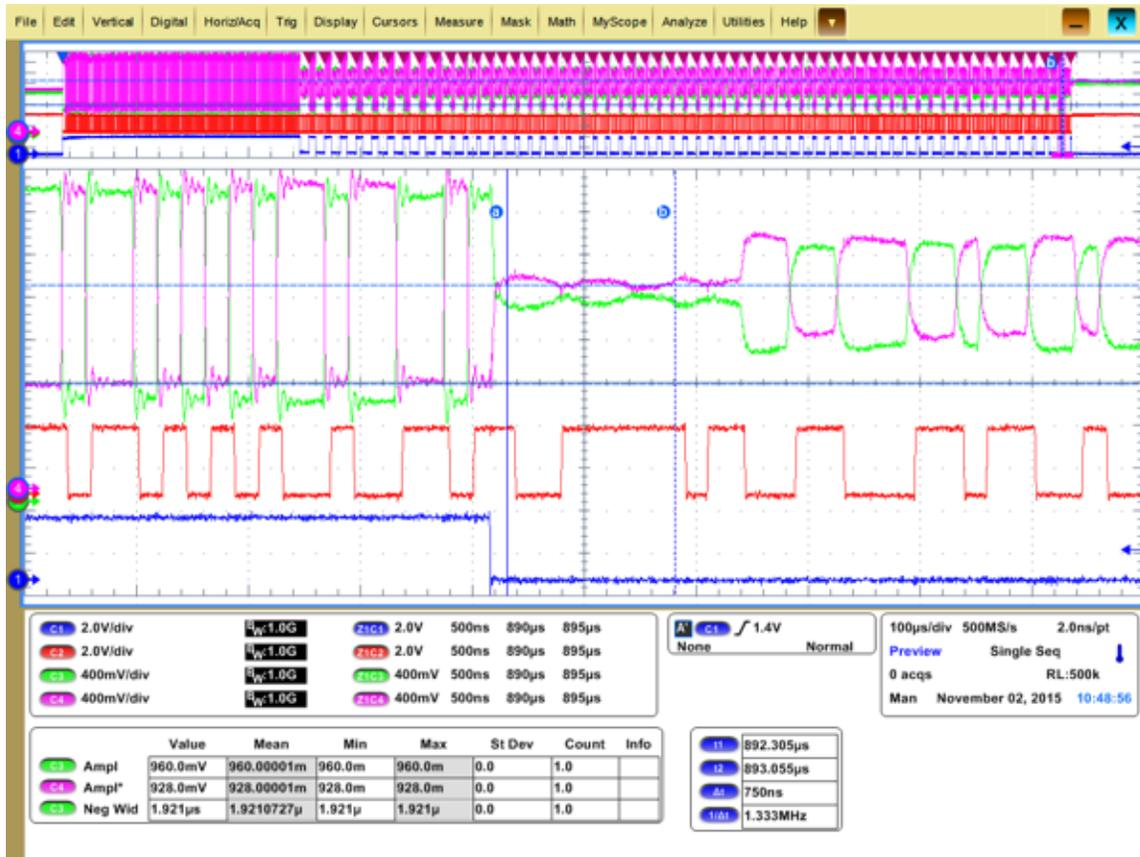
Figure 13. Failing Condition With Unbalanced DC Line
