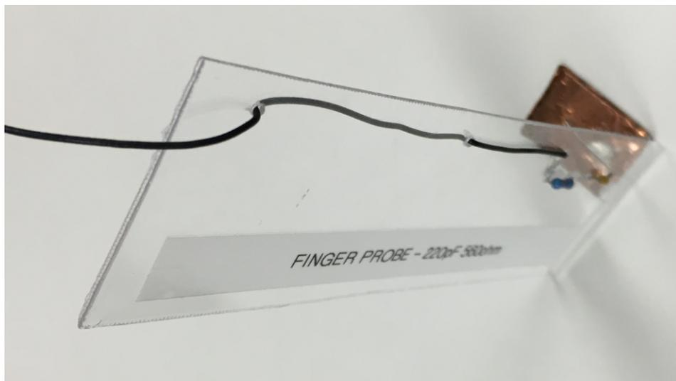
Figure 55. Artificial Finger Probe
