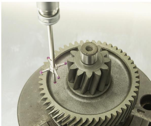
*Figure 1. Example of a coordinate measurement machine probe*
