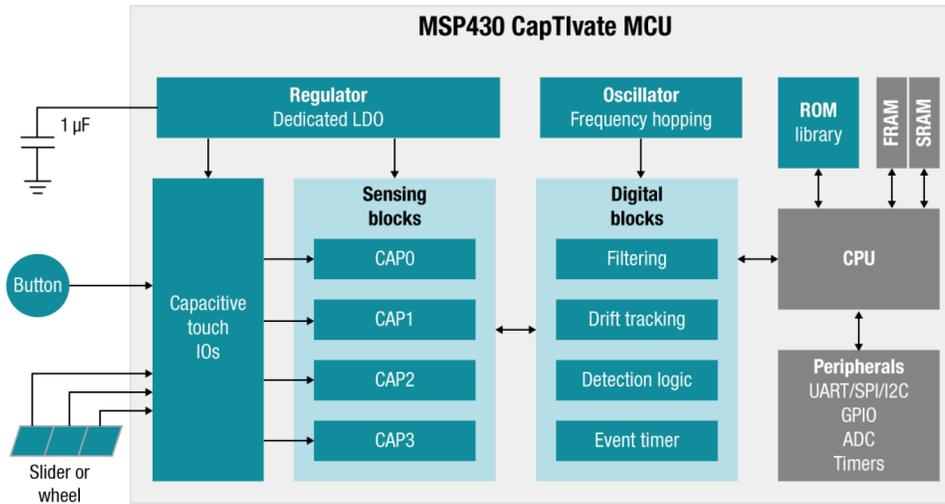
**Figure 2-1. MSP430 Capacitive Sensing MCU Block Diagram**
