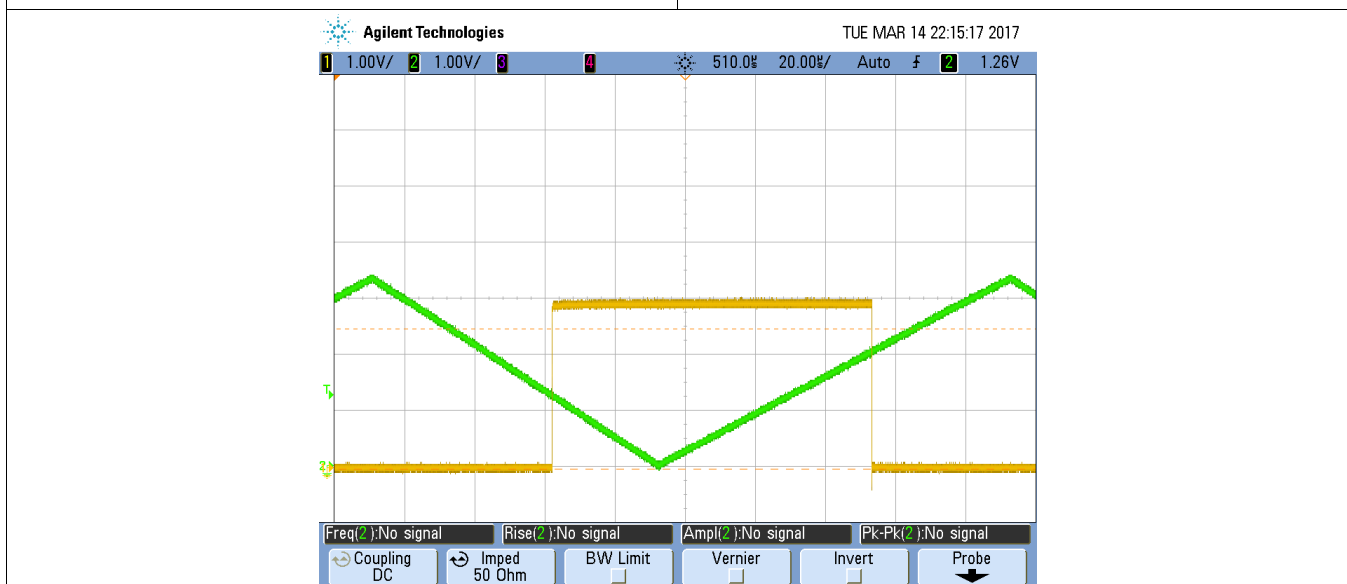
Figure 16. Lab Setup Comparison With Schmitt Trigger SN74LVC1G14
