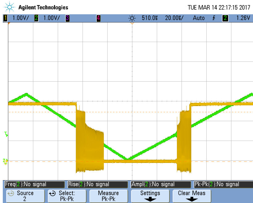
Figure 12. Waveforms Without Schmitt Trigger- SN74LVC1G34
