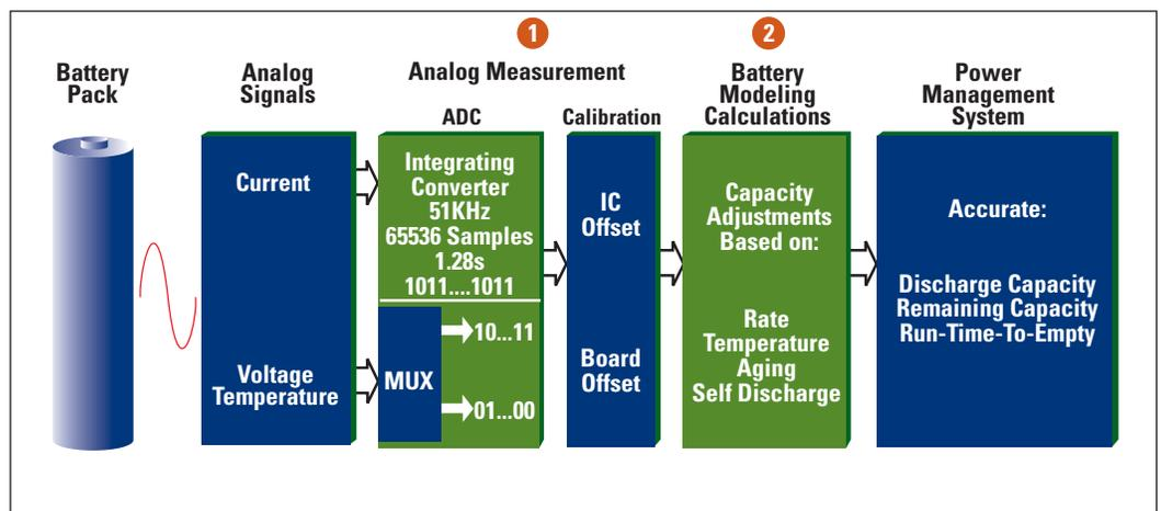
**Figure 3.** The two components of battery fuel gauge accuracy: analog measurement and battery modeling
