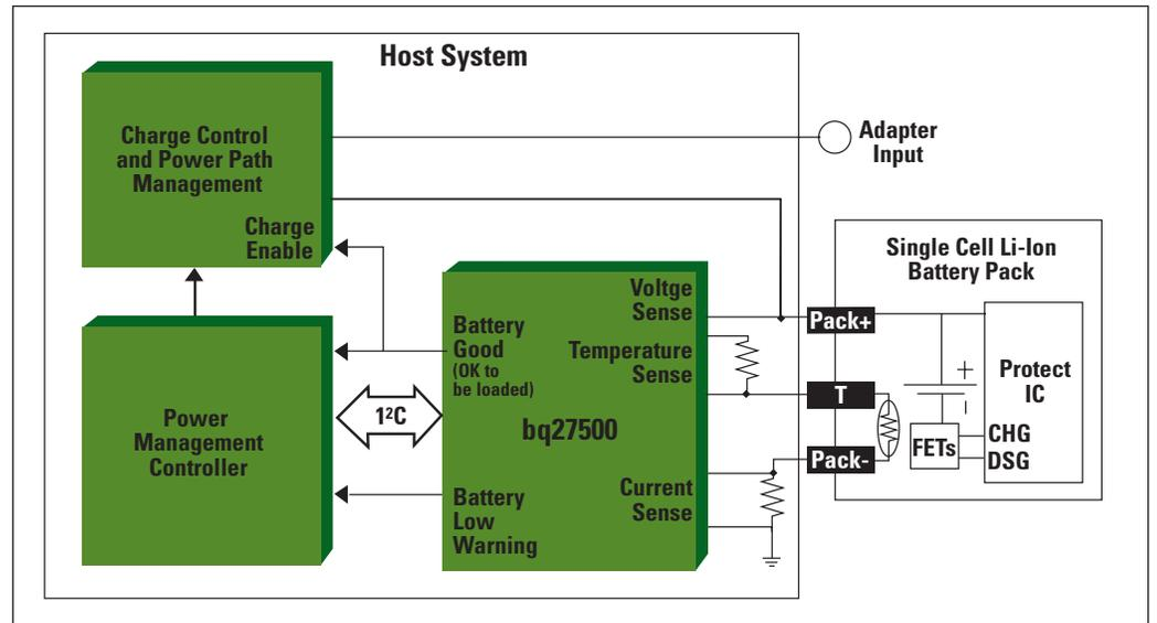
**Figure 5.** Impedance Track enables a new battery management architecture: Host-side (system-side) battery fuel gauging with the bq27500
