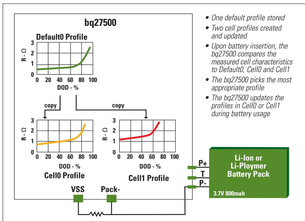
**Figure 6.** bq27500 "arbitration" method for an inserted battery pack
