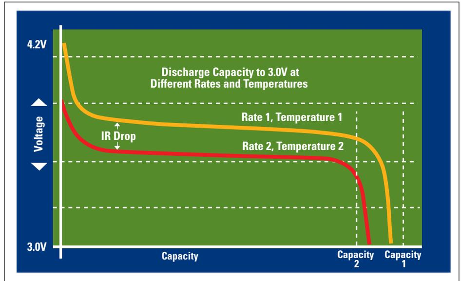
**Figure 4a.** Rate and temperature dependency on battery discharge capacity
