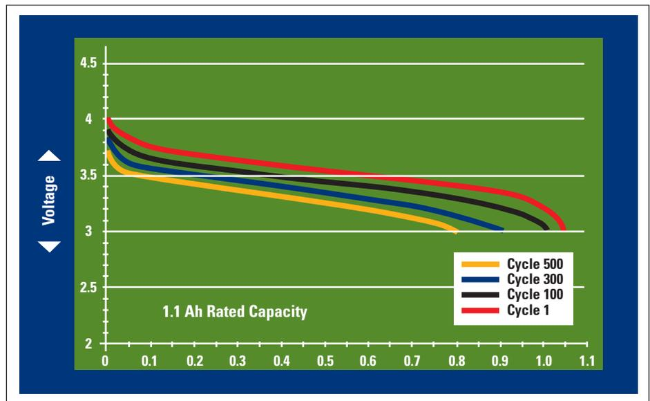
**Figure 4b.** The effect of battery aging (increase in impedance) because of usage on battery discharge capacity
