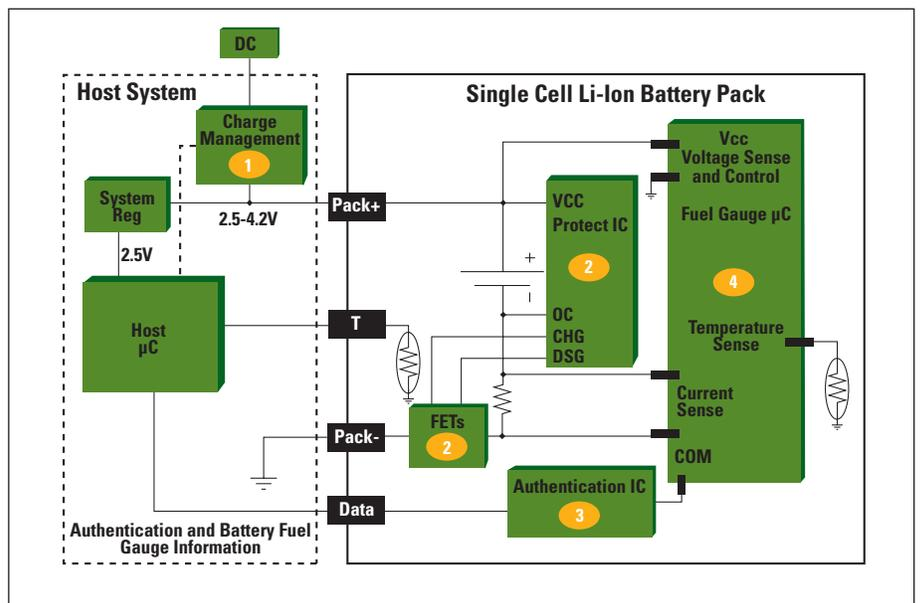
**Figure 1.** The four basic functions of battery management: 1. Charge control, 2. Li-Ion protection, 3. Battery pack authentication and 4. Battery fuel gauging
