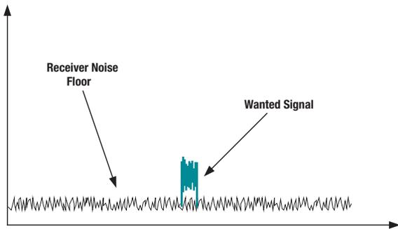
Figure 3. Small wanted signal in sensitivity case
