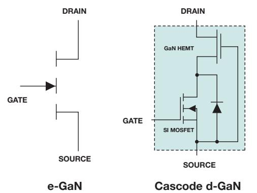
**Figure 1.** Symbols of e-GaN and cascode d-GaN devices highlight structural difference.
