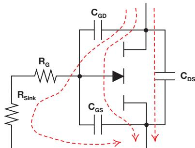
**Figure 3.** Parasitic capacitances and currents in a GaN power device.
