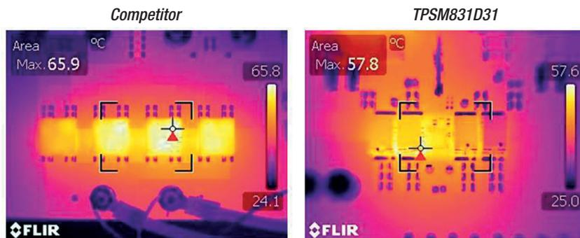
Figure 3. Thermal performance comparison:  $V_{IN} = 12\text{ V}$ ,  $V_{OUT} = 1.0\text{ V}$ ,  $I_{OUT} = 100\text{ A}$ ,  $F_{sw} = 500\text{ kHz}$ ,  $22^\circ\text{C}$  ambient,  $200\text{ linear ft./min.}$  airflow.
