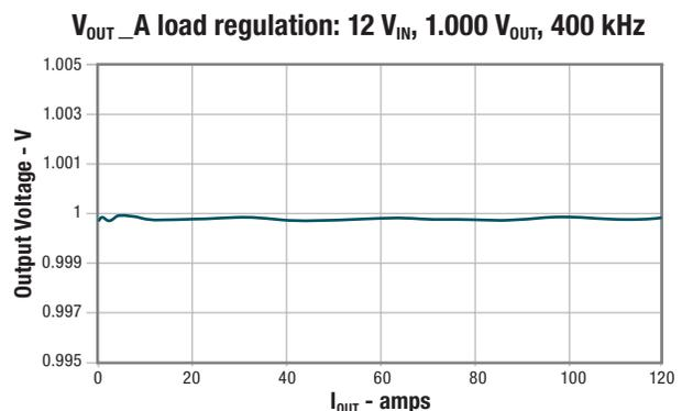
**Figure 11.** TPSM831D31 DC load regulation up to 120 A.
