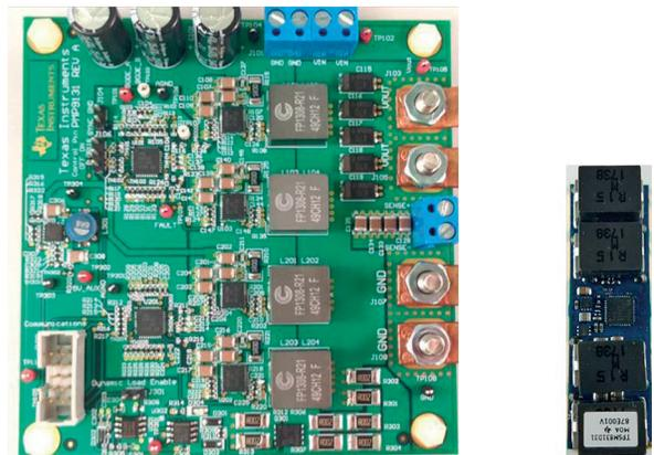
Figure 14. Discrete regulator vs. the TPSM831D31 (four total phases in each design).
