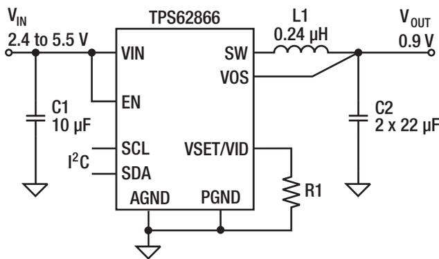
**Figure 7.** The TPS62866 contains both an I<sup>2</sup>C bus and a VID pin to adjust the output voltage after startup.
