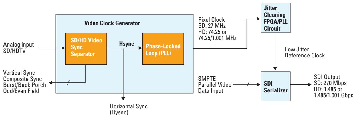
Figure 1. SDI Reference Clock Generator Block Diagram
