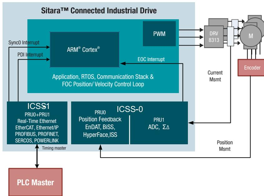
Figure 7: Connected industrial drive processor
