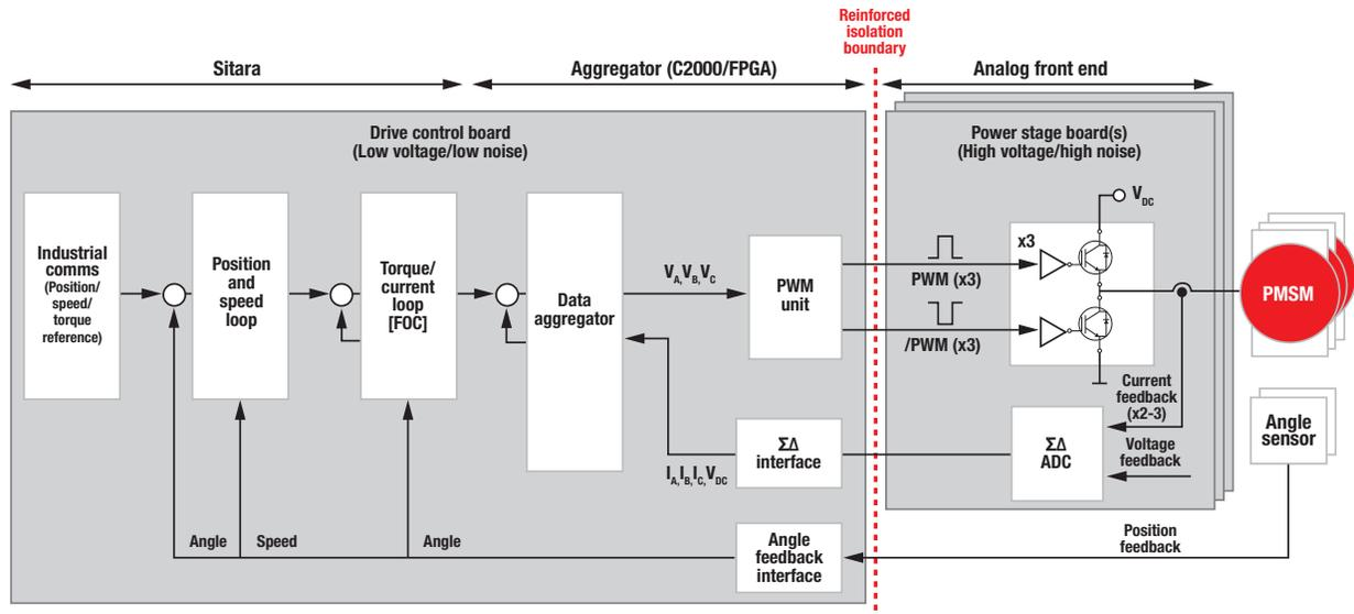
**Figure 3** Example of using a Sitara processor as a servo processor with control function offloaded to a C2000™ microcontroller or an FPGA on the cold side of the system.
