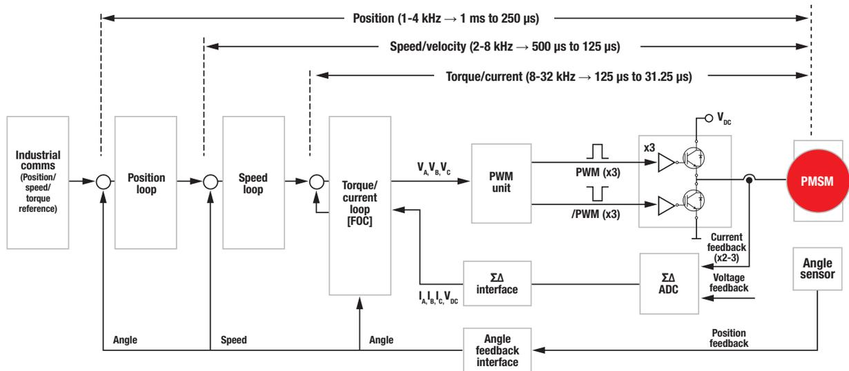
**Figure 1** Typical servo motor control loop topology.
