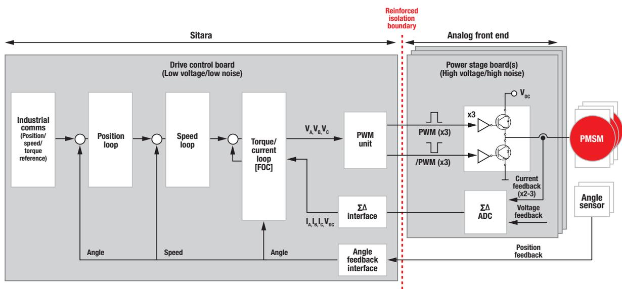
**Figure 4** Example of using a Sitara processor to implement full servo control on the cold side.
