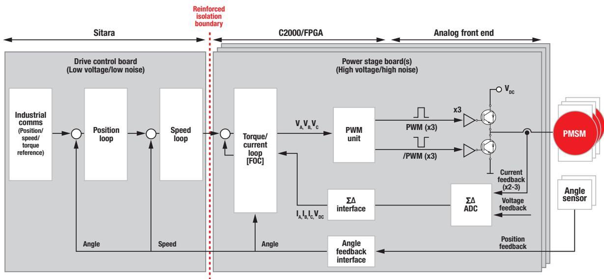
**Figure 2** Example of using a Sitara processor to communicate across the isolation boundary to a separate control unit on the hot side of the system.
