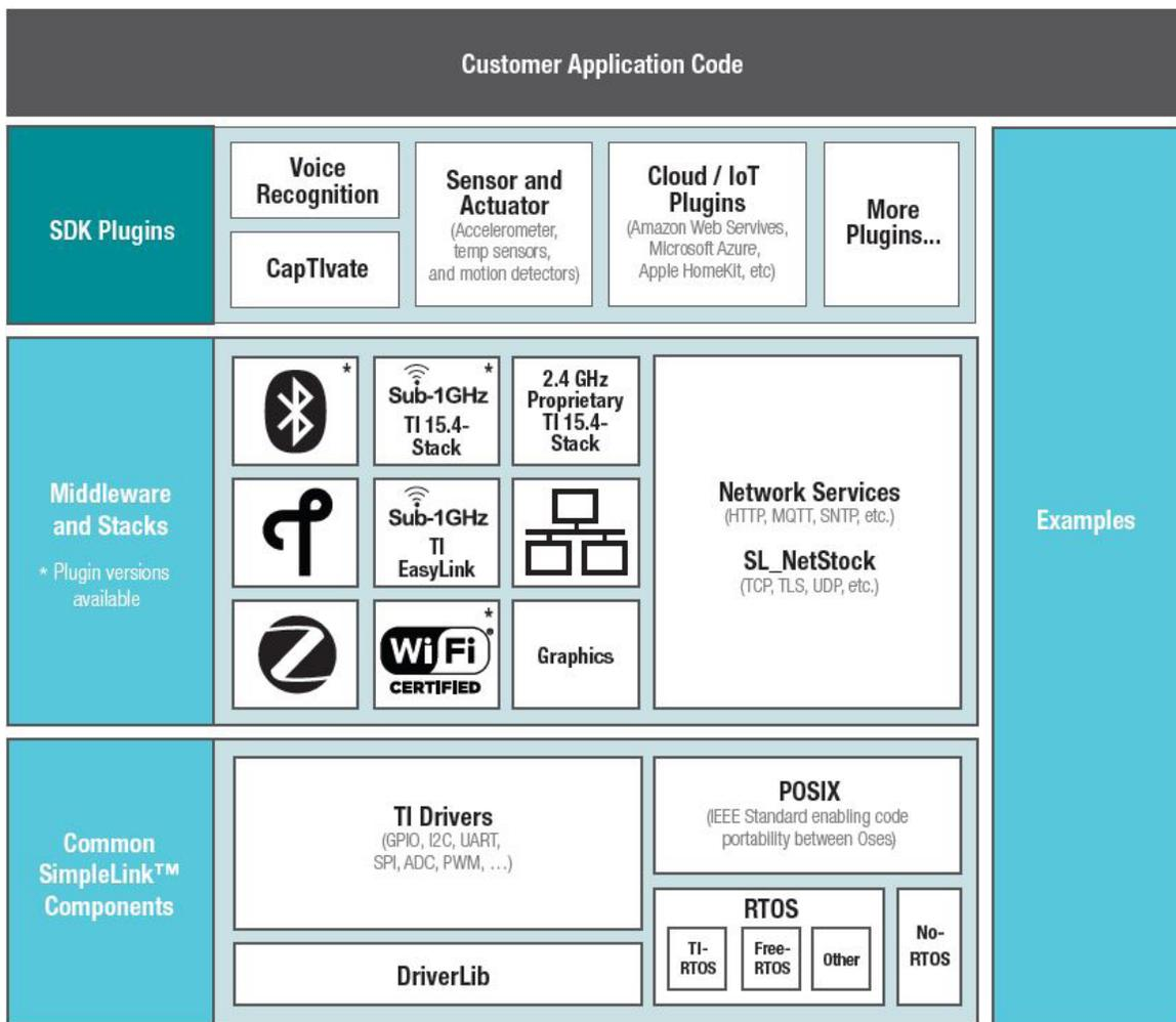
Figure 3. SimpleLink SDK diagram.
