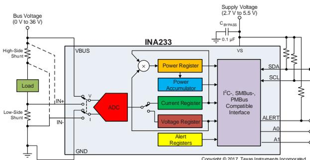
Figure 1. INA233 Typical Application Circuit
