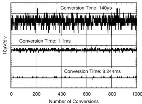
**Figure 3. Noise vs. ADC Conversion Time**
