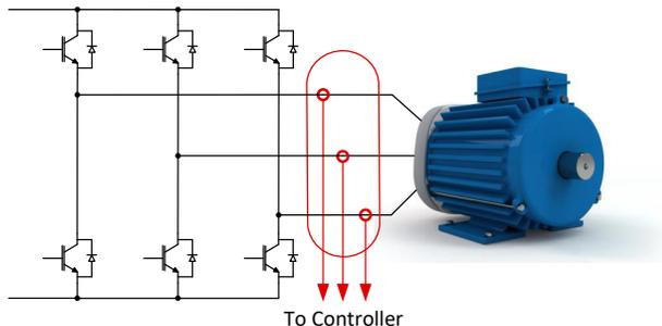
**Figure 1. In-Line Current Sensing**
