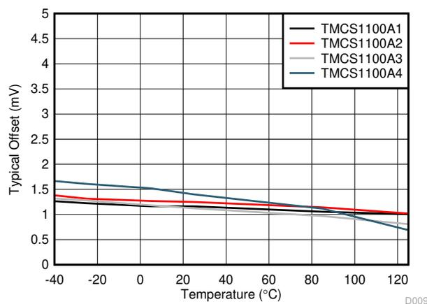
**Figure 4. TMCS1100 Typical Output Offset Across Temperature**
