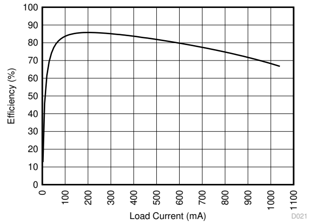
Figure 6-24. Efficiency vs Load Current
