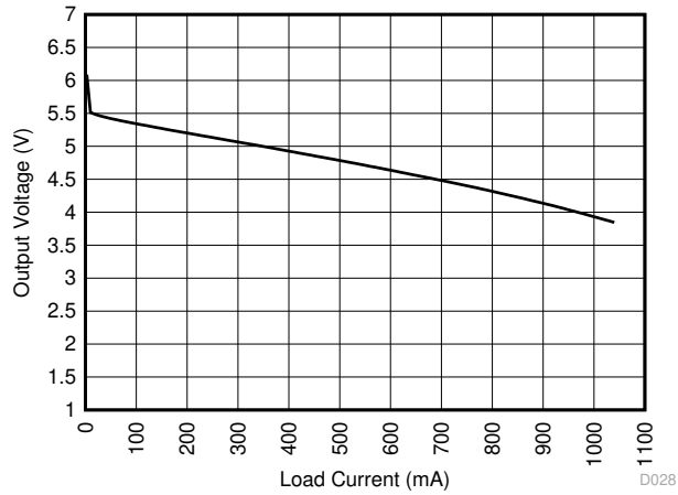
Figure 6-3. Output Voltage vs Load Current
